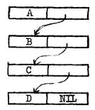
Because of this use of pointers, a list may be a member of many other lists, each of which has a pointer to it. When a new list is generated by cons, a single memory word is used. In it are placed pointers to the two elements of the dotted pair being created by the cons. No account is taken of other lists of which either element may be a member.
