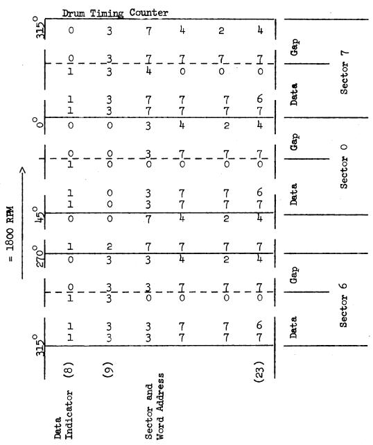
Information is written on 84 bands around the drum. Each band is divided into 8 sectors. Each sector contains 2,048 words of storage and 236 words of gap (non-addressable memory). Bits 9 through 23 of the drum timing counter contain the word address of the location. Bit 8 indicates data or gap field.
