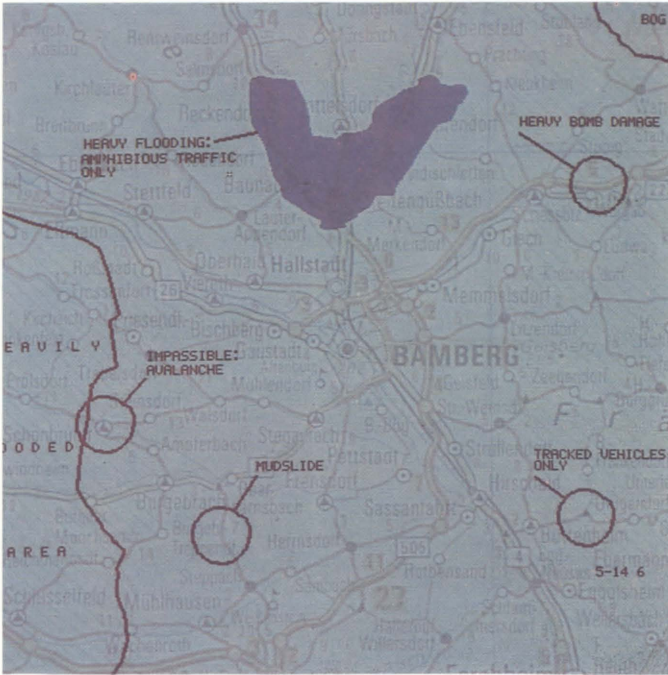
Trafficability Perspective The Trafficability Perspective reflects potential for moving forces on a broad scale. It is not confined to normal transportation routes and it includes terrain and soil characteristics for large areas and nuclear, biological, and chemical (NBC) contaminated areas.
