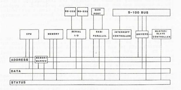
Figure 2-1. BLOCK DIAGRAM
