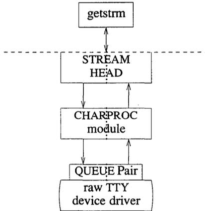
**Figure 4-1** Idle Stream Configuration for Example
