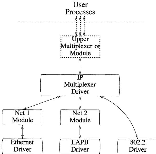
**Figure 6-3** Internet Multiplexing Stream
