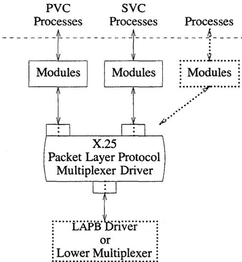
Figure 6-4 X.25 Multiplexing Stream
