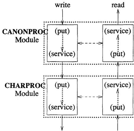
Figure 5-4 Module Put and Service Procedures
