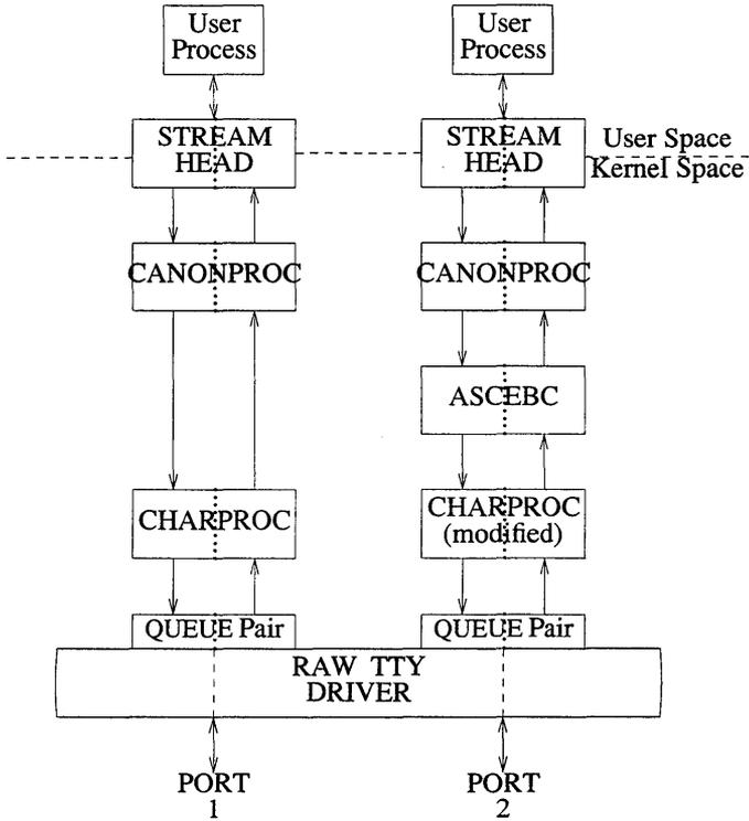
Figure 4-2 Asynchronous Terminal Streams
