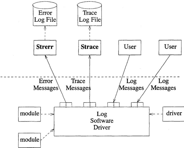
Figure 6-5 Error and Trace Logging
