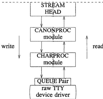
**Figure 5-3** Operational Stream for Example
