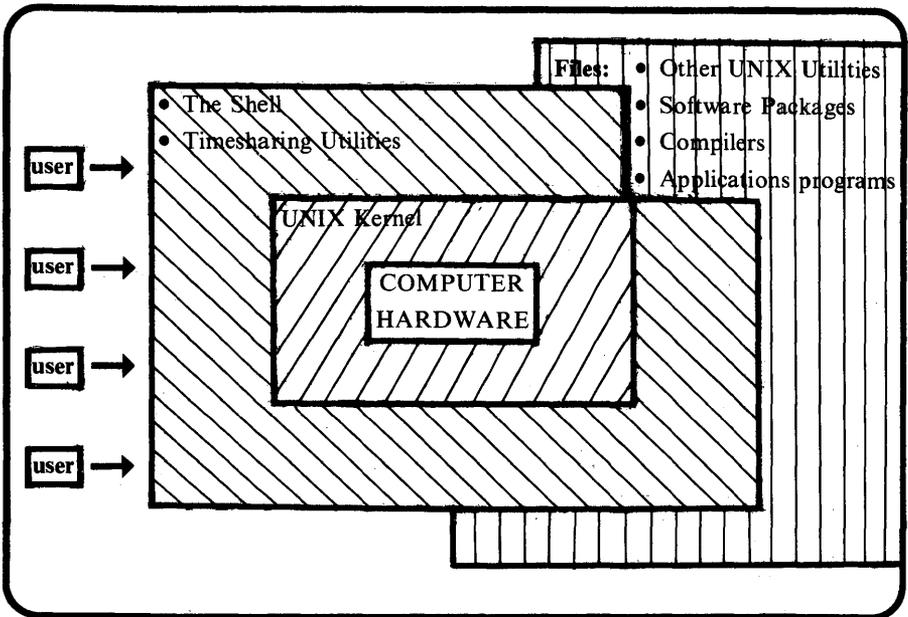
**Figure 1.1.** General structure of the UNIX operating system.
