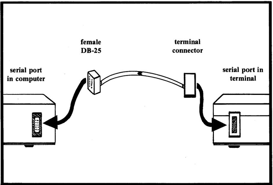
**Figure 3.1.** Diagram of connection between an IBM PC XT computer and a terminal.
