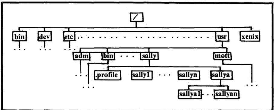
Figure 9.1. Simplified illustration of the XENIX file system.
