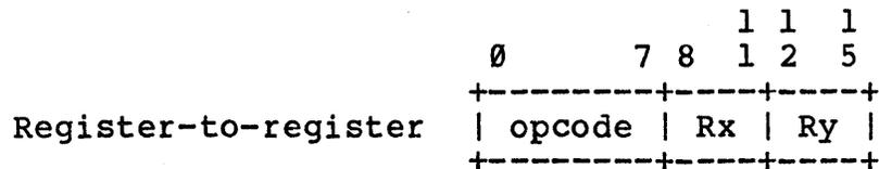
A few register-to-register format instructions also have an immediate mode. In immediate mode the 4-bit value of the Ry register field is used to specify an integer in the range from 0 to 15.
