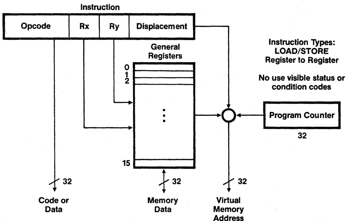
Figure 2 Model of Processor Architecture
