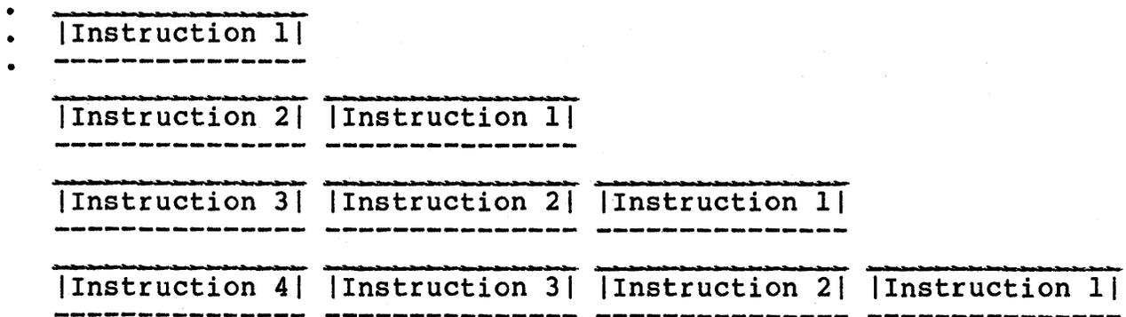
Figure 3. Processor Instruction Pipeline
