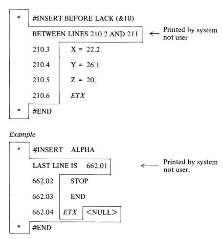
Syntax Checking and Statement Reformatting • When a program is initially being entered at the terminal, it is normally checked for executability by the interactive system. This check is carried out by also building a symbol table and checking for consistency in the use of names. In order to change this normal mode, the following control options are allowed on the #INSERT statement:
