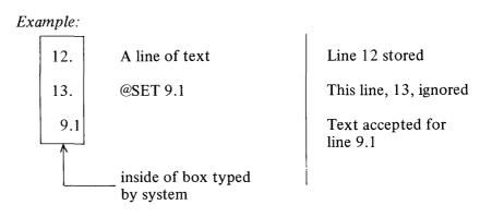
This command is valid only if an insert is being made to a file and if a line number has been typed out by the system.
