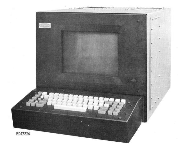
Figure 1-1. Model 402-2AM13 Display Terminal
