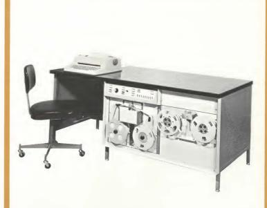
The Tape Preparation Unit is an off-line preparation desk equipped with a typewriter, a paper-tape punch with supply and take-up reels, and a paper-tape reader with bi-directional tape reading capability.
