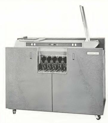
The Card Read-Punch is a device which can read standard 80-column cards at 800 cards per minute and punch cards at 250 per minute. Card reading and punching are by row with independent reading and punching achieved through the use of an opposing feed design. The Card Read-Punch unit has easy access to all operating mechanisms and the
