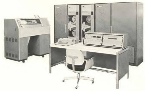
The Raytheon 520 System provides the most powerful and useful input/output capability available in machines of its class. Input, output, and computing can occur simultaneously. Maximum input-output character rate is four million characters per second; word rate is 1MC.
