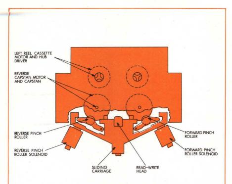
Simple cassette drive design. Four motors, though more complex by some yardsticks than one or two motors, are still more reliable than the mechanical linkages needed when the one or two motors must be connected to both reel shafts and both capstans in a bidirectional tape cassette drive. Head penetration into the cassette, controlled by the sliding carriage, is less than in some other machines, extending head life and improving tape guidance
