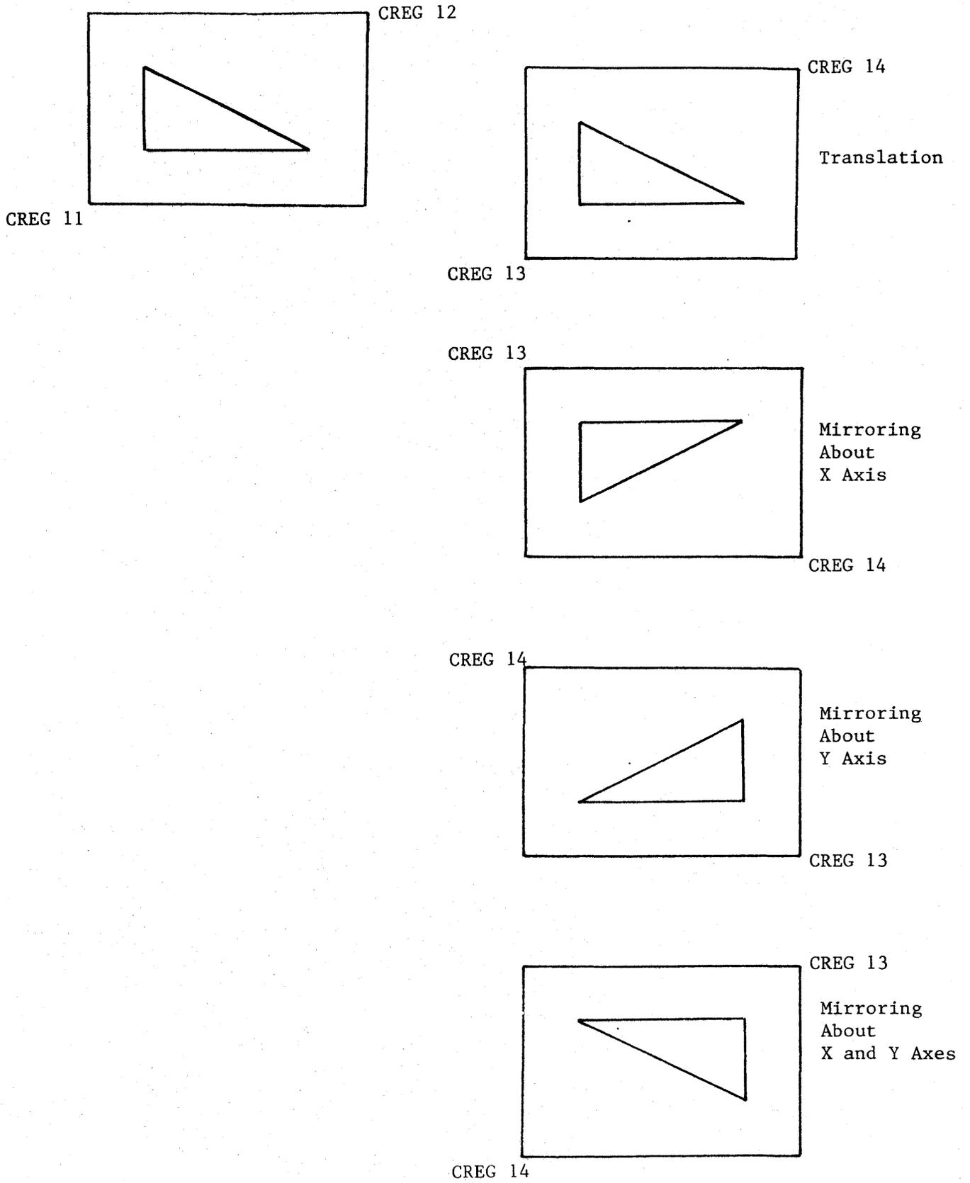
Figure 8.1 Settings of CREGS 11 Through 14 Allow Mirroring
