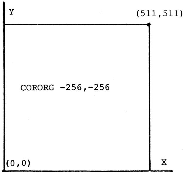
Figure 3.2 Resetting the Coordinate Origin
