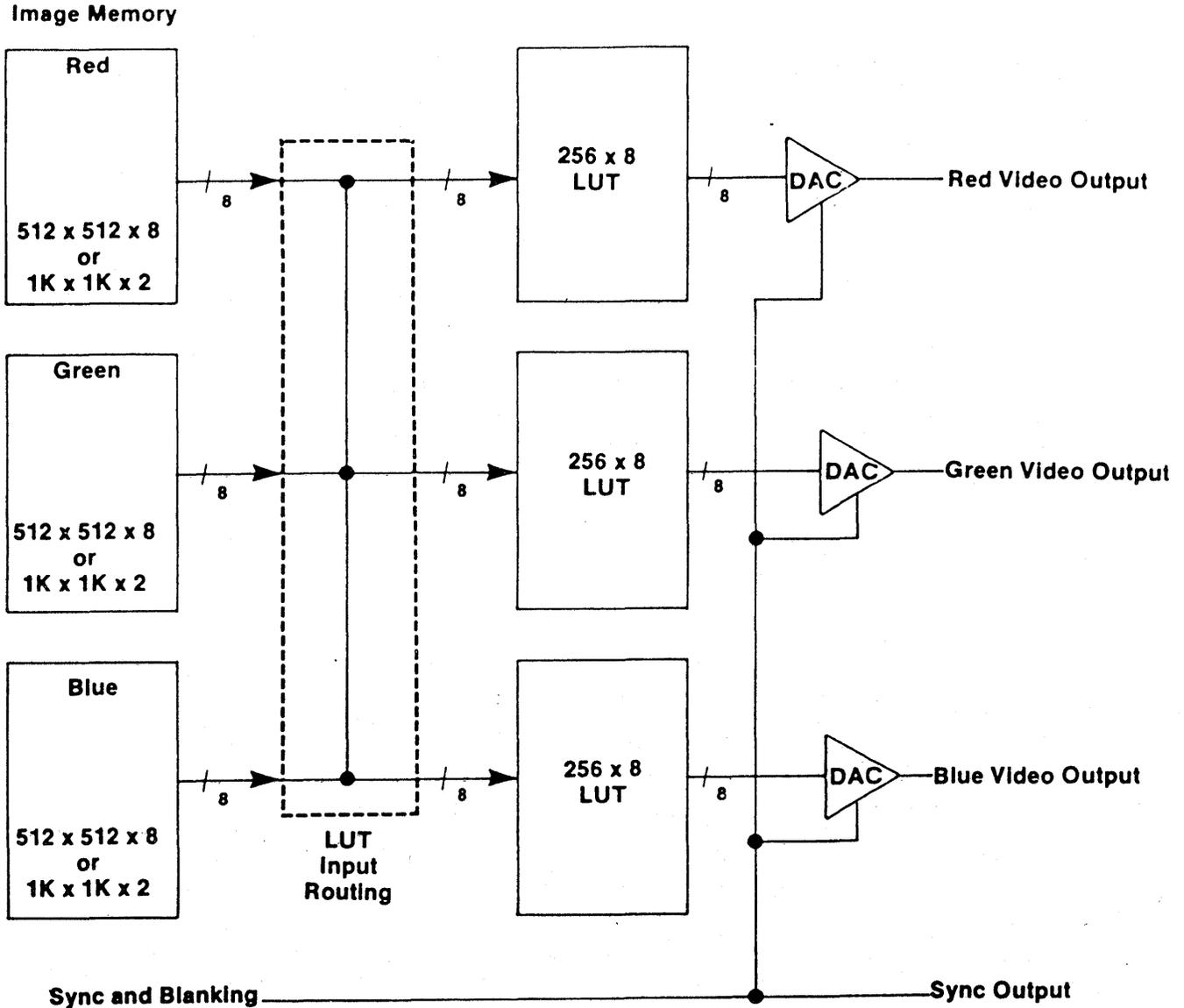
Figure 4.1 The Interrelationship of the Image Memory, Look-Up-Tables, and Digital-to-Analog Converters
