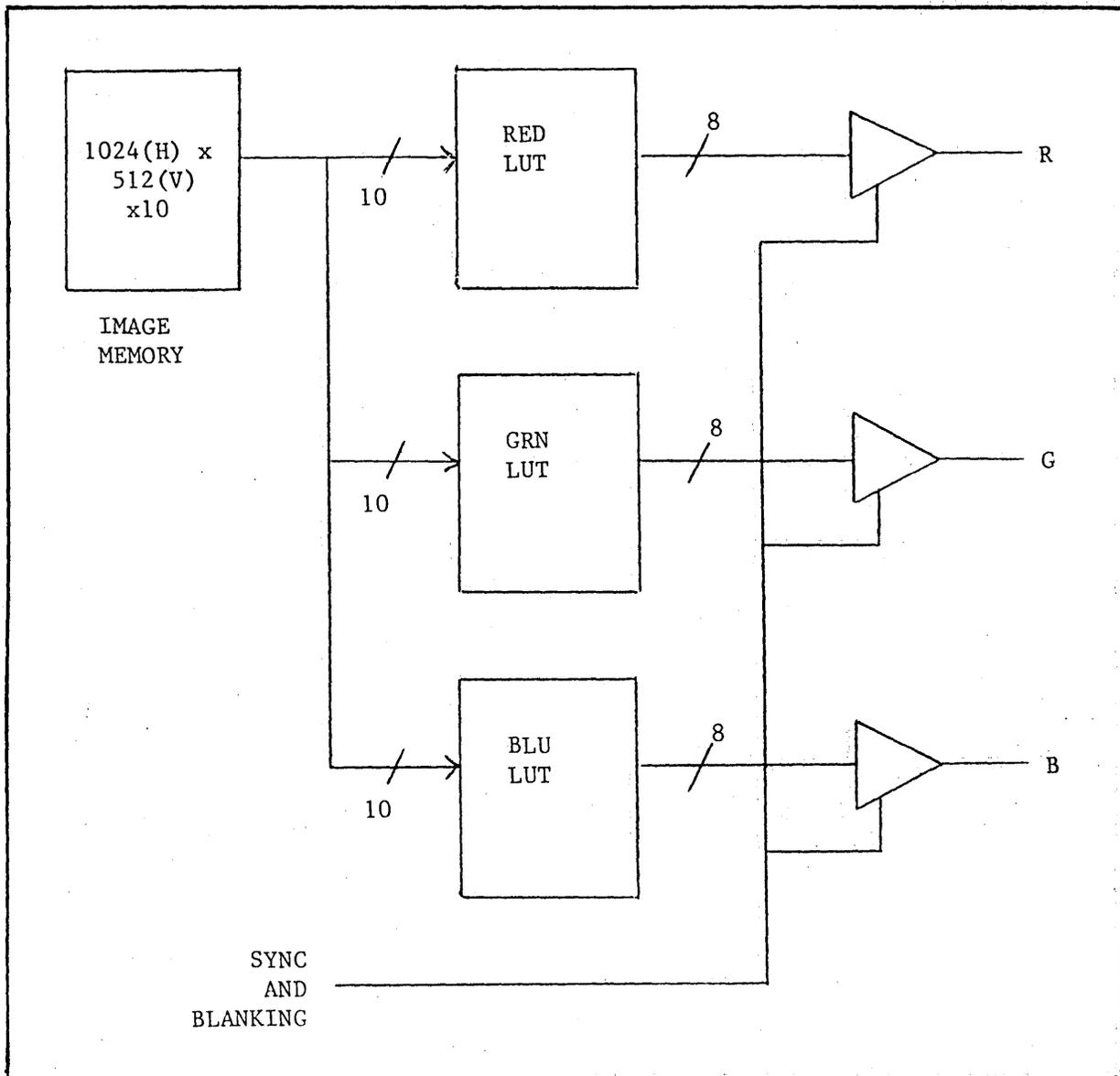
Figure 8.1 Image Memory Output Diagram
