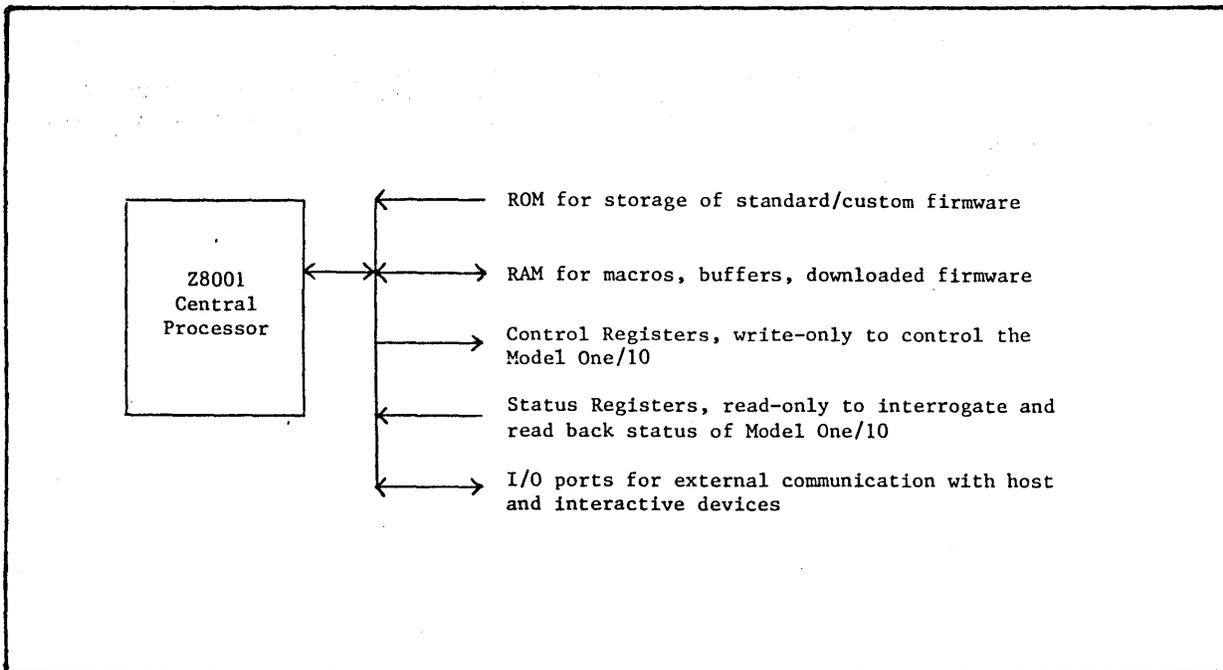
Figure 6.1 Central Processor Addressing and I/O
