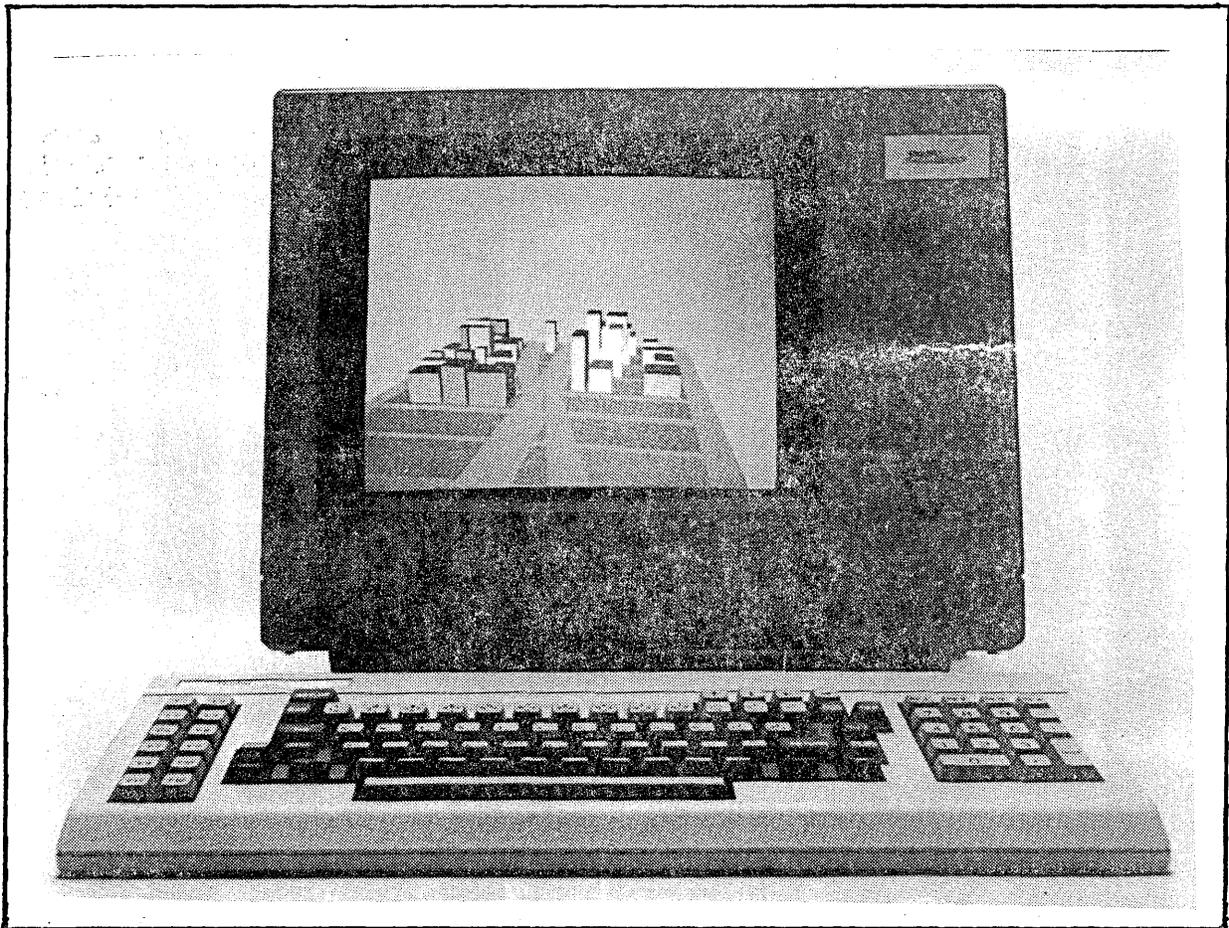
Figure 2.1 Model One/10 Integrated Graphics Terminal
