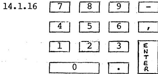
The keypad is arranged in adding-machine style, for applications requiring a great deal of numeric input. With Alternate Keypad mode off, pressing numeric key transmits the same numeric code as the corresponding key in the main keyboard section. The ENTER key functions as the RETURN key does on the main keyboard. However, with Alternate Keypad mode enabled, keypad keys are programmed to send escape sequences (see Table 14.3).
