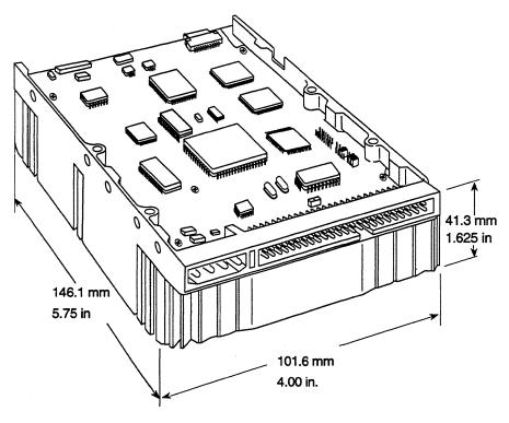
Figure 3-1 Mechanical Dimensions
