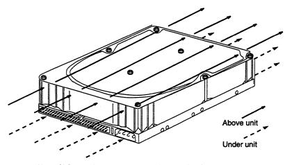
Note: Airflow in the direction shown (back to front) or in reverse direction (front to back)
