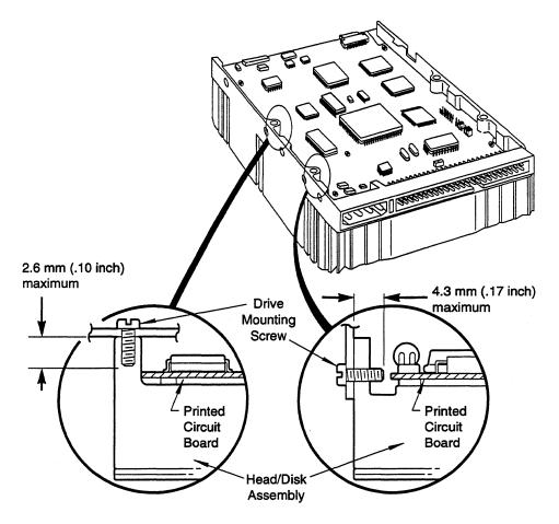
Figure 3-5 Mounting Screw Clearance
