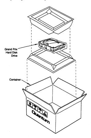
Figure 3-2 Packing Assembly
