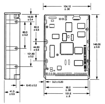
Figure 3-4 Mounting Dimensions (in millimeters)
