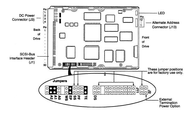
Figure 3-3 Jumper Pin and Terminator Locations on the Drive PCBA
