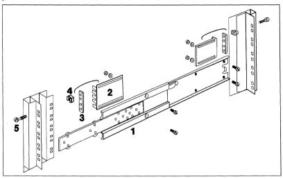
[1] Telescopic Slides[2] Mounting Bracket[3] Threaded Strip[4] M6 Cage nut[5] Collar screw
