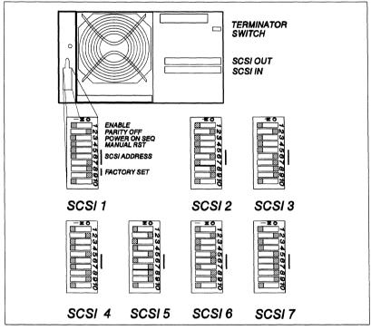
When the drive is at the end of the bus, and using the black SCSI cable, the switch 2 on the rear panel of the drive should be set to the "T" position and the metal SCSI terminator should be fitted to the upper SCSI connector.
