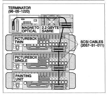
This example shows how a Picturebox Single, Picturebox Twin, a Harriet, a 2.2 Gbyte Sabre drive and a Magneto Optical drive are connected together to form a Shared user bus.
