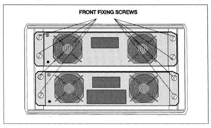
When the tower and unit are secured, the unit's front panel can be replaced, the tower's feet can be fitted and the tower can be stood up.
