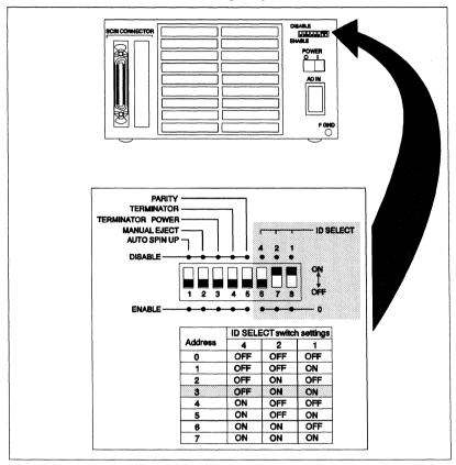
The termination switches at the rear of the unit are set differently when the drive is at the end of the bus and when the drive is in the middle of the bus. These settings are as follows:
