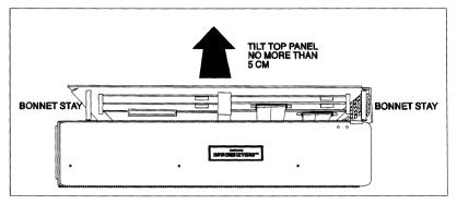
When the top panel is securely on the 'bonnet stays', the printed circuit boards and edge mounted switches can be accessed.
