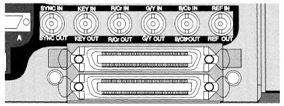
Note: Cables supplied by Quantel must be used at all times and all SCSI busses <u>MUST BE</u> terminated when not in use.
