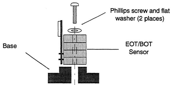
**Figure 9-8** EOT/BOT Sensor Assembly Mounting
