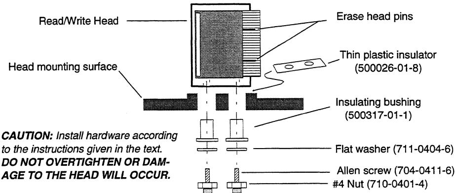
**Figure 9-6** Head Installation Hardware
