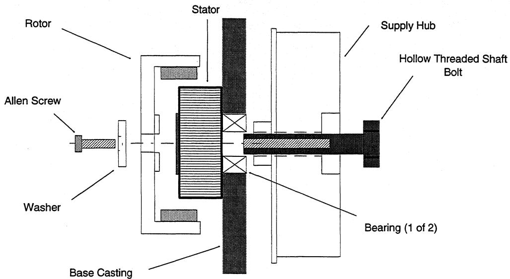
**Figure 9-9** Typical Motor Assembly
