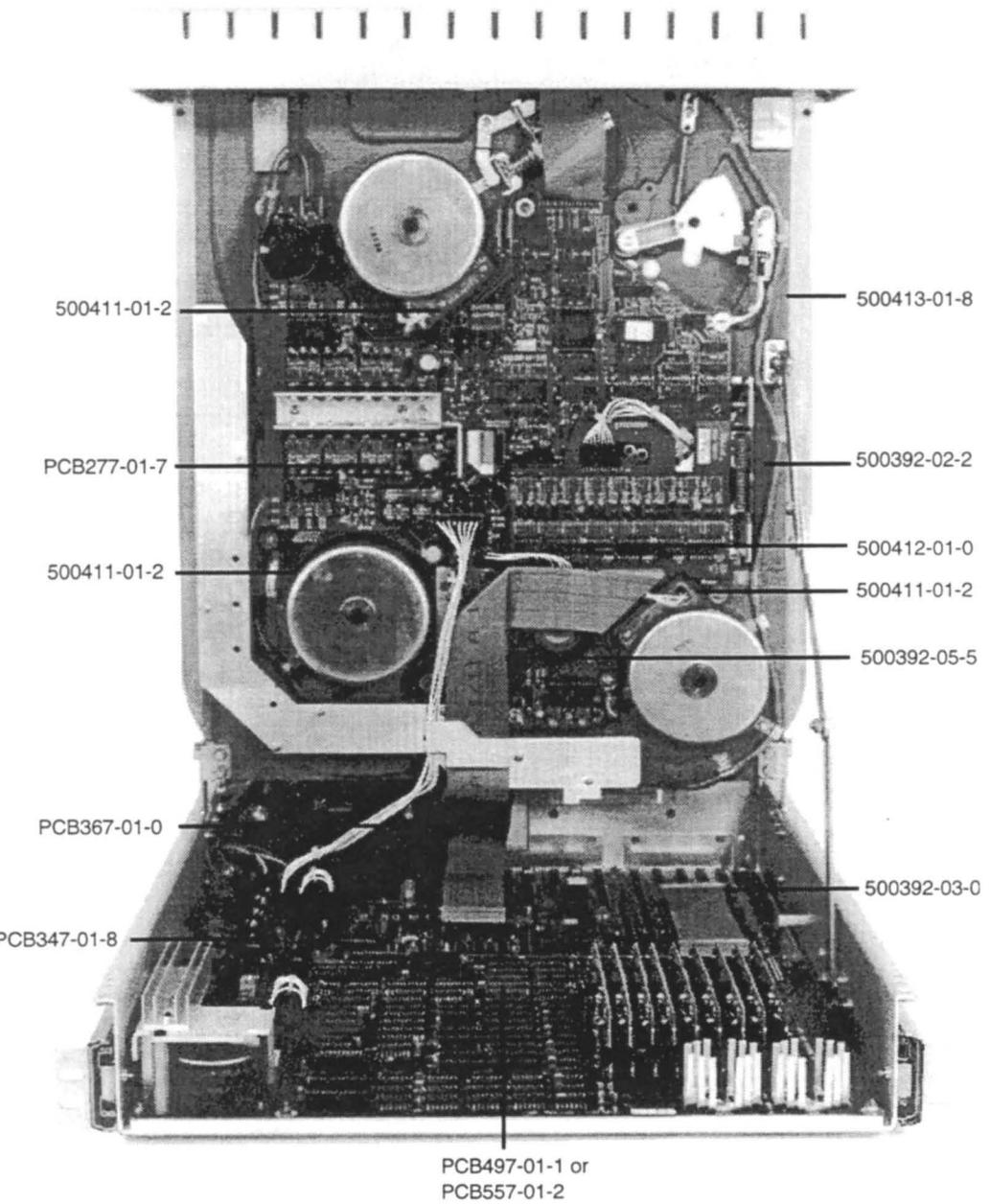
**Figure 13-3** 3410/3412 Internal Component Locations
