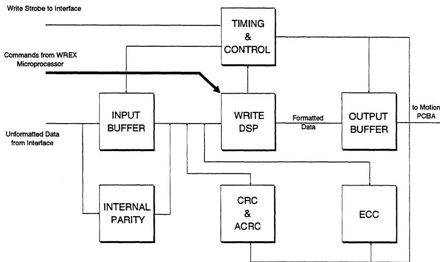
**Figure 5-1** Write Formatter Block Diagram
