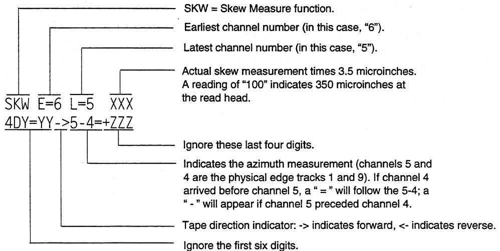
**Figure 10-1 Skew Measure Front Panel Display**
