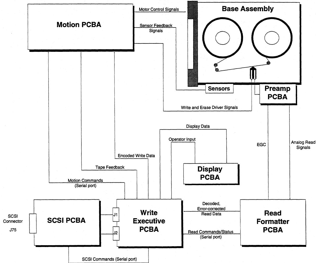
**Figure 2-1** 34XX Series General Block Diagram
