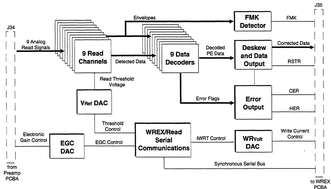
Figure 6-2 500497 Read Formatter Block Diagram
