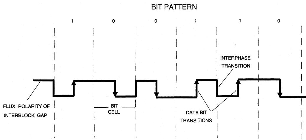
Figure 3-1 PE Data Bit Pattern
