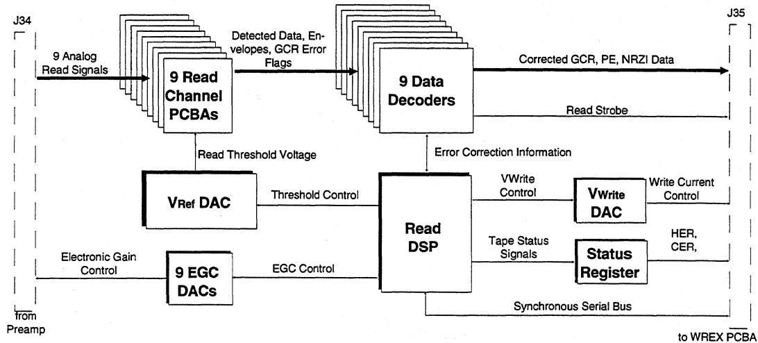
Figure 6-1 500377 Read Formatter Block Diagram
