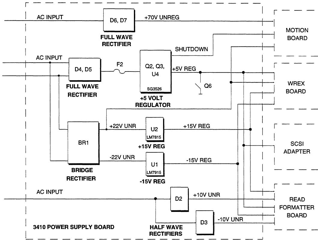
**Figure 4-3** Power Supply Block Diagram
