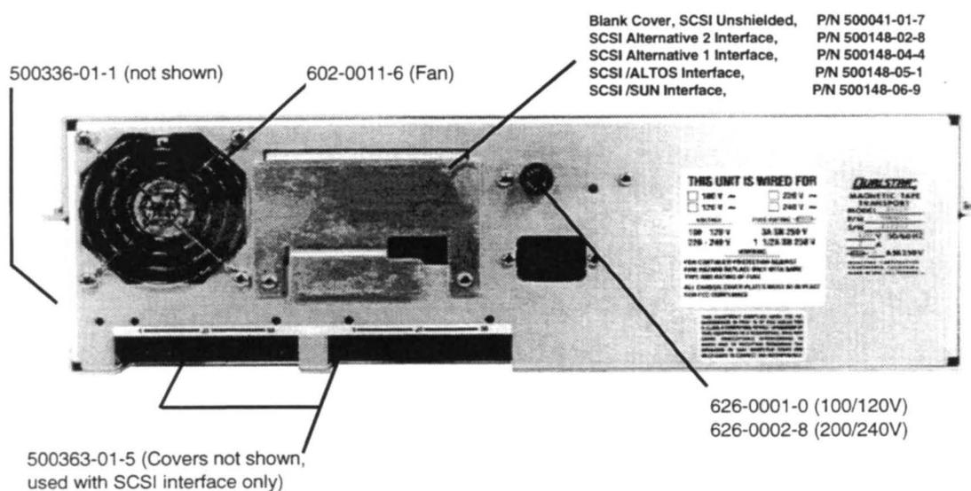
**Figure 13-2** 34XX Tape Drive, Rear View
