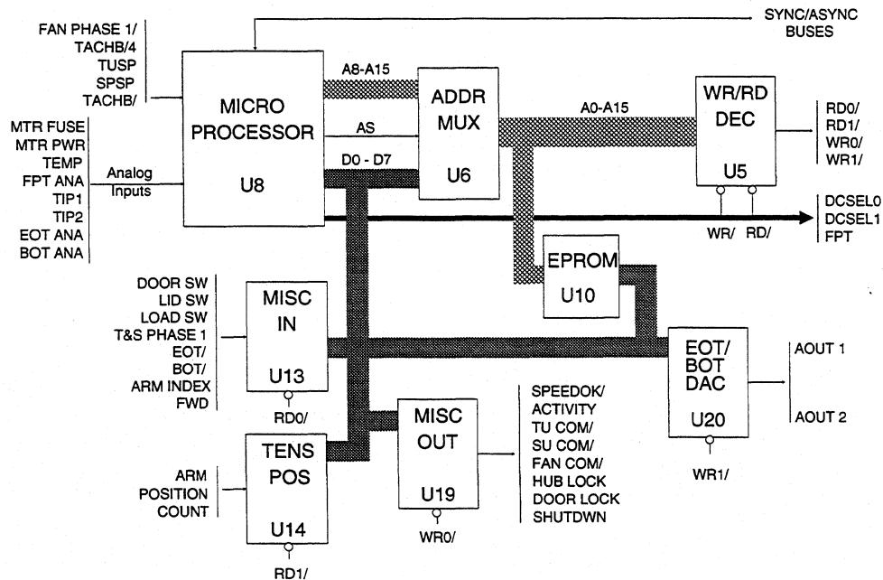
**Figure 4-1** Motion Board Microcomputer Block Diagram
