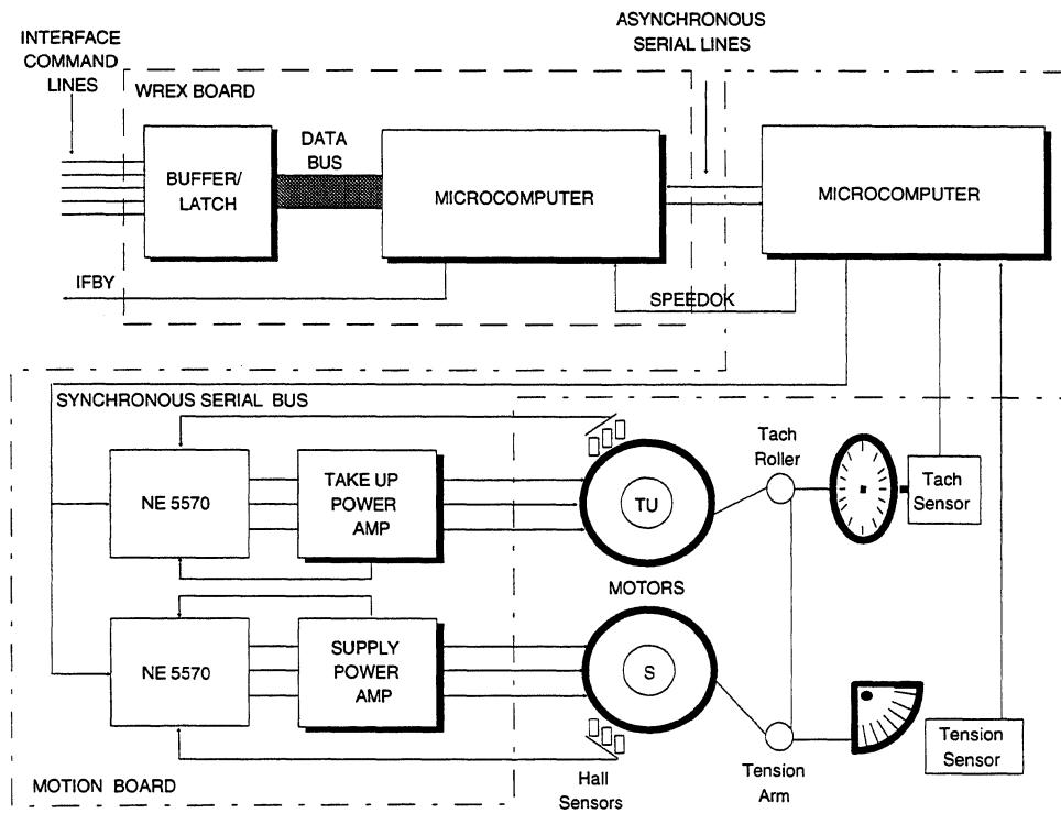
**Figure 4-2** Motor Control Block Diagram
