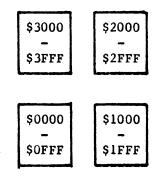
The MEM 3AP board has one switch with a "LO" (down) and a "HI" (up) position to distinguish low (first 16K) from high (next 16K) memory. This switch is set to the "LO" position if the board is the first memory board in the processor. It is set to the "HI" position on any other MEM3AP board.
