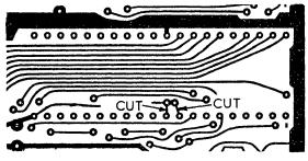
NOTE: If the DMA option is later removed (chips U15 and U16 removed) these traces MUST be re-installed or the SCCS-85 will not operate.
