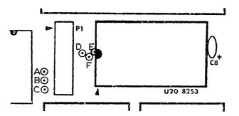
At this point possible reconfigurations should be apparent. If it is desired to supply any of the timers with clocks other than the CPU clock, one need only cut the appropriate trace under P1 (or trace D-E in the case of timer 1) and connect the desired clock. Note that if the clock is originating off the board, pin 1 of J3 has been conveniently routed to pin 9 of P1 for the user to connect to whatever he pleases.
