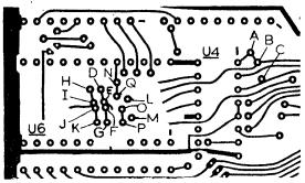
Step 3 Using short lengths of wire-wrap wire use two of the gates in the 74LSOO chip to add the following circuit to the board:
