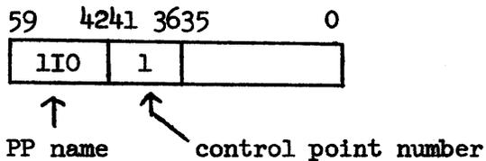
It then writes this word into the first word of the message buffer in the PP9 communication area. It next writes the MTR function code to request a PPU in the output register. PP9 then enters a waiting loop which scans the output register constantly. If MTR does not respond within a fixed time period, a "SYSTEM BUSY" message will be displayed
