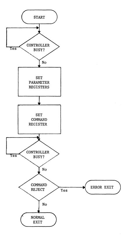
Figure 1. Basic Command Flow
