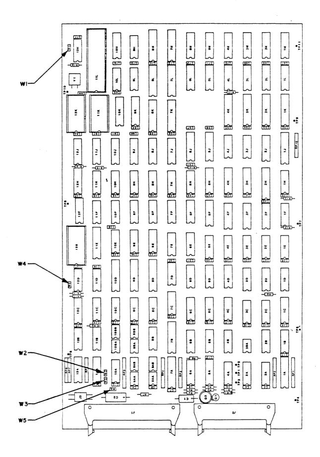
FIGURE 1. SMART Jumper Locations
