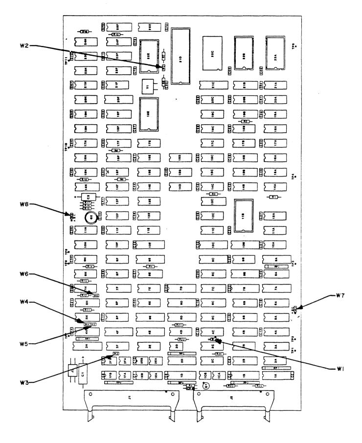
Figure 2. SMART-E Jumper Locations
