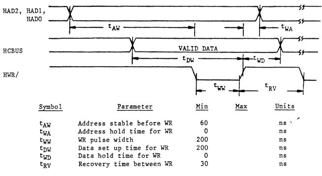
Figure 6 - SMART-E Register Write AC Characteristics
