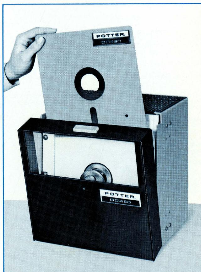
insure proper head-disk contact, is retracted. In addition, should no further commands occur within one and one half additional revolutions, the disk drive motor may be turned off. These features, along with the overall simplicity, provide long term reliability.
