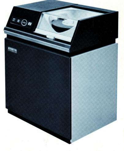
The Potter DD 4314-1 Disk Storage Drive is a random access device which provides an "on-line" capacity of 233 million bits. The unit is capable of reading and writing on disk surfaces and utilizes the IBM 2316 Disk Pack or equivalent. Each disk pack can be removed and interchanged between disk drives in a simple and rapid operation.
