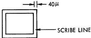
5.1.3.2 Distance from inside edge of scribe line to adjacent bonding pad, Building Block, P or metal line:  $50\ \mu$
