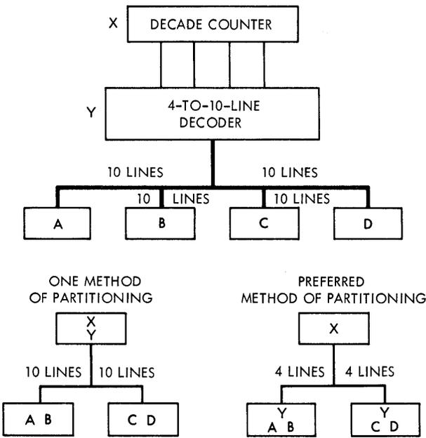
Fig. 4.3 Minimizing Area by Redundancy.
