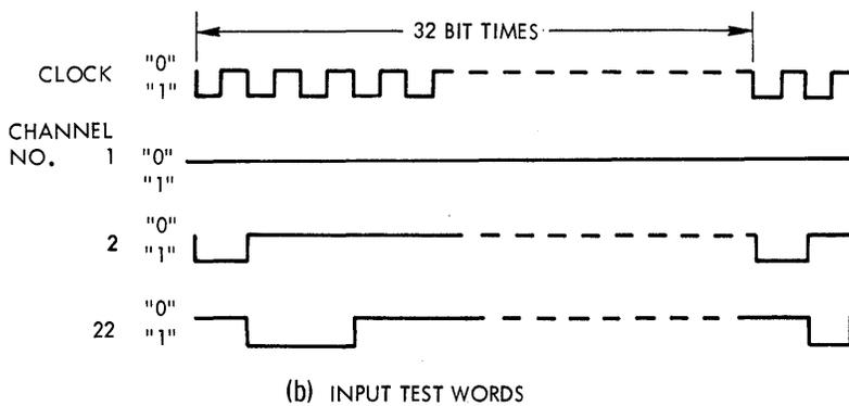
*Fig. 7.5 Program Card and Input Test Words.*
