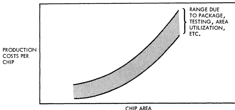
Fig. 4.1 Graph of Relationship Between Production Costs per Chip and Chip Area.
