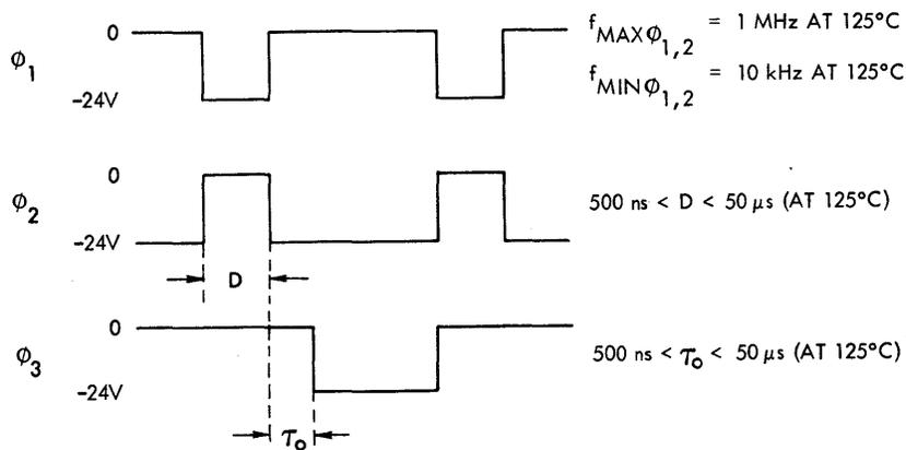
Fig. 3.7 One-Bit DC Shift Register Stage (BB-403) and Clock Waveforms.
