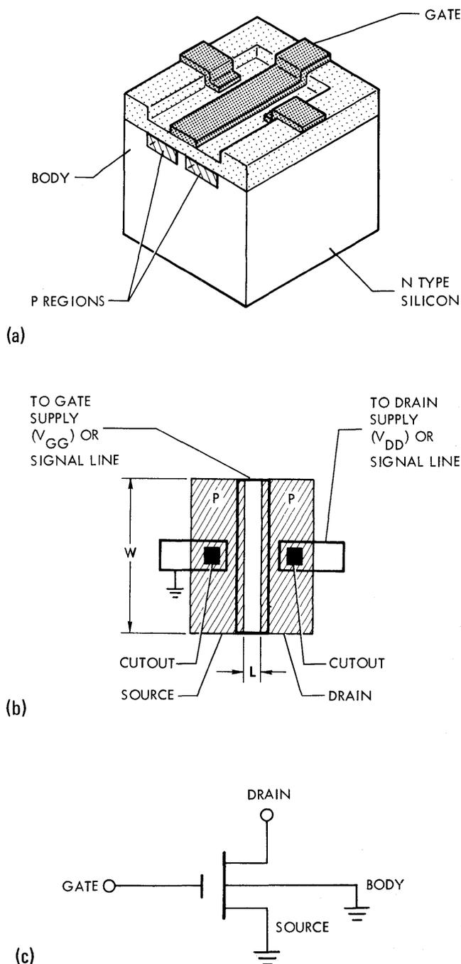
Fig. 2.1 The MOS Transistor: (a) Three-Quarter View; (b) Stylized Top View; (c) Schematic Diagram.
