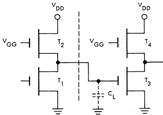
Fig. 2.5 Two Building-Block Inverter Stages.
