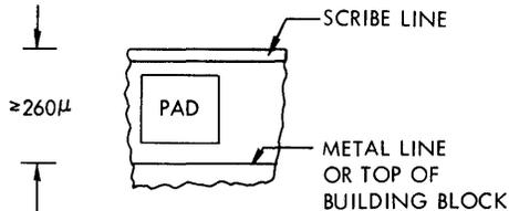
5.1.7 Rules for Placement of Lines Between Building Blocks\*
