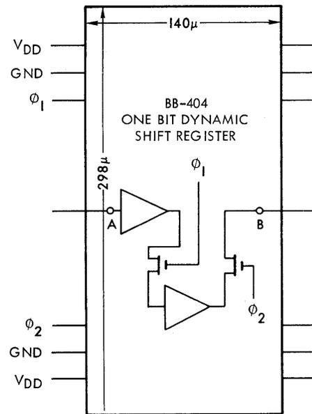
Fig. 5.6 Block Outline of BB-404, the One-Bit Dynamic Shift Register.
