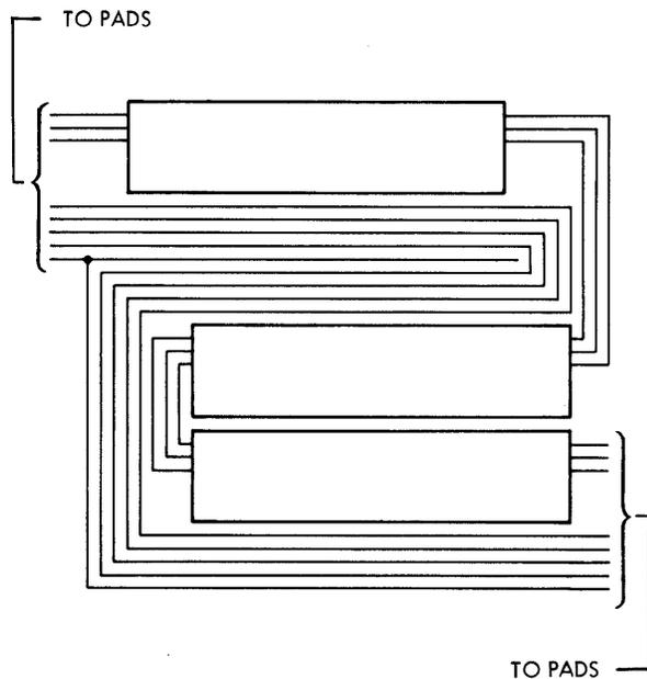
Fig. 5.4 Layout Suggested as Alternative to Very Long Rows of Blocks.
