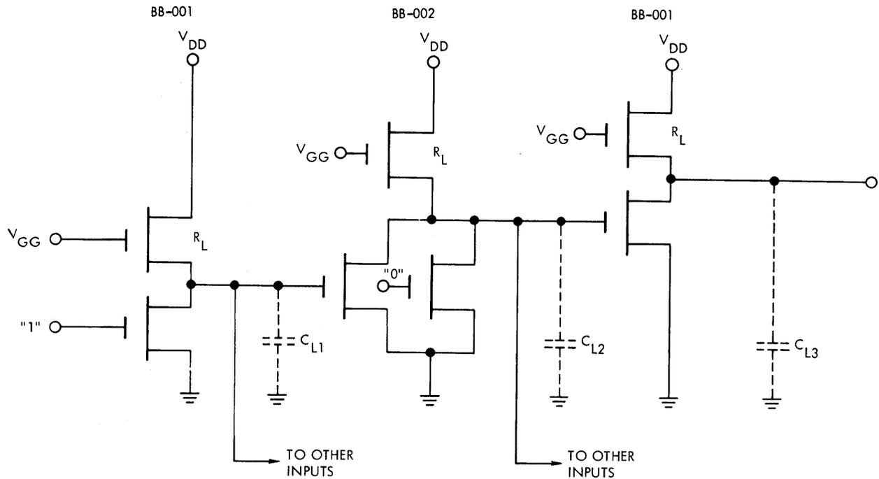
Fig. 6.3 Three Blocks in Cascade.
