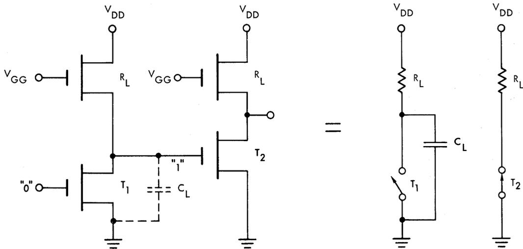
Fig. 2.6 Isolation of Input from Output Stage.
