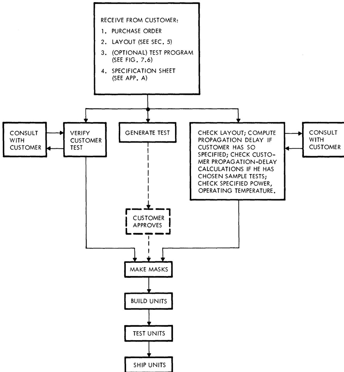
Fig. 8.1 Flow Chart Showing Procedure for Ordering, Manufacturing, and Shipping of Building-Block Arrays.
