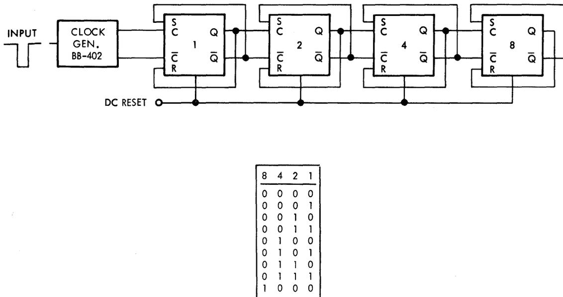
Fig. 3.5 Four-Stage Binary Ripple-Through Counter Using Master-Slave Flip-Flops.
