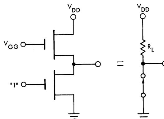
Fig. 2.3 Inverter with “1” on its Gate and Equivalent Circuit.
