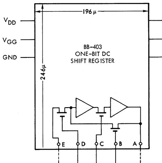
Fig. 5.5 Block Outline of BB-403, the One-Bit DC Shift Register.
