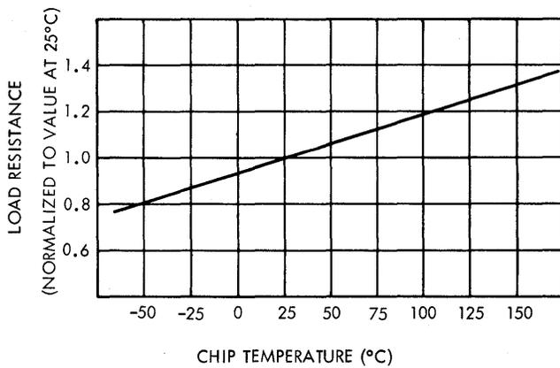
Fig. 6.6 Load Resistance versus Chip Temperature.
