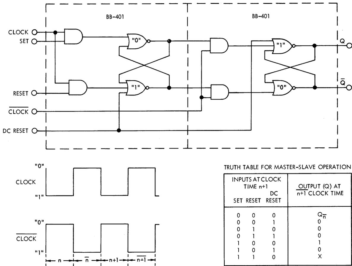
Fig. 3.4 Logic Diagram, Truth Table and Clocks for Master-Slave Flip-Flop.
