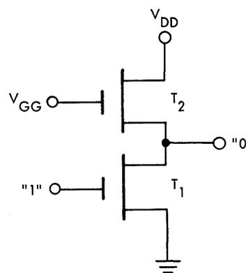
Fig. 2.2 Schematic Diagram of Building-Block Inverter Stage.
