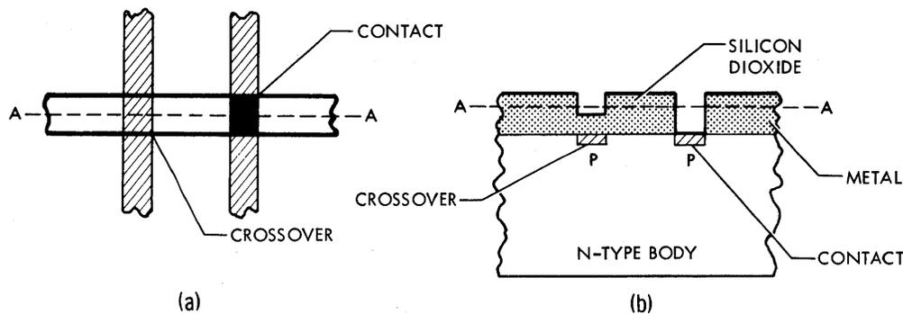
Fig. 2.7 P and Metal Interconnect Lines: (a) Stylized Top View; (b) Cross-Section.
