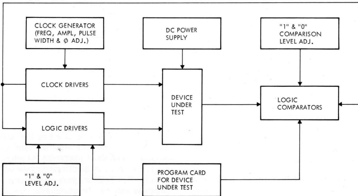
Fig. 7.4 Functional Block Diagram of MOS Tester.
