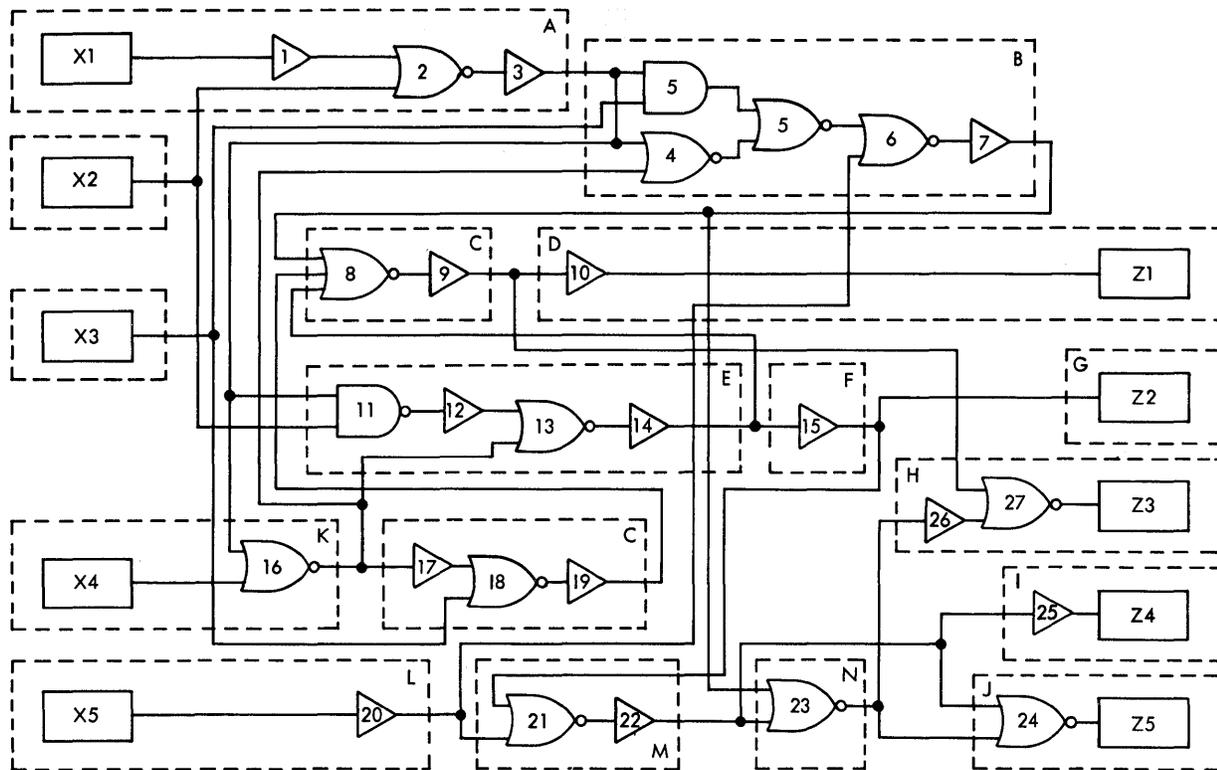
Fig. 5.9 Partitioning Logic for Layout by Simple Matrix.
