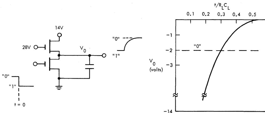
Fig. 6.2 Turn-on Waveform of MOS Inverter with Step Input.
