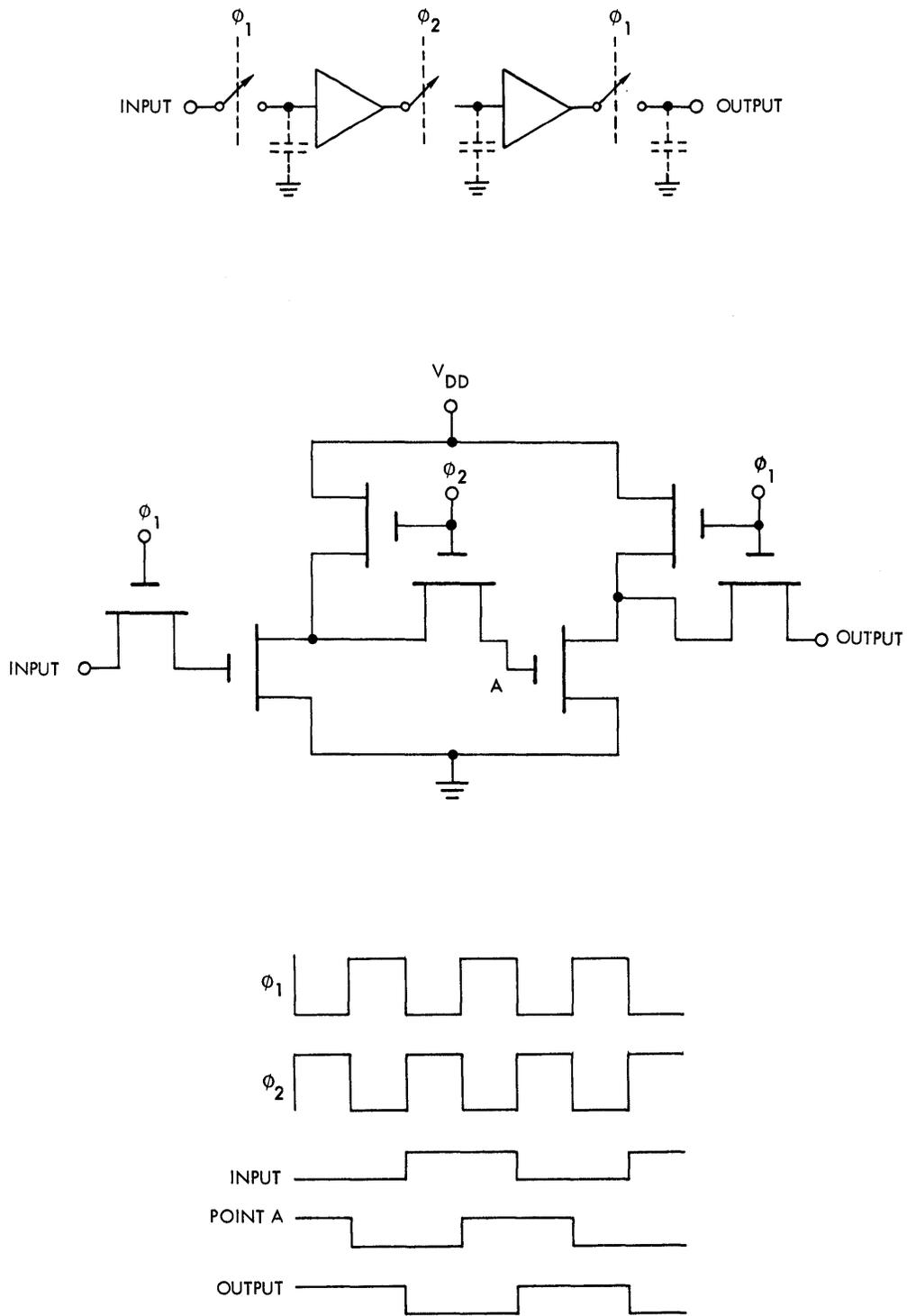
Fig. 3.8 One-Bit Dynamic Shift-Register Stage (BB-404) and Clock Waveforms.
