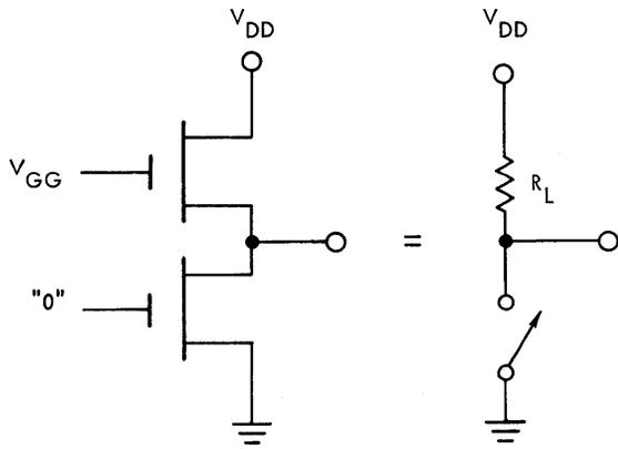
Fig. 2.4 Inverter with "0" on its Gate and Equivalent Circuit.
