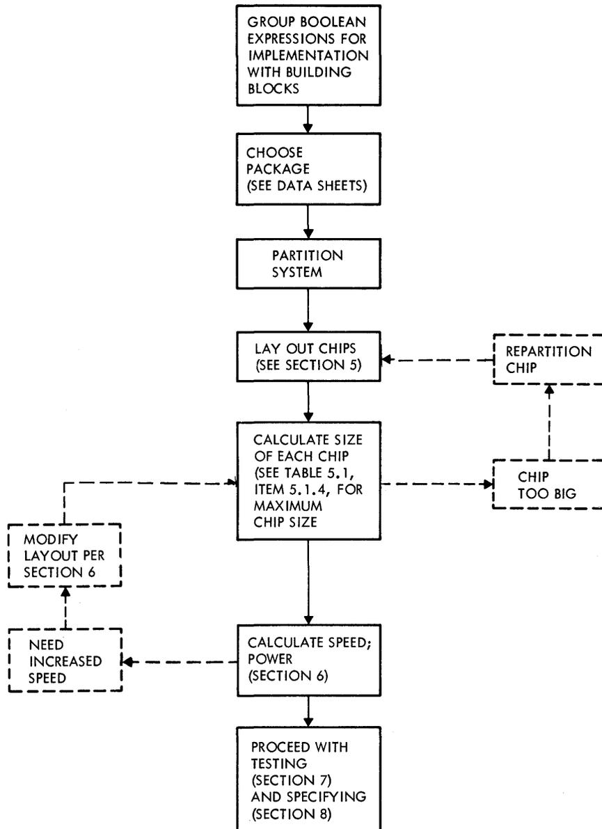
Fig. 4.4 Flow Chart of Steps in Partitioning and Laying Out a Building-Block System.
