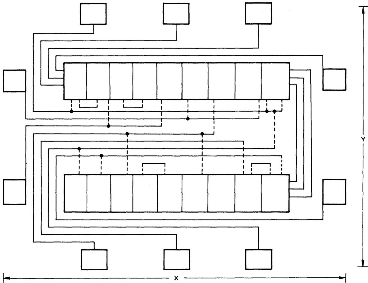
Fig. 5.3 Block Layout with Bonding Pads at Periphery of Chip
