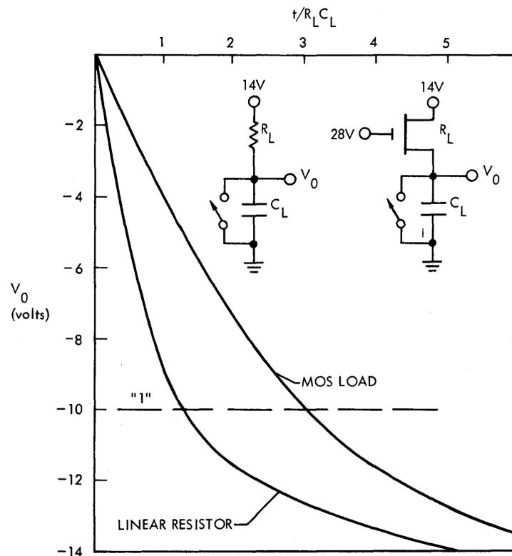
Fig. 6.1 Typical Turn-off Waveforms with MOS Load and Simple Linear Resistor.
