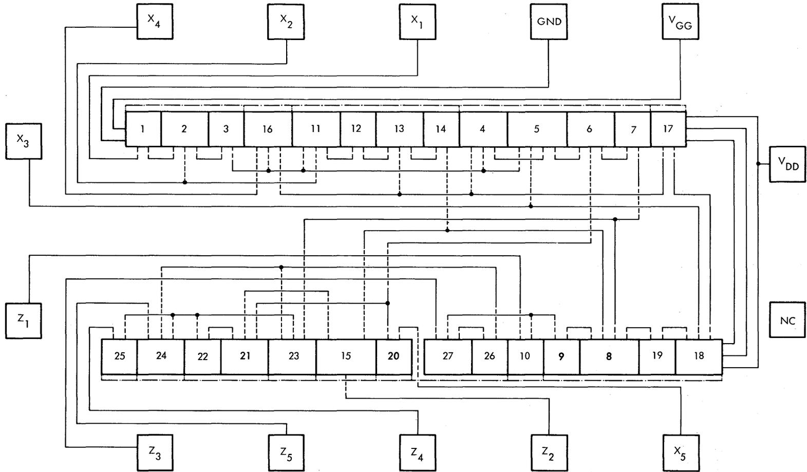
Fig. 5.12 Layout of Logic in Fig. 5.7 by Simple Matrix.
