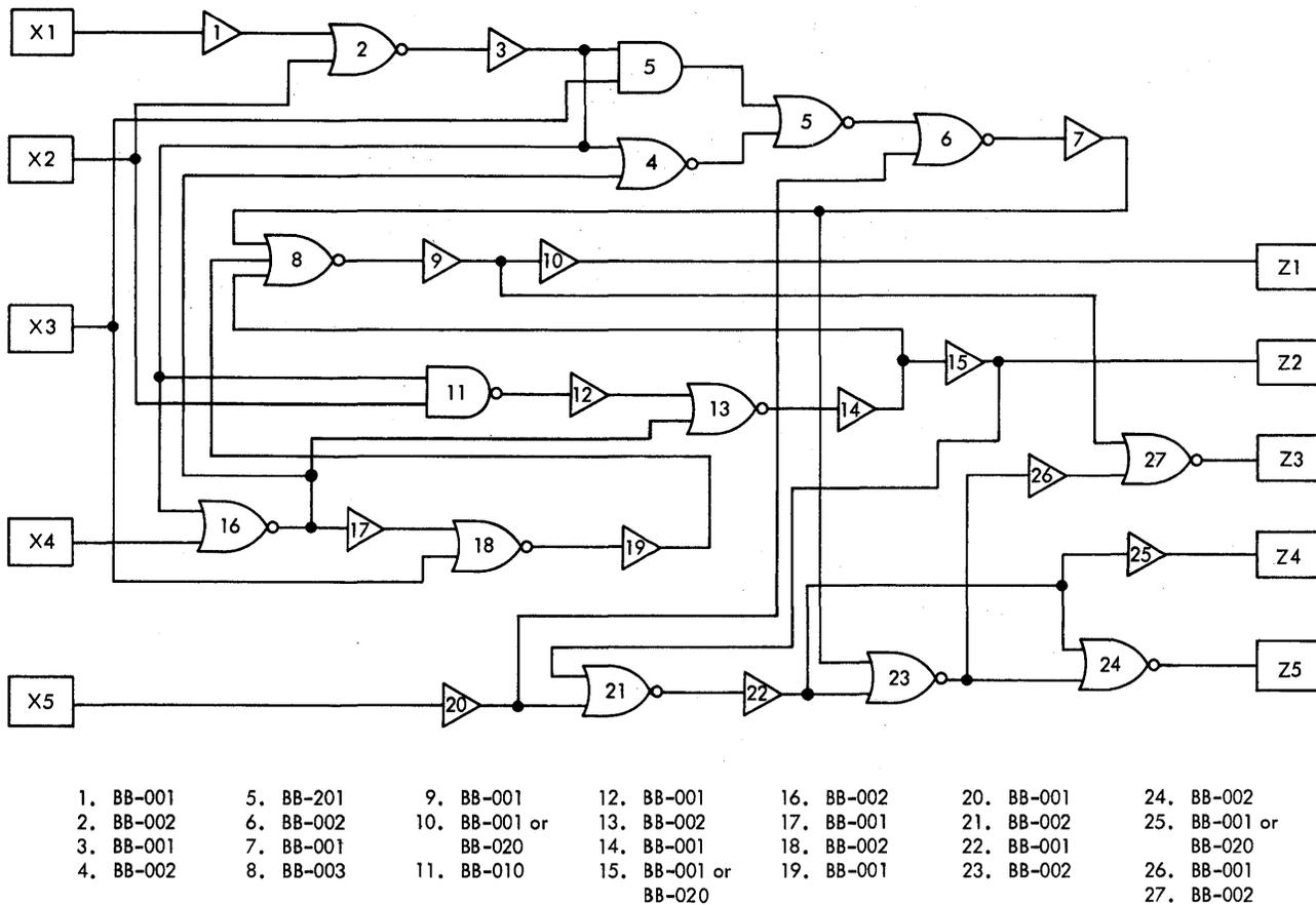
Fig. 5.7 Hypothetical Logic Diagram to be Laid Out on a Chip.
