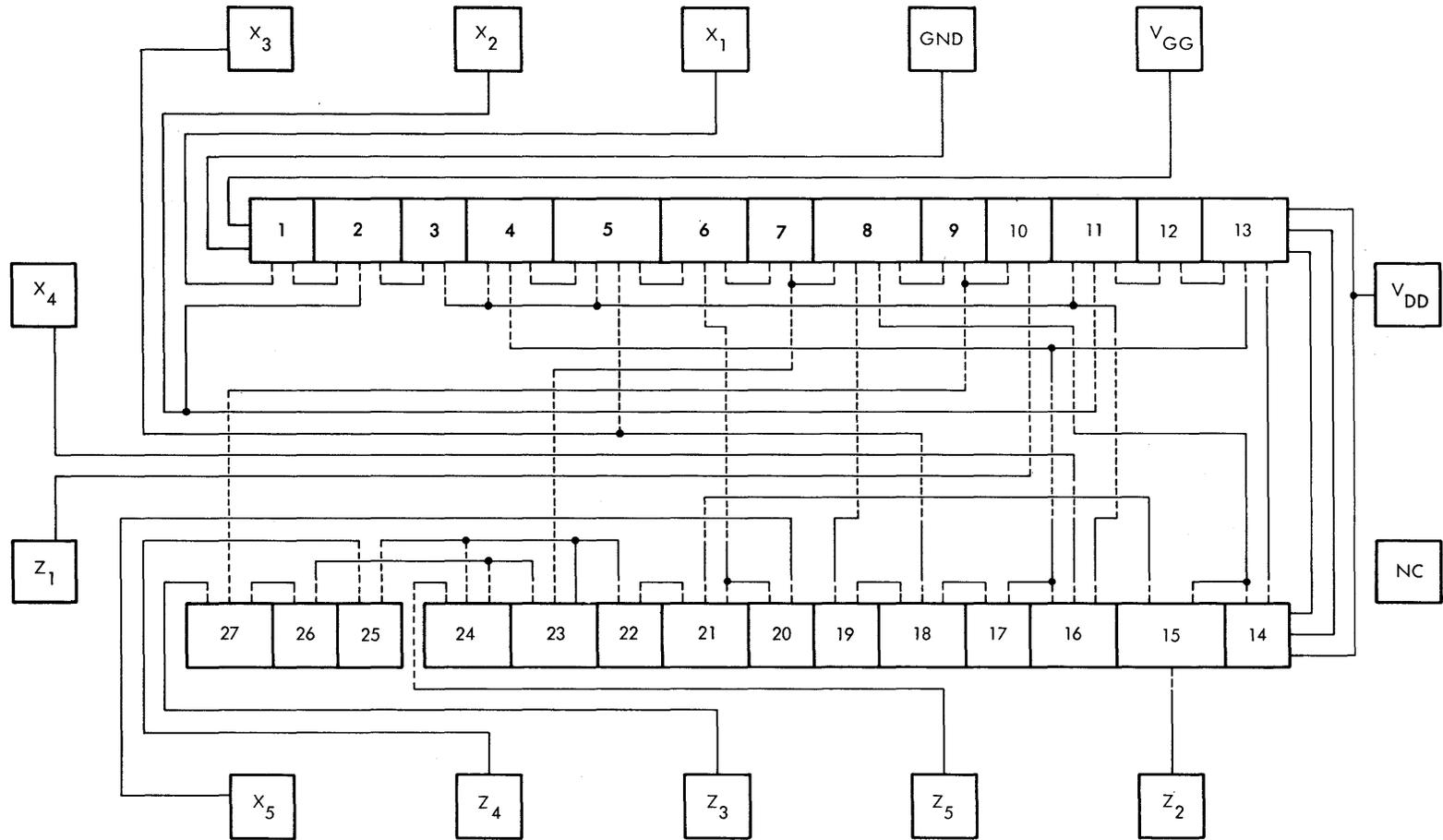
Fig. 5.8 Layout "By Eye" of Logic in Fig. 5.7.
