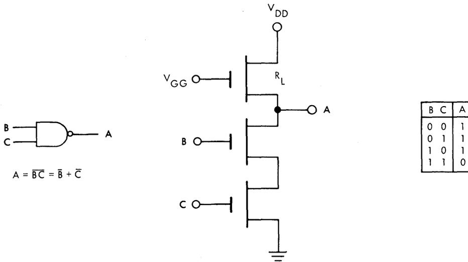
Fig. 3.2 Basic NAND Gate: Logic Diagram, Circuit Diagram and Truth Table
