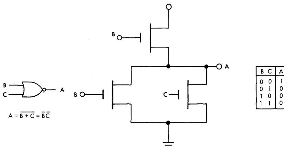
Fig. 3.1 Basic NOR Gate: Logic Diagram, Circuit Diagram and Truth Table.
