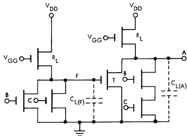
Fig. 6.5 Schematic Diagram of BB-101.
