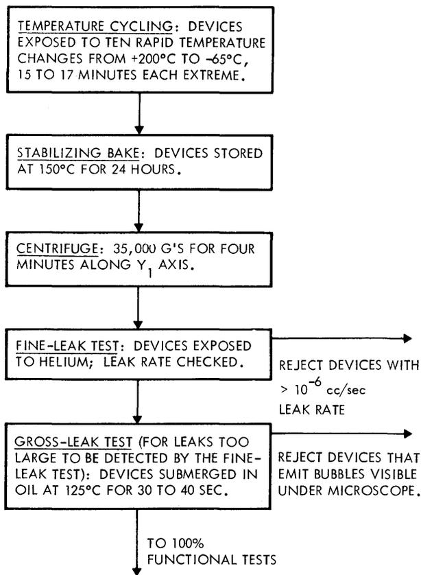
Fig. 7.2 100% Environmental Tests (Flatpacks).
