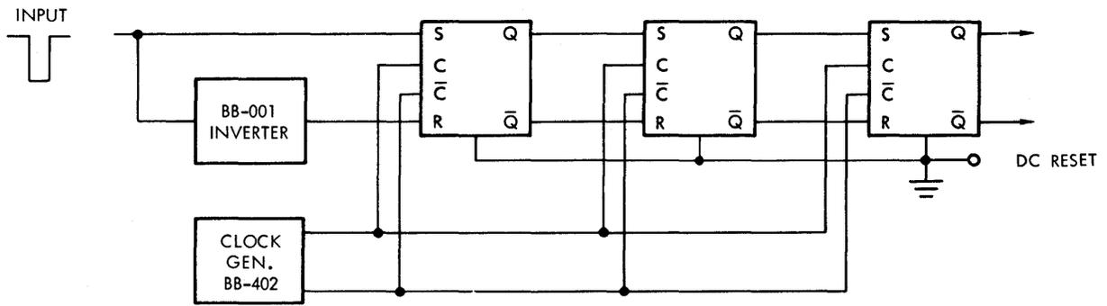
Fig. 3.6 Master-Slave Shift Register.
