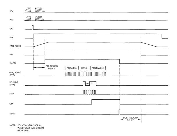
Figure 4-5. PE Read Operation Illustrating Error Correction for Last Two Data Bytes
