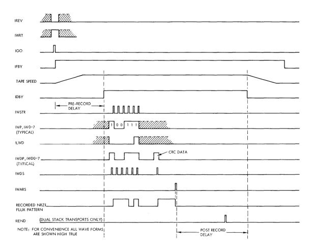
Figure 4-2. 9-Channel NRZI Write Operation
