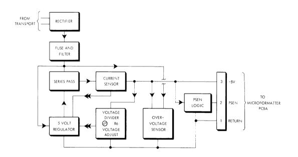
Figure 4-7. Power Supply Functional Block Diagram
