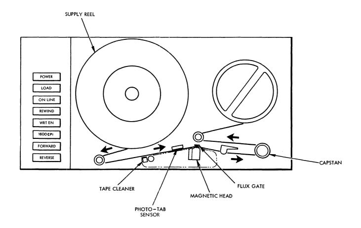
Figure 3-1. Model T7640 Tape Path and Controls
