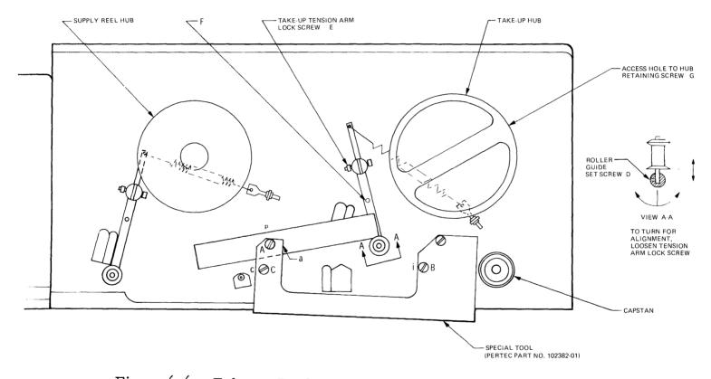
Figure 6-6. Take-up Reel Tension Arm Guide Roller Adjustments
