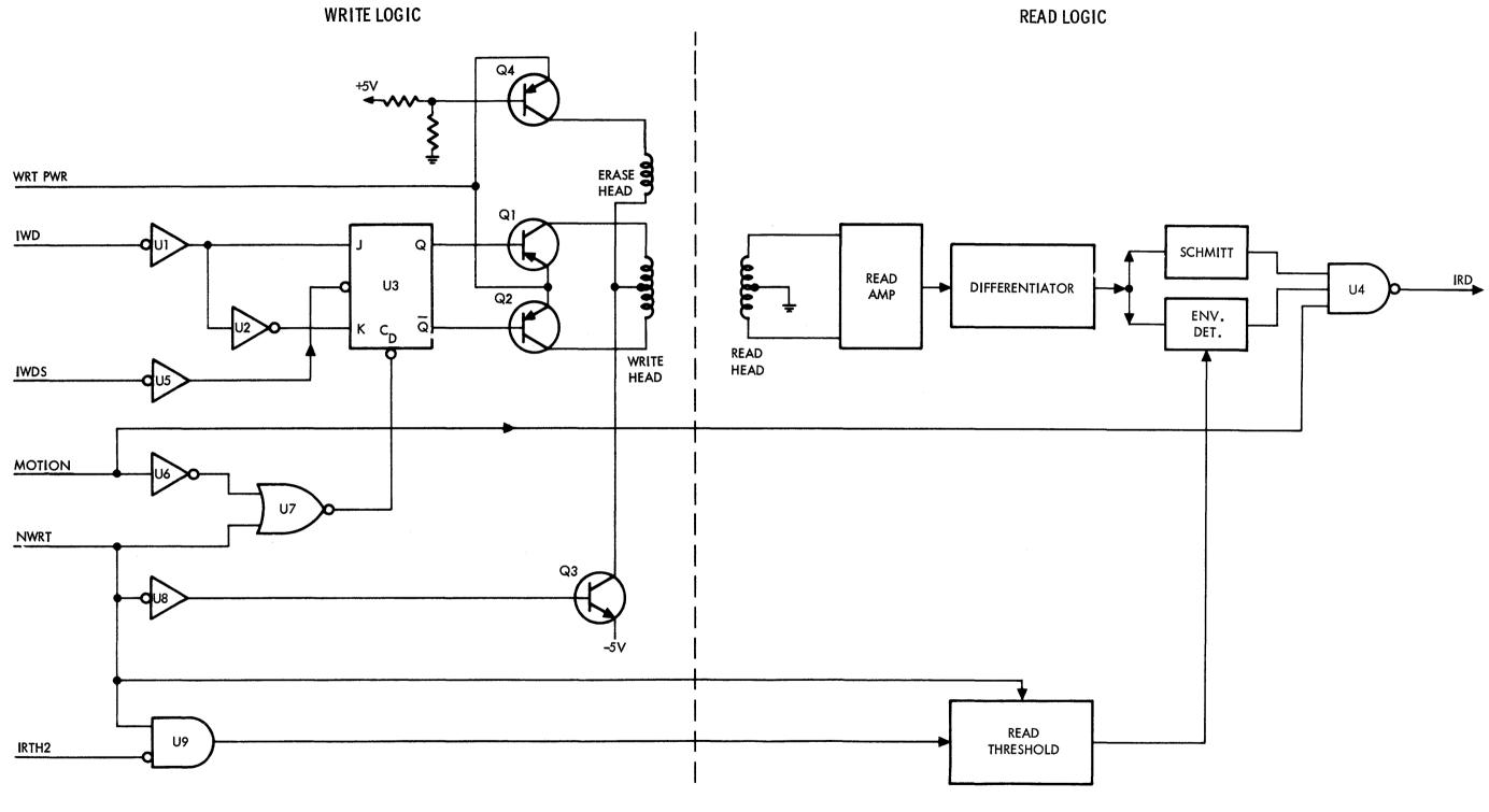
Figure 4-10. One Channel of Data Electronics
