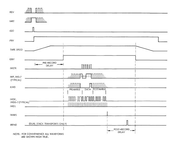
Figure 4-3. 9-Channel PE Write Operation
