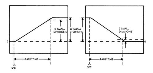
Figure 6-1. Ramp Levels and Timing
