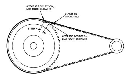
Figure 6-5. Reel Servo Belt Tension Adjustment
