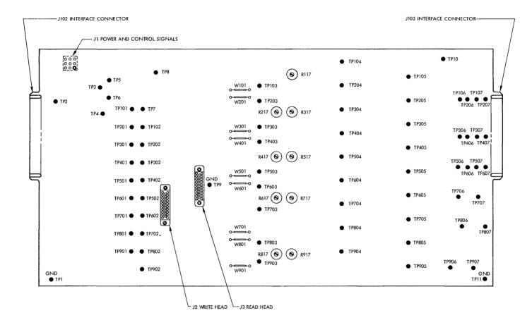
Figure 5-2. Data H PCBA Connector and Test Point Location
