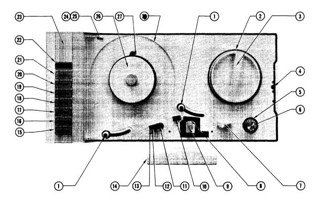
Figure 7-1. T7640 Transport Photo Parts Index
