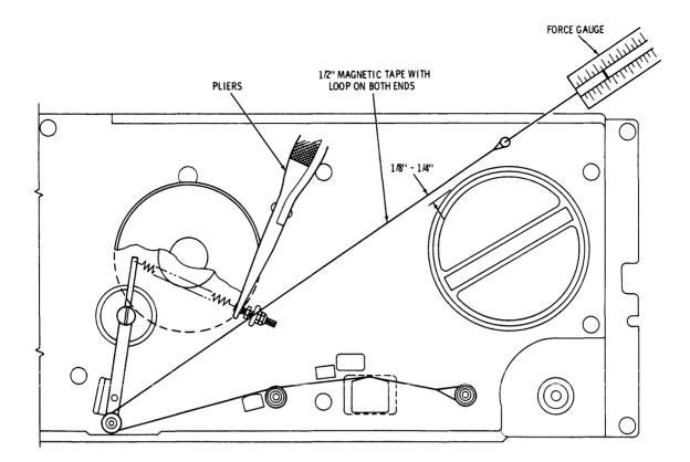
Figure 6-8. Tension Adjustment for Supply Reel
