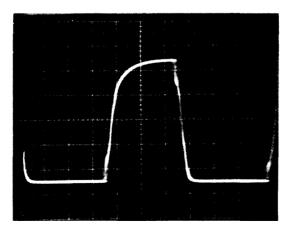
Figure 6-3. Skew Waveform (Typical)
