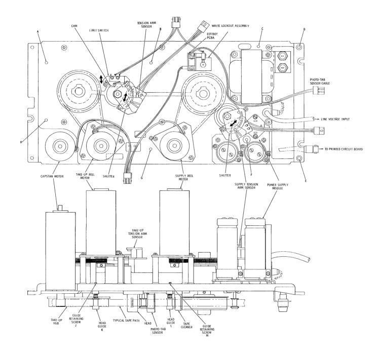
Figure 6-2. Tape Deck Diagram (Rear View)
