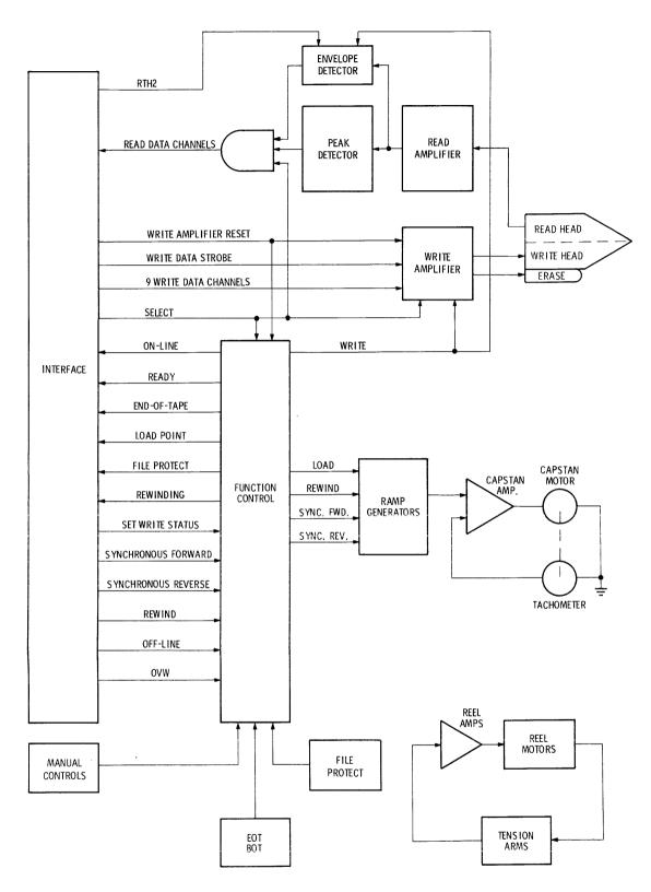
Figure 1-3. Block Diagram of Model T7640 Tape Transport
