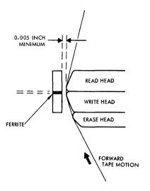
Figure 6-4. Flux Gate Adjustment
