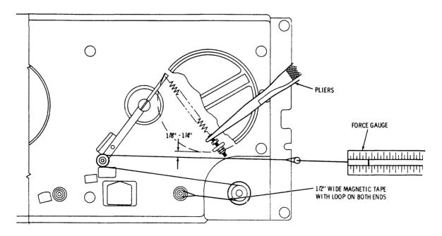
Figure 6-9. Tension Adjustment for Take-up Reel
