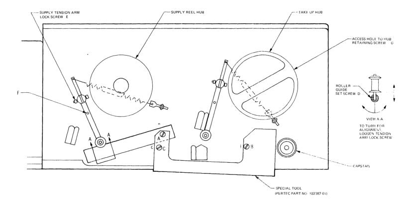
Figure 6-7. Supply Reel Tension Arm Guide Roller Adjustments
