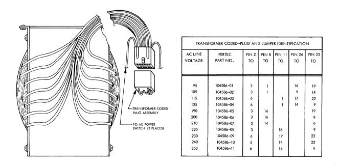
Figure 4-3. Transformer Primary Connections
