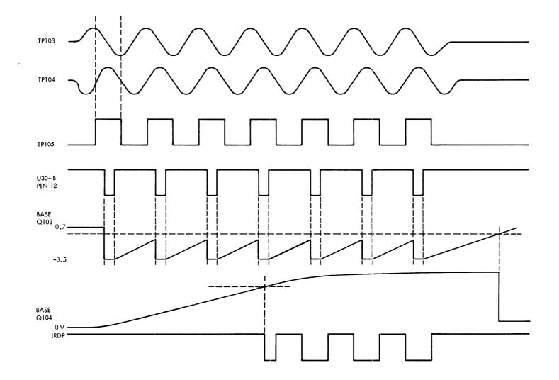
Figure 5-3. Timing and Signal Relationships, One Channel Read Electronics
