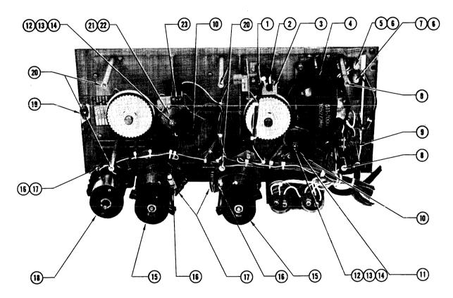
Figure 7-3. T7000 Series Transports Photo Parts Index
