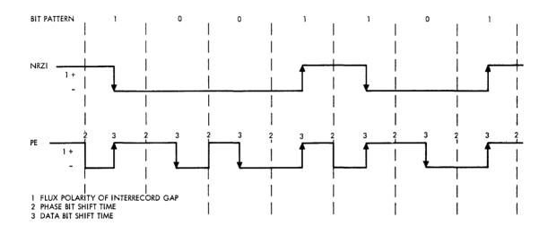
Figure 4-7. Comparison of NRZI and PE Recording Modes
