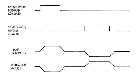
Figure 4-5. Typical Capstan Servo Waveforms
