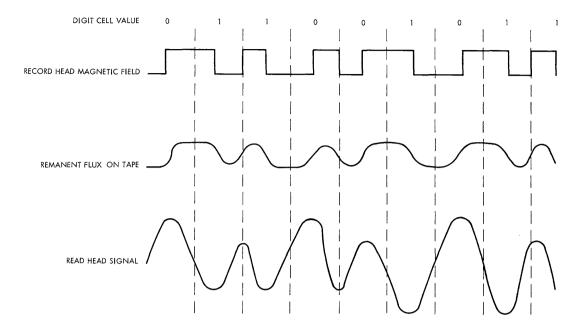
Figure 3-2. PE Write and Read Waveforms
