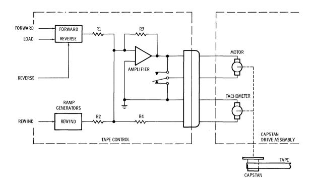
Figure 4-4. Capstan Servo Block Diagram
