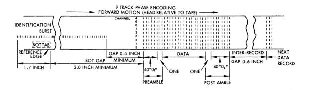
Figure 4-8. 9-Track PE Allocation, Spacing and Format
