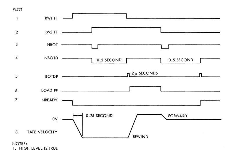
Figure 4-15. Tape Control Waveforms During Rewind to Load Point Sequence
