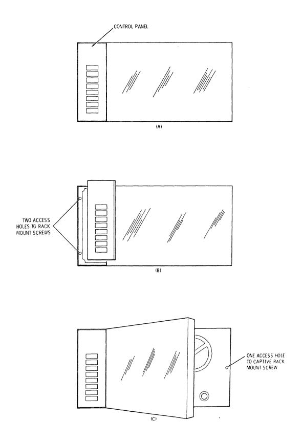
Figure 2-2. Rack Mounting the Transport
