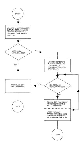
Figure 4-6. Fault Isolation Flow Chart
