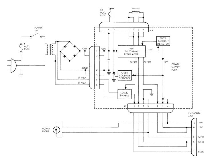
Figure 4-2. Block Diagram, Power Supply Subassembly
