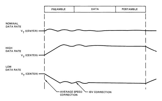
Figure 5-7. Operation of Tracking Oscillator
