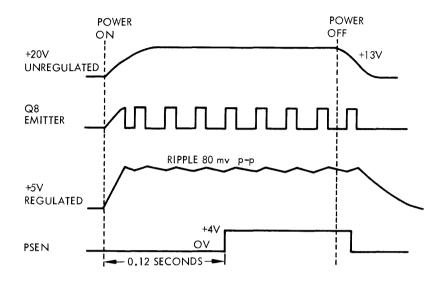
Figure 5-4. Switching Regulator Waveforms
