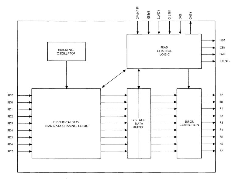
Figure 4-6. Read Recovery PCBA, Simplified Block Diagram
