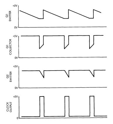
Figure 5-5. Fixed Oscillator Waveforms
