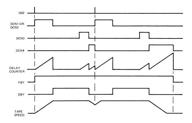
Figure 5-12. On-the-Fly Operation
