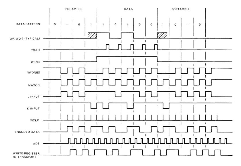
Figure 5-15. Write Data Encoding
