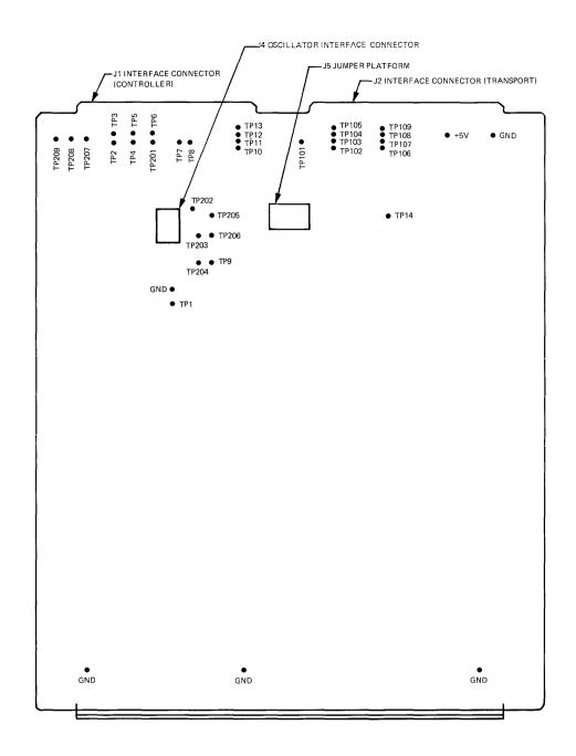
Figure 5-16. PE Read Recovery PCBA, Test Point and Connector Placement
