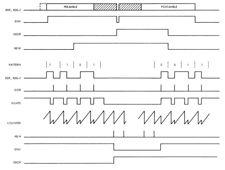
Figure 5-19. Envelope and Drop Waveforms
