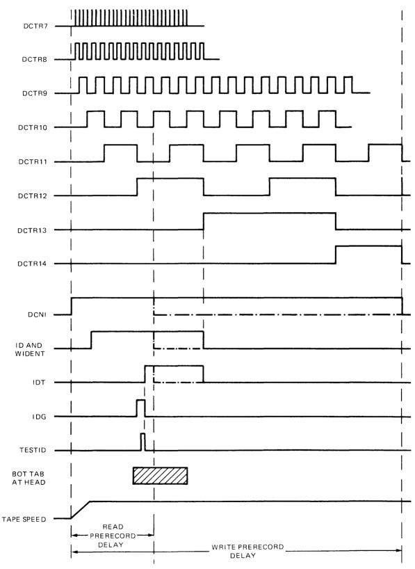
Figure 5-13. Identification Timing, Read and Write
