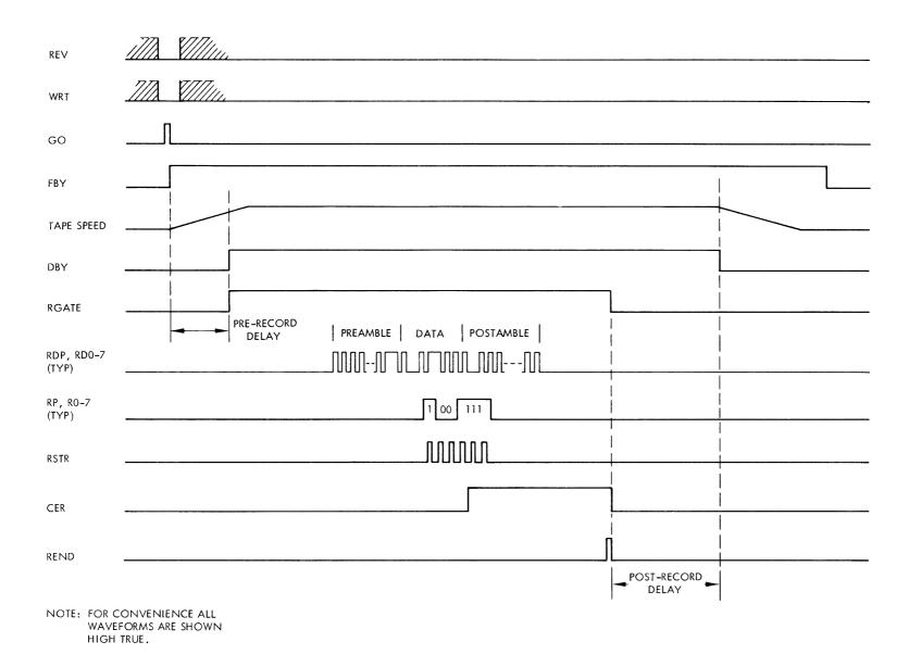
Figure 4-8. Phase Encoded Read Operation Illustrating Error Correction for Last Two Data Bytes
