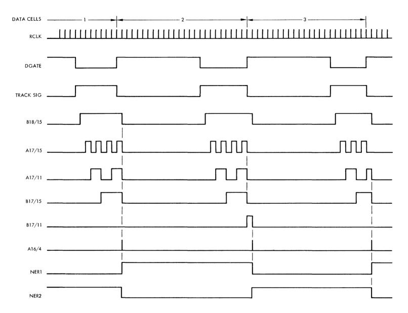
Figure 5-21. Tracking Control Waveforms
