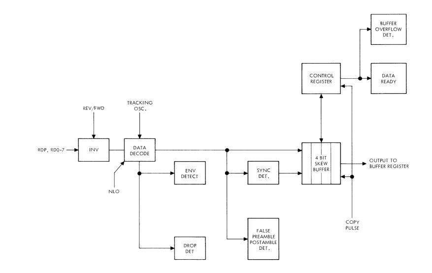
Figure 4-7. Read Data Channel Logic
