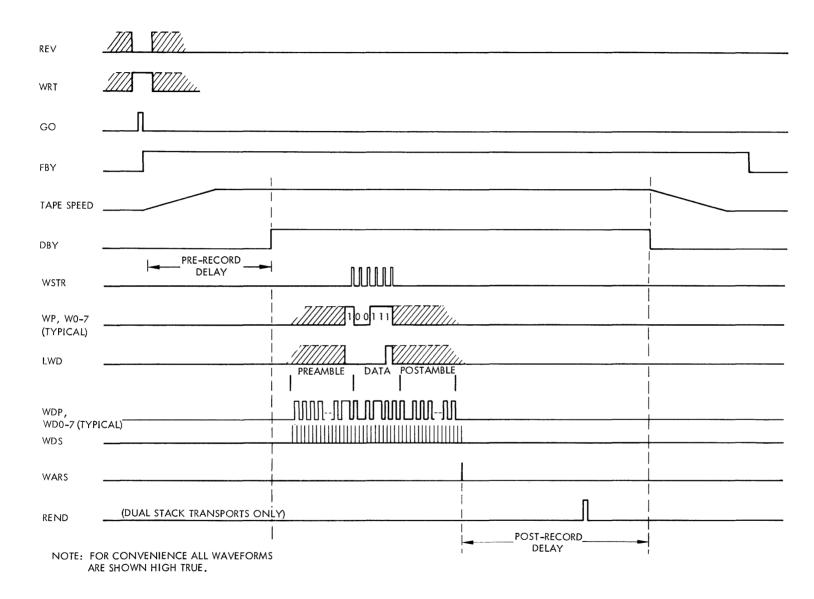
Figure 4-5. Phase Encoded Write Operation
