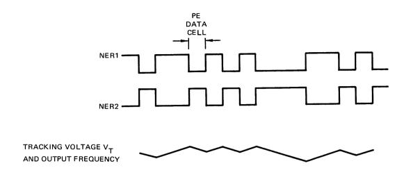
Figure 5-6. Tracking Oscillator Control Waveforms
