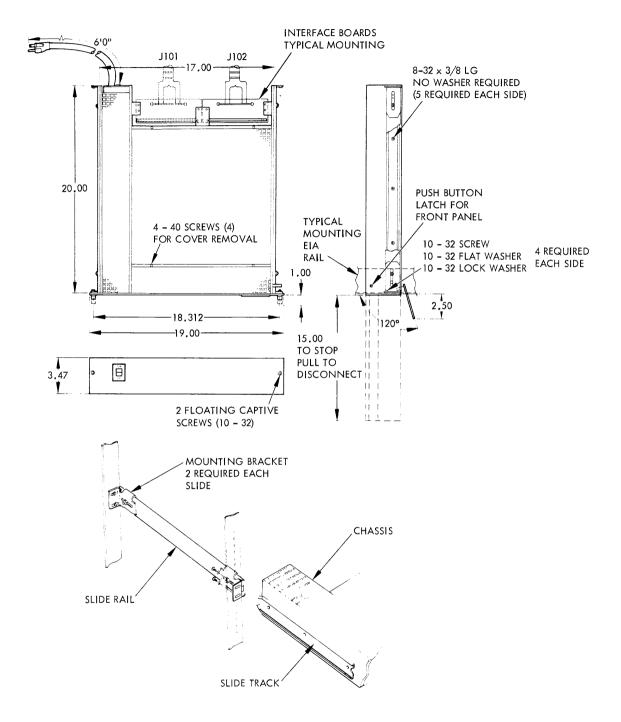
Figure 2-2. Rack Mounting the Formatter
