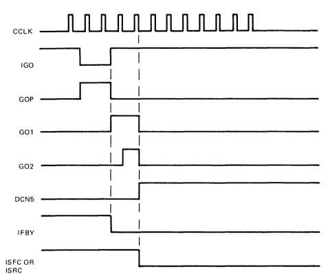
Figure 5-10. Command Initiation Waveforms
