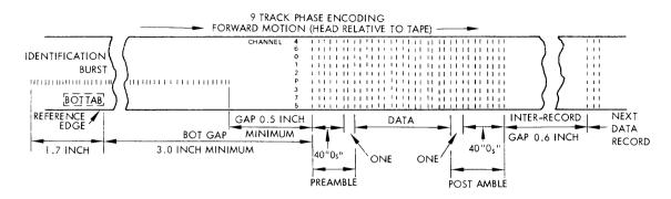
Figure 3-1. 9-track PE Tape Format
