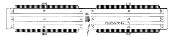
Figure 4-1. Physical Relationship between the Motherboard Connectors, Three Card Slots, and Interface Cables
