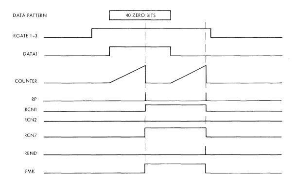
Figure 5-25. File Mark Waveforms
