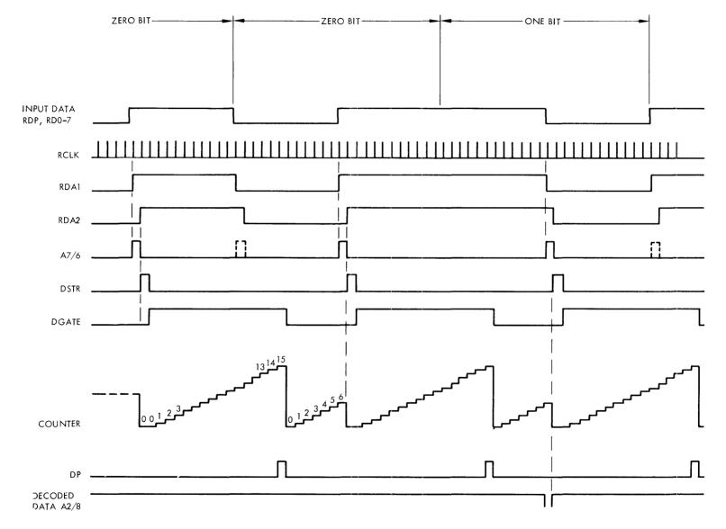
Figure 5-18. Data Decoding Waveforms
