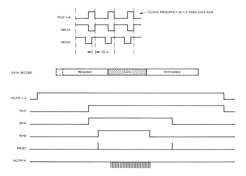
Figure 5-22. Control Signals to Data Channels
