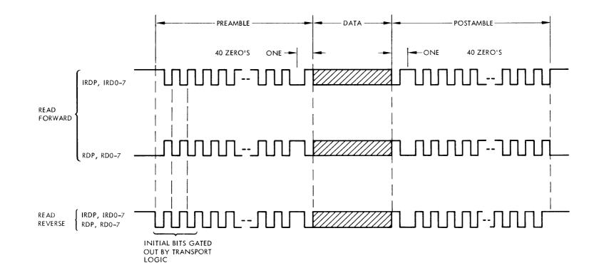
Figure 5-17. Read Input Signals
