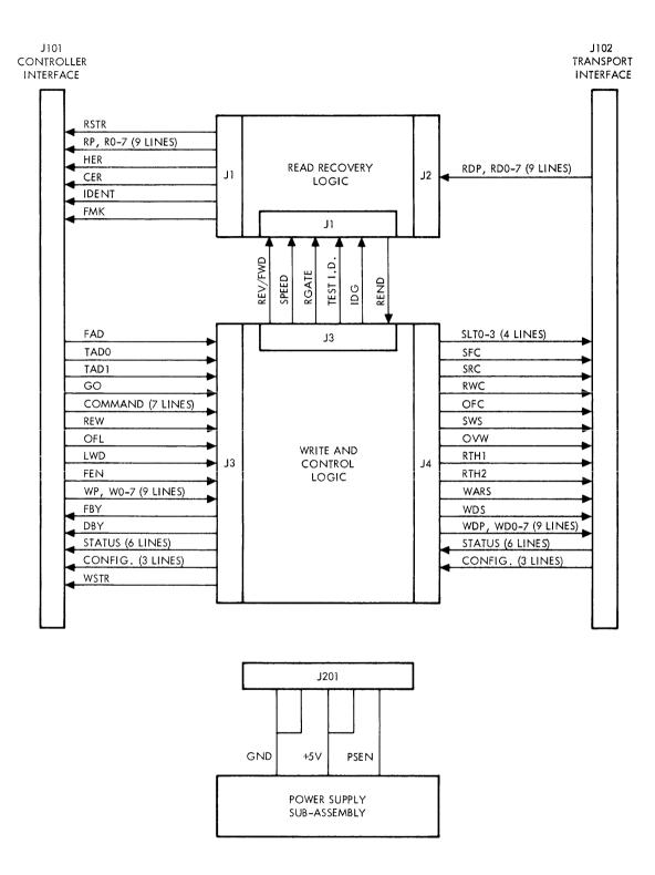
Figure 4-3. Phase Encoded Formatter Organization
