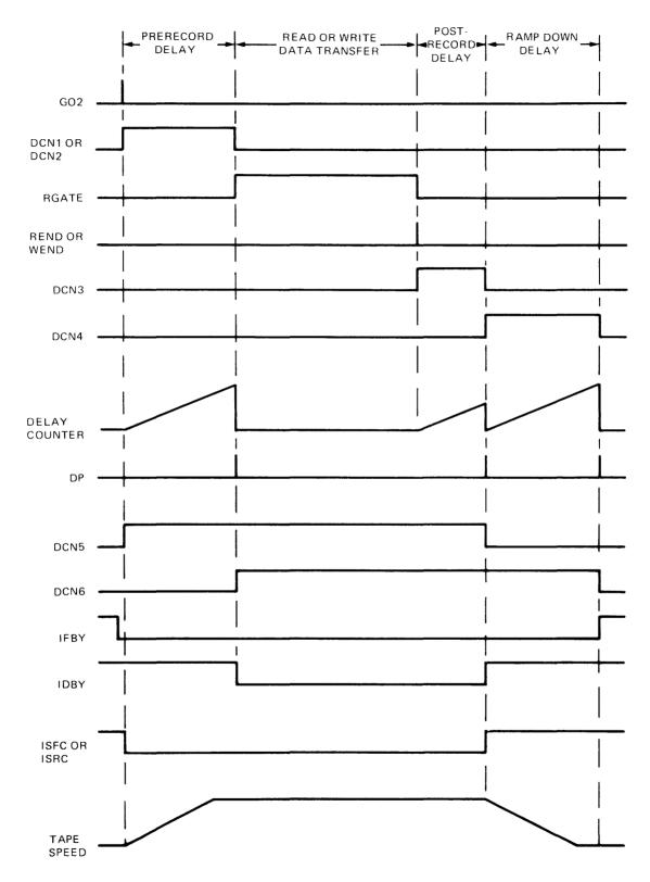
Figure 5-11. Command Timing
