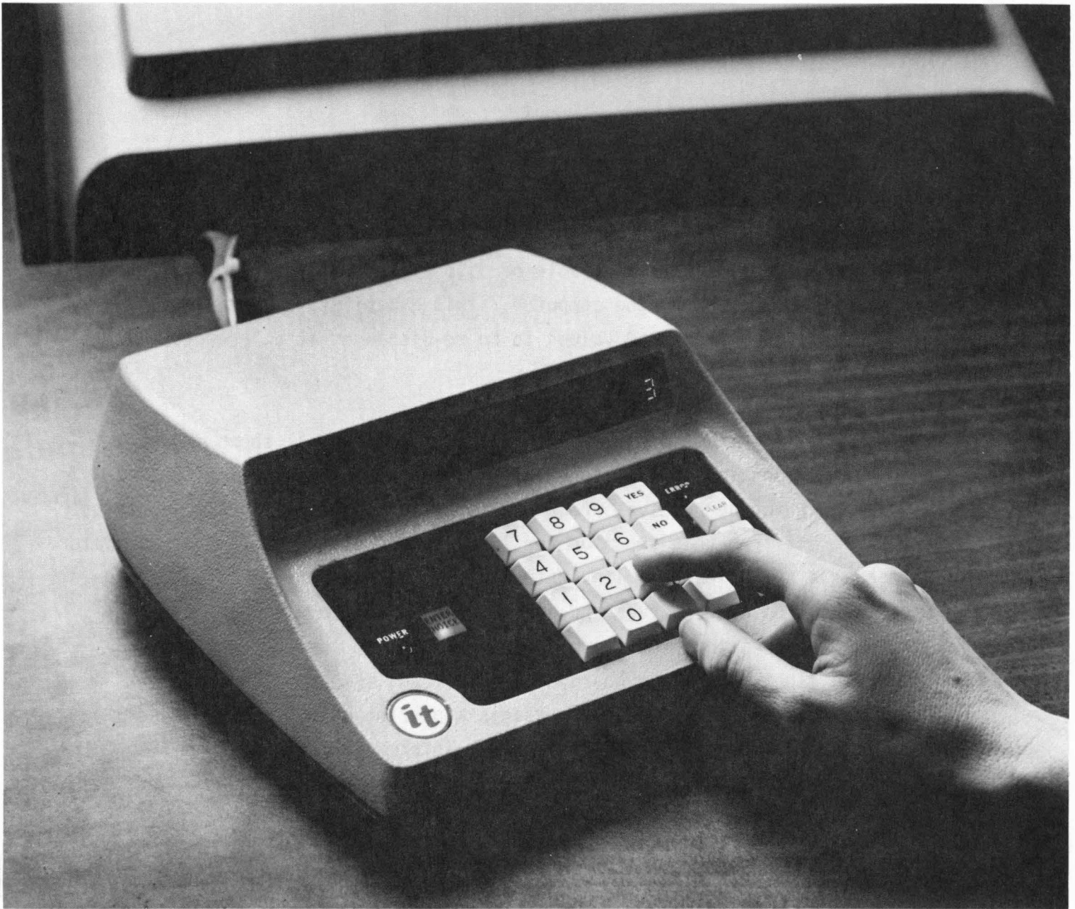
FIGURE 2-2. A PARTICIPANT TERMINAL, SHOWING THE DESIGNATOR SIGNAL (ENTER CHOICE) AND LED FEEDBACK DISPLAY (3).
