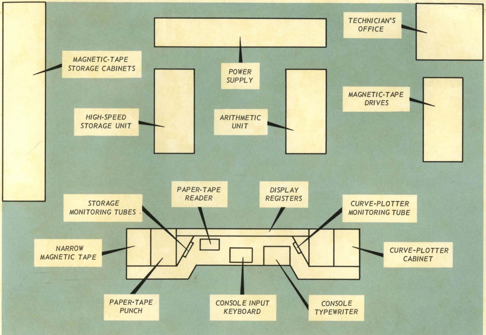
Floor plan of the computer room, showing the location of primary Oracle components. Paper tape preparation and printing machines are in an adjoining room.
