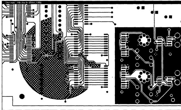
The circular copper pour has a cross-hatch pattern with the hatch grid of 50 at a 45 degree rotation.
