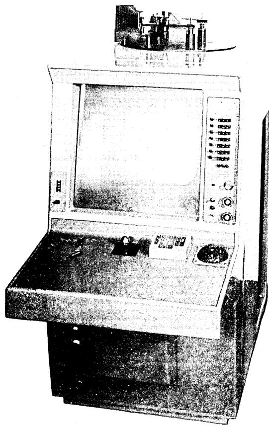
Figure 3 - Ballistic Film Analyzer and Recorder
