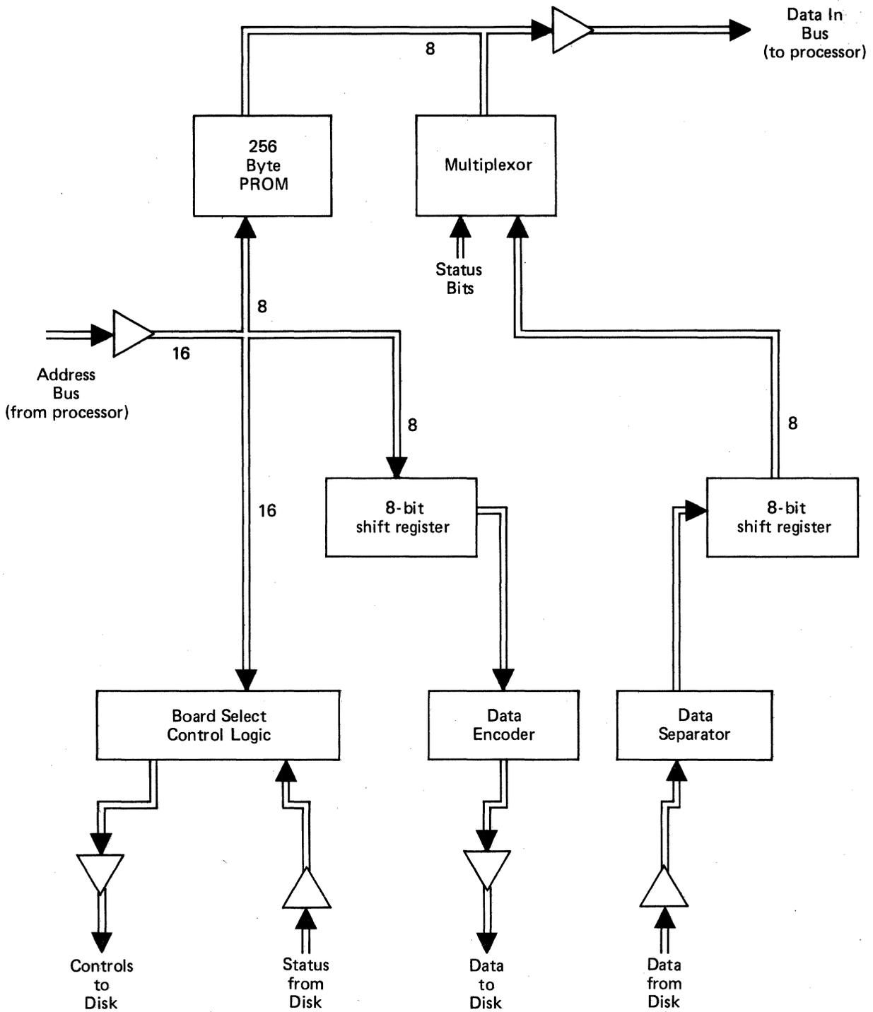
Figure 1T. Disk Controller Block Diagram
