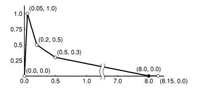
Figure 3-11. Simulated Piano Envelope
