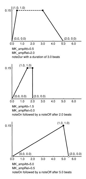
Figure 3-8. Envelope with Attack and Release
