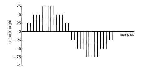
Figure 2-3. Three-Bit Quantization
