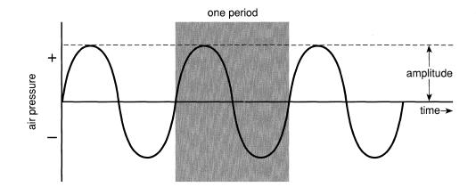
Figure 2-1. Air Pressure Wave
