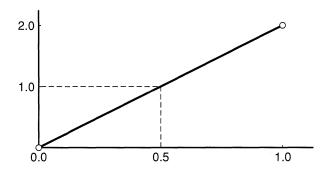
Figure 3-13. Linear Interpolation
