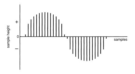
Figure 2-2. Sampled Waveform
