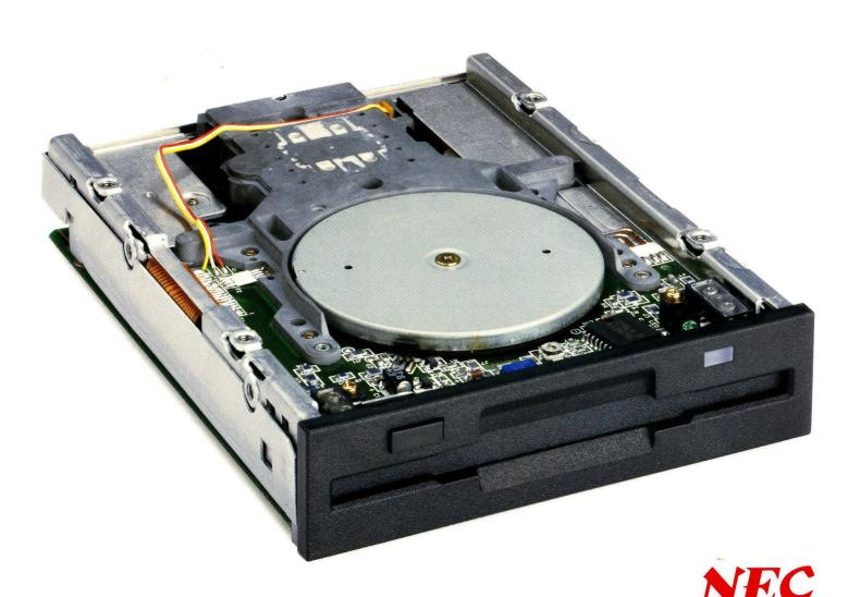
NEC's FD1335H offers 10 MB of formatted storage on a single 3 ½-inch diskette. The FD1335H solves storage problems for applications such as desktop publishing, image processing, computer-aided design, and software distribution.
