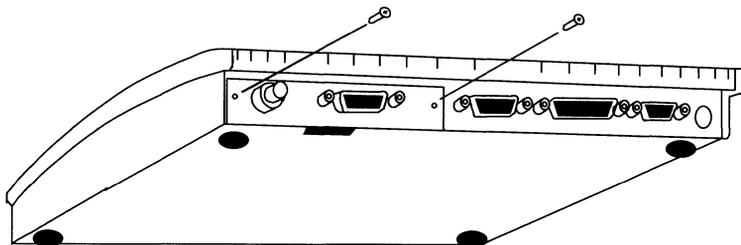
*Figure 2-6. Removing the Communications Interface Module Screws*
