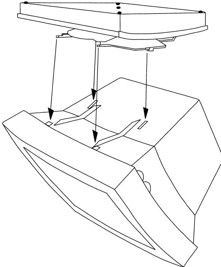
*Figure 2-14. Base Unit/Display Monitor Tab and Tab Socket Locations*
