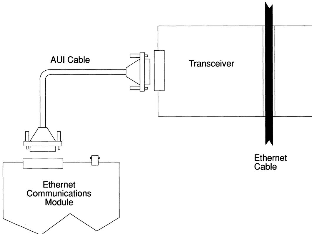
*Figure 2-18. Connecting a Transceiver to the NCD16*
