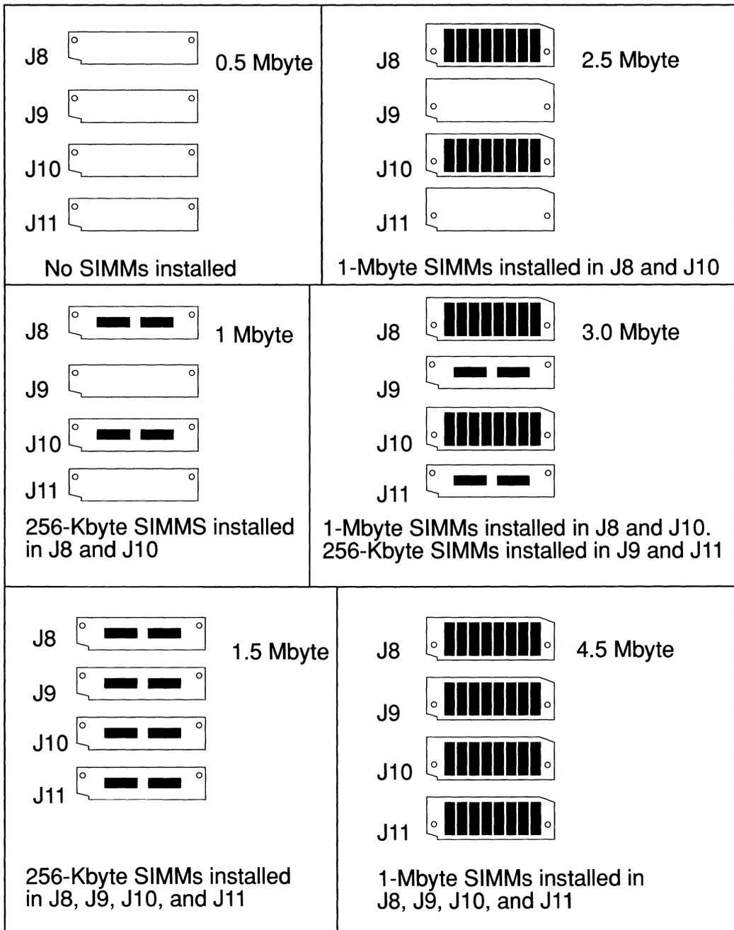
Figure 2-12. Allowable SIMM Configurations
