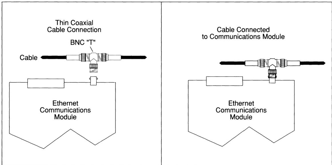
Figure 2-18. Thin Cable Ethernet Connection
