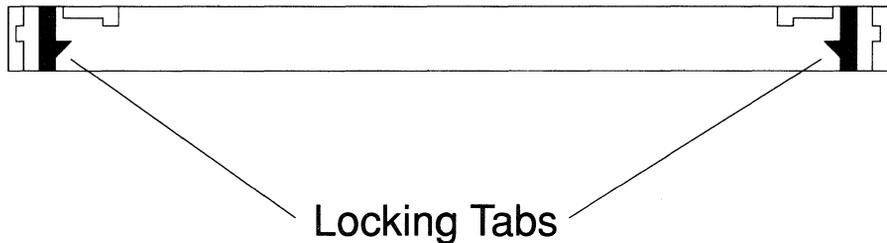
*Figure 2-11. SIMM Socket Locking Tabs*
