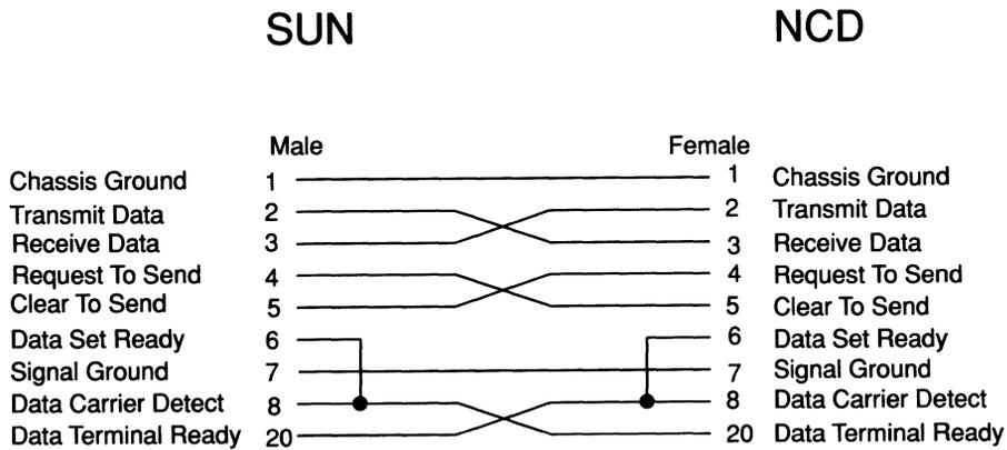
*Figure A-2. Sun-to-NCD Serial Cable Pinouts*
