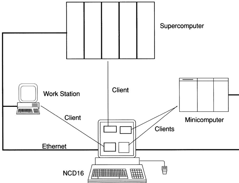
*Figure 3-1. NCD16 Using X Window System Over a Network*
