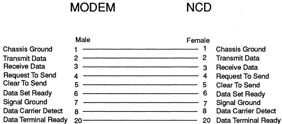
*Figure A-1. Modem-to-NCD Serial Cable Pinouts*
