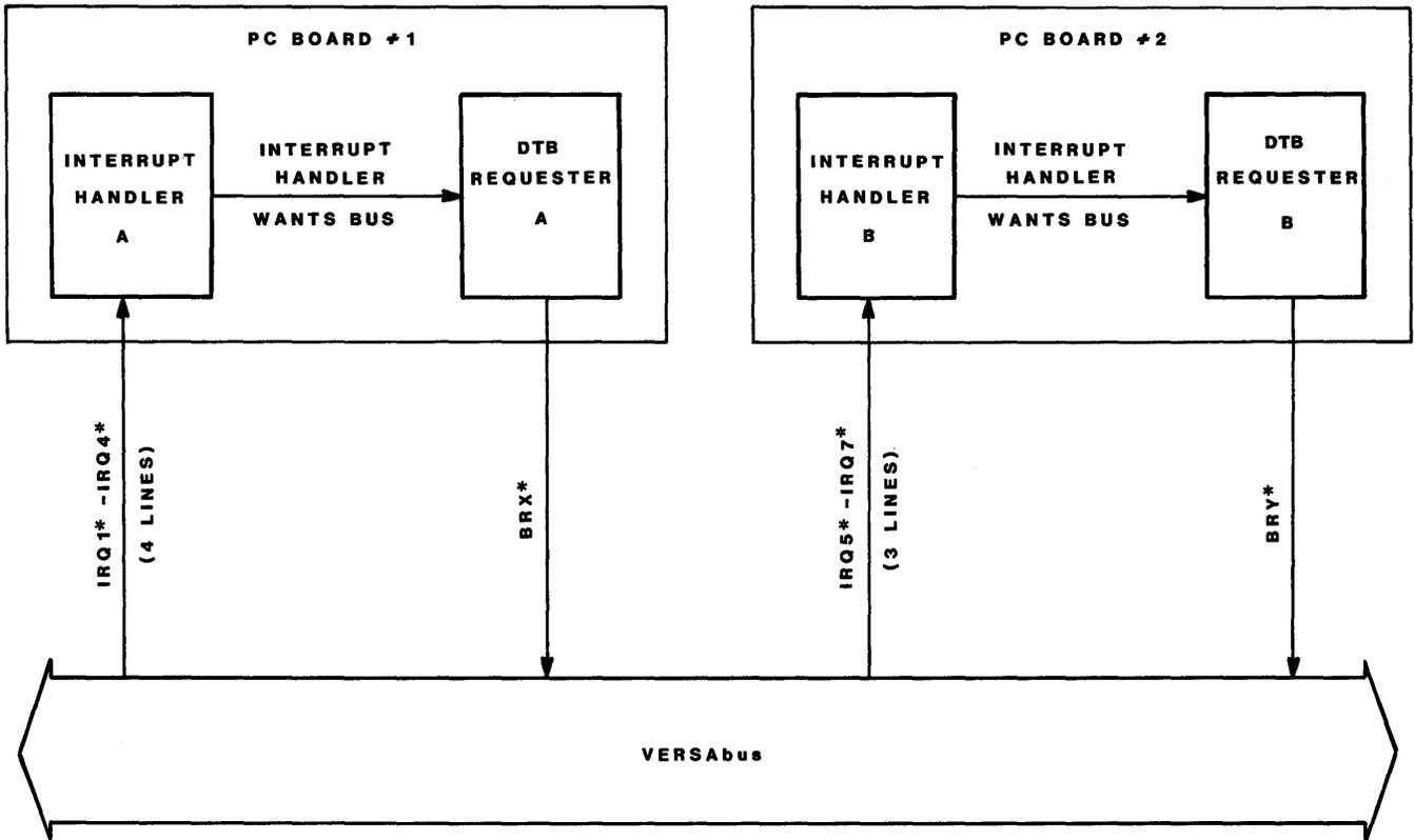
FIGURE 4-9. Two INTERRUPT HANDLERS, Each Monitoring Several Interrupt Request Lines
