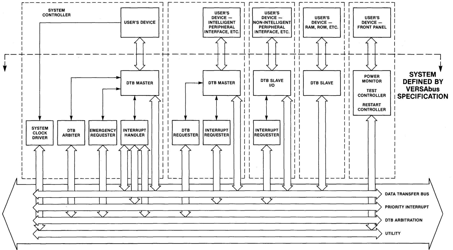
FIGURE 1-3. Functional Modules and Buses contained within the VERSAbus Definition
