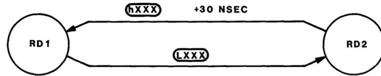
THE STATES SHOWN IN THE DIAGRAM ABOVE DON'T RESULT IN ANY OUTPUT CHANGES. (THEY REPRESENT THE STATE OF AN INTERNAL MONOSTABLE FLIP-FLOP.) THEY ARE LABELLED SIMPLY "REQUESTER DELAY STATES 1 AND 2."
