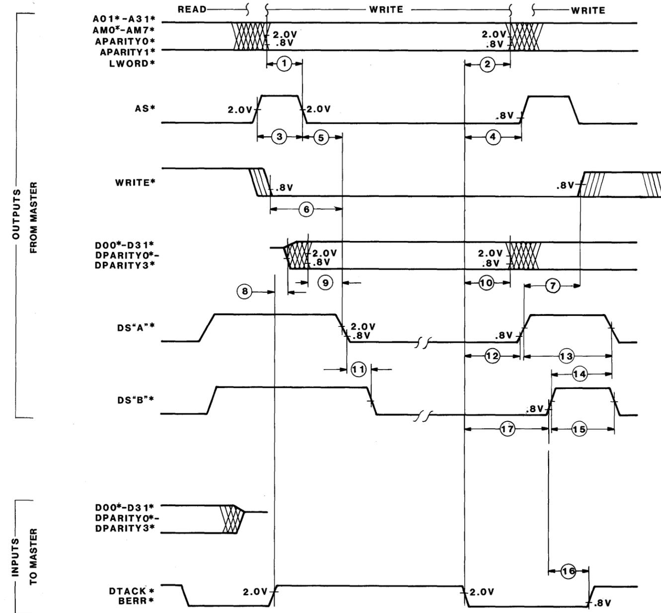
FIGURE 2-14. DTB MASTER Timing: Read Cycle Followed by Write Cycle
