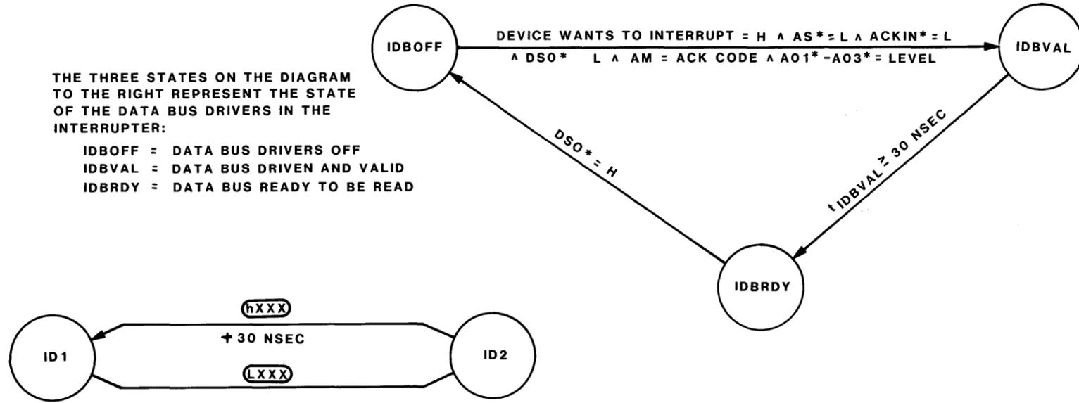
THE STATES SHOWN IN THE DIAGRAM ABOVE DON'T RESULT IN ANY OUTPUT CHANGES. (THEY REPRESENT THE STATE OF AN INTERNAL MONOSTABLE FLIP-FLOP.) THEY ARE LABELLED SIMPLY "INTERRUPTER DELAY STATES 1 AND 2"
