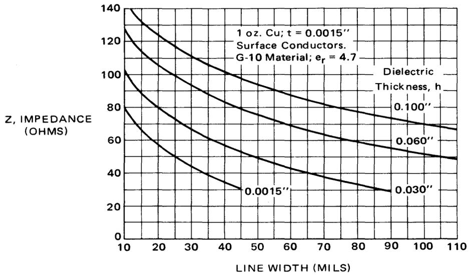
FIGURE 7-4. Impedance versus Line Width and Dielectric Thickness for Microstrip Lines
