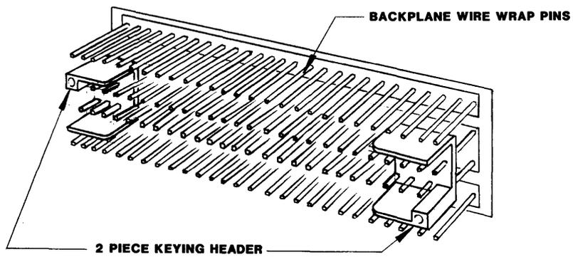
FIGURE 8-8. Single Cable Method Keying Header Configuration
