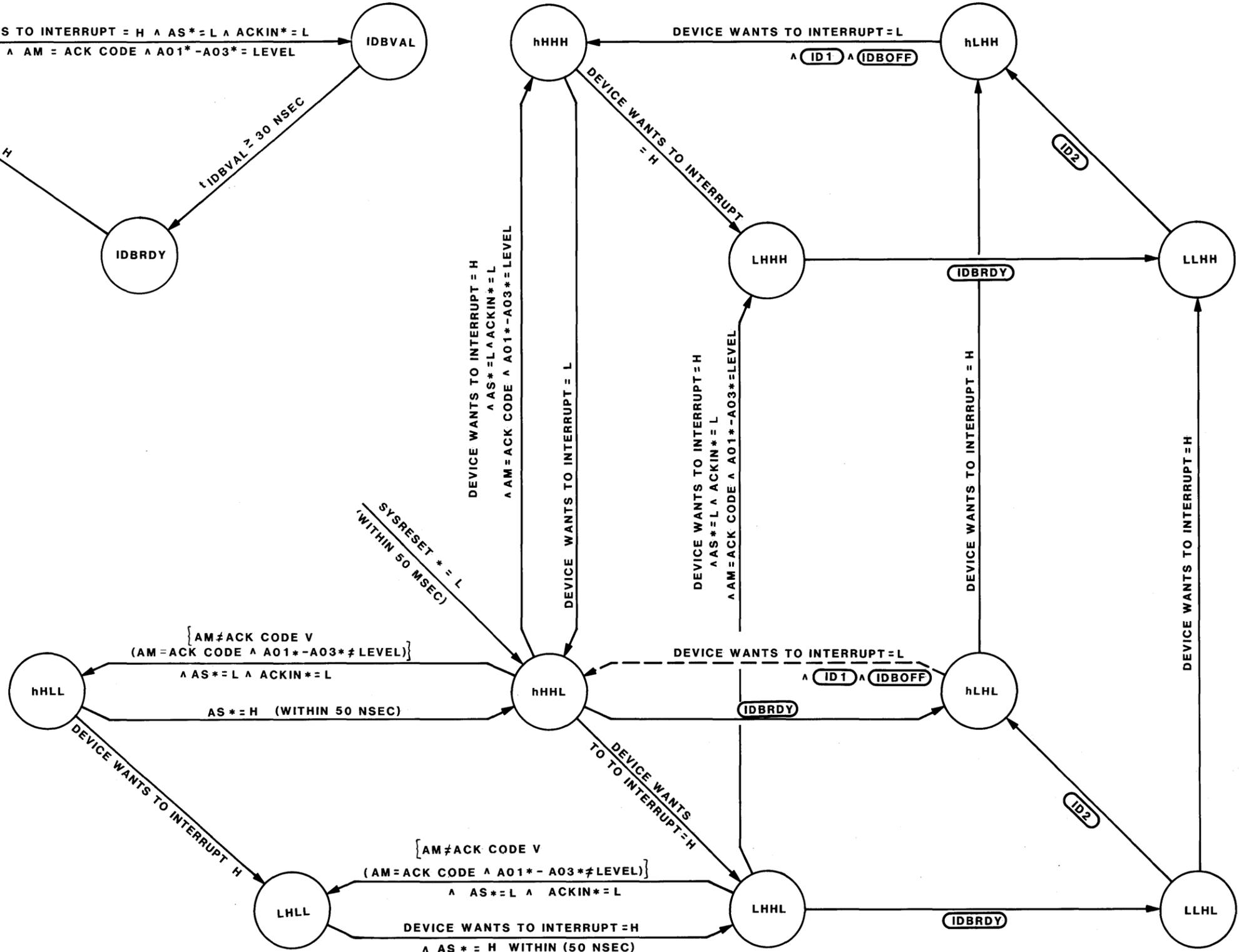
FIGURE 4-12. INTERRUPTER State Diagram
