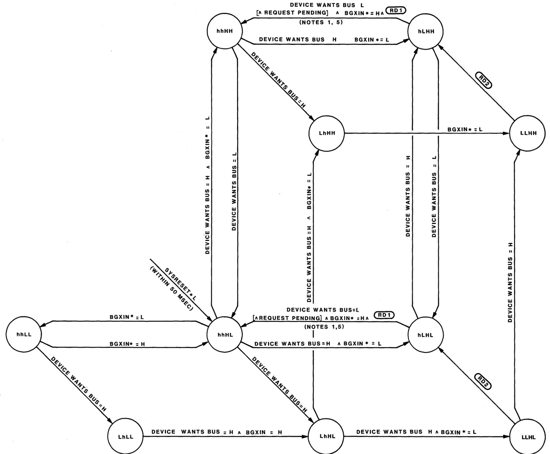
FIGURE 3-15. DTB REQUESTER State Diagram
