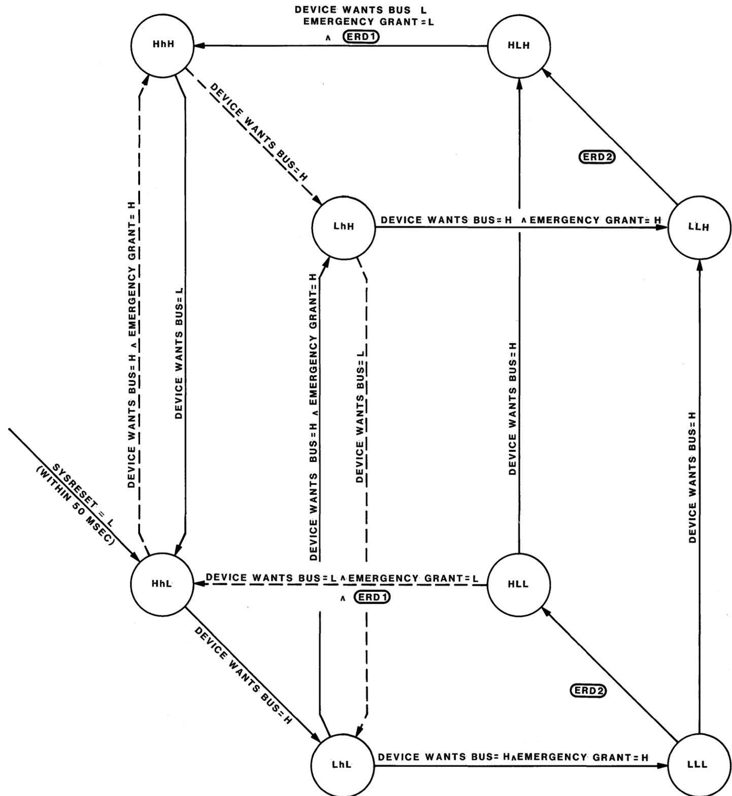
FIGURE 3-18. EMERGENCY REQUESTER State Diagram
