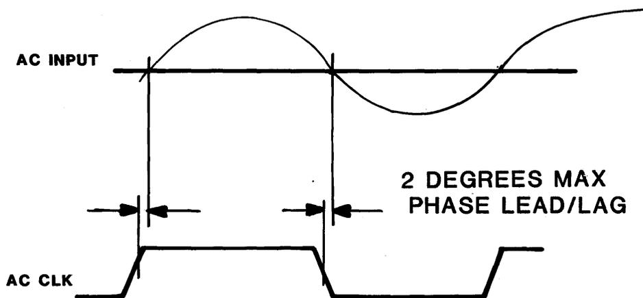
FIGURE 5-3. AC Clock Timing Diagram
