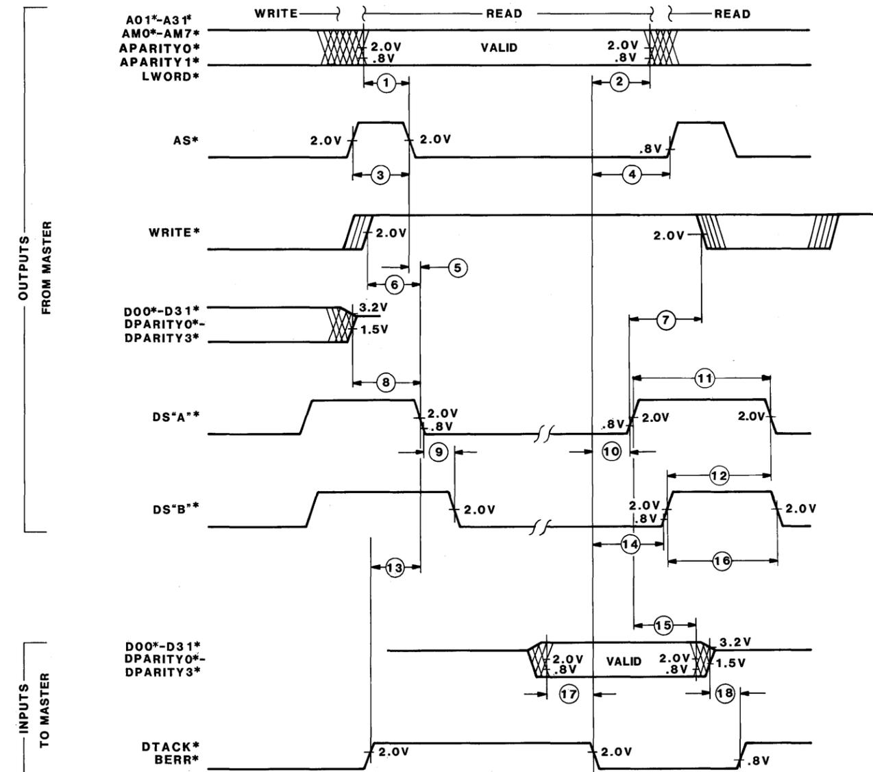
FIGURE 2-13. DTB MASTER Timing: Write Cycle Followed by Read Cycle
