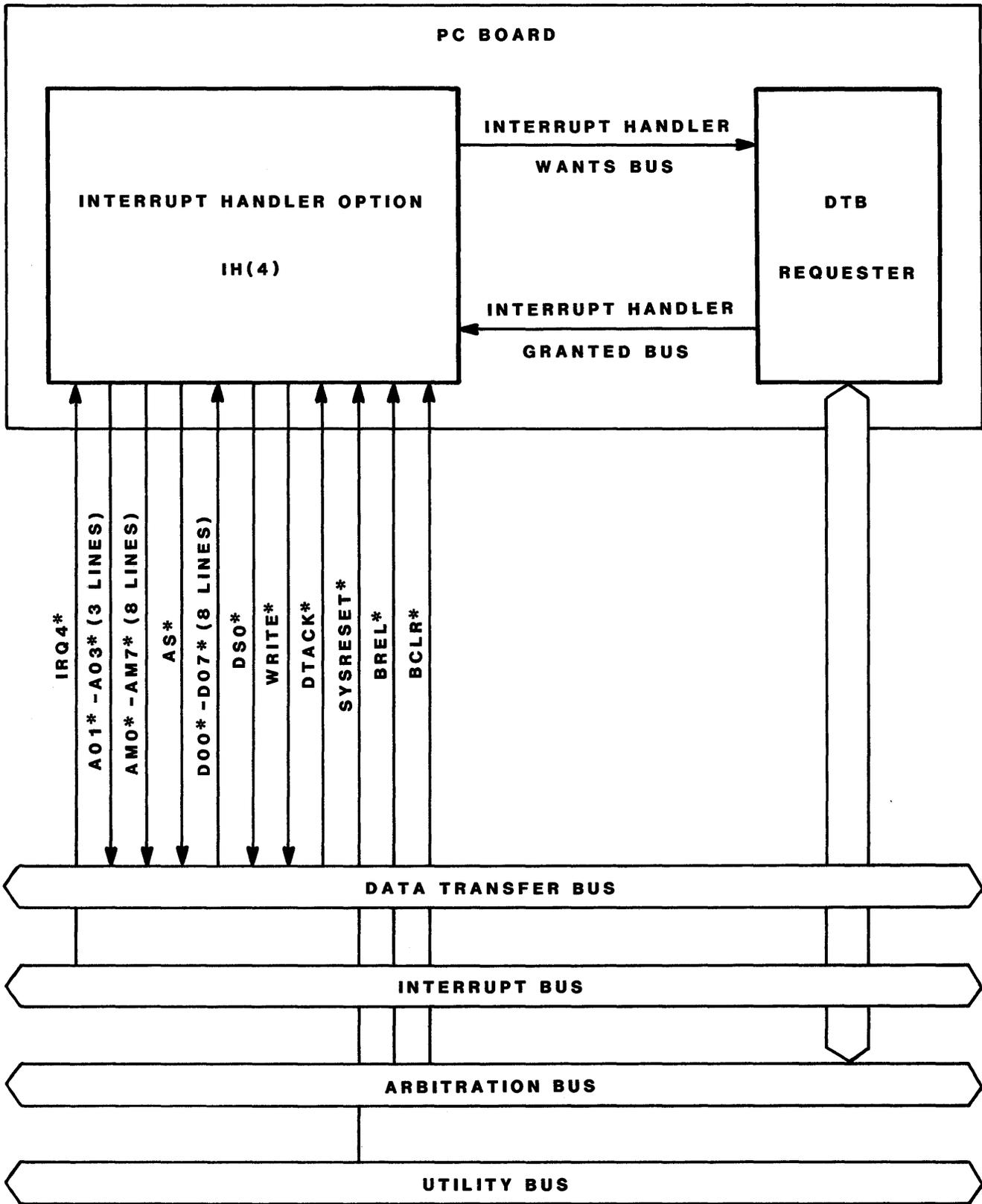
FIGURE 4-7. INTERRUPT HANDLER Monitoring Only IRQ4\*
