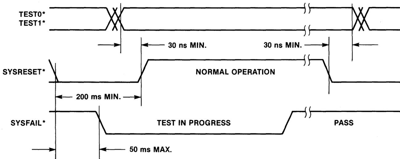
FIGURE 5-4. System Reset and Test Timing Diagram
