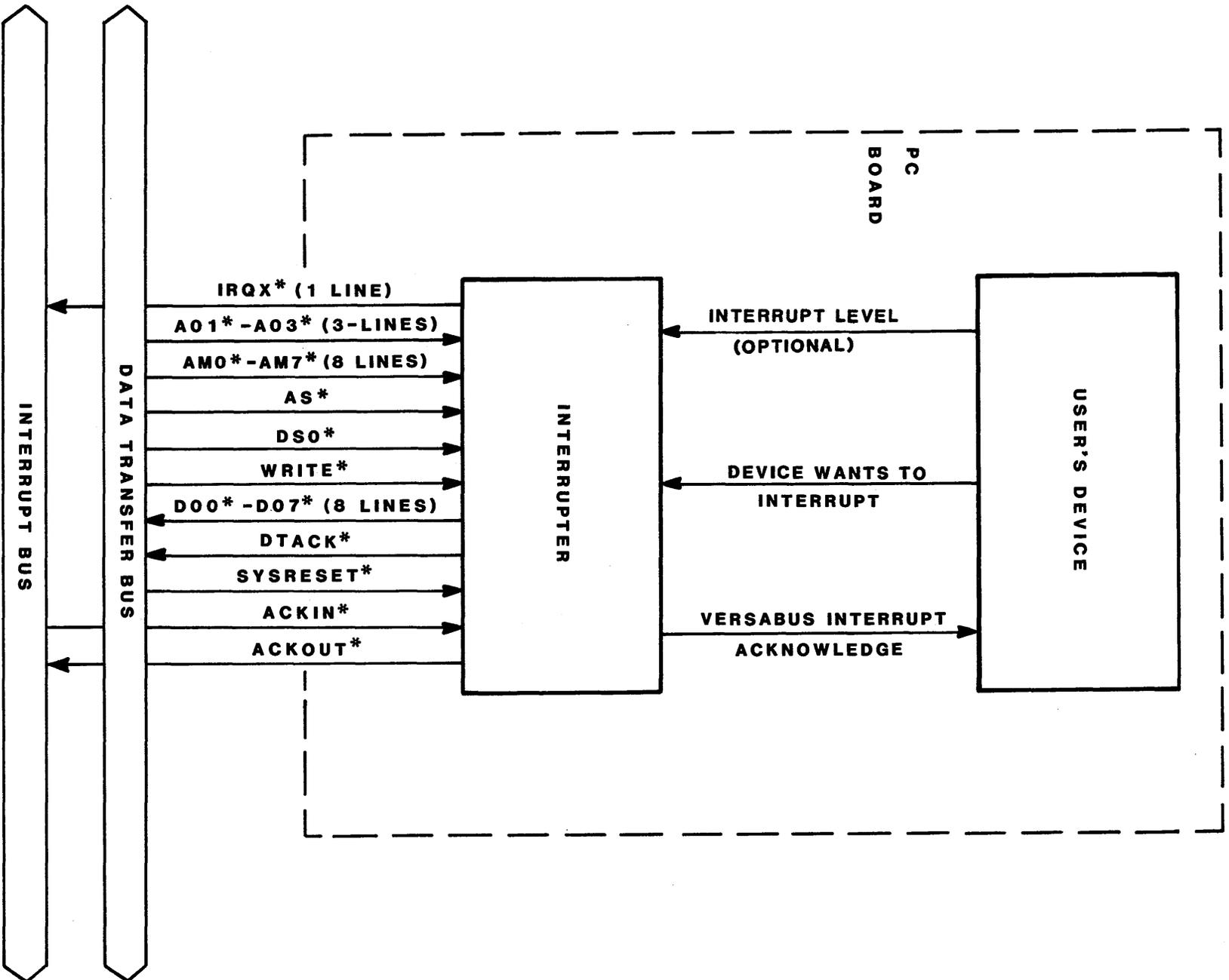
FIGURE 4-13. INTERRUPTER Block Diagram
