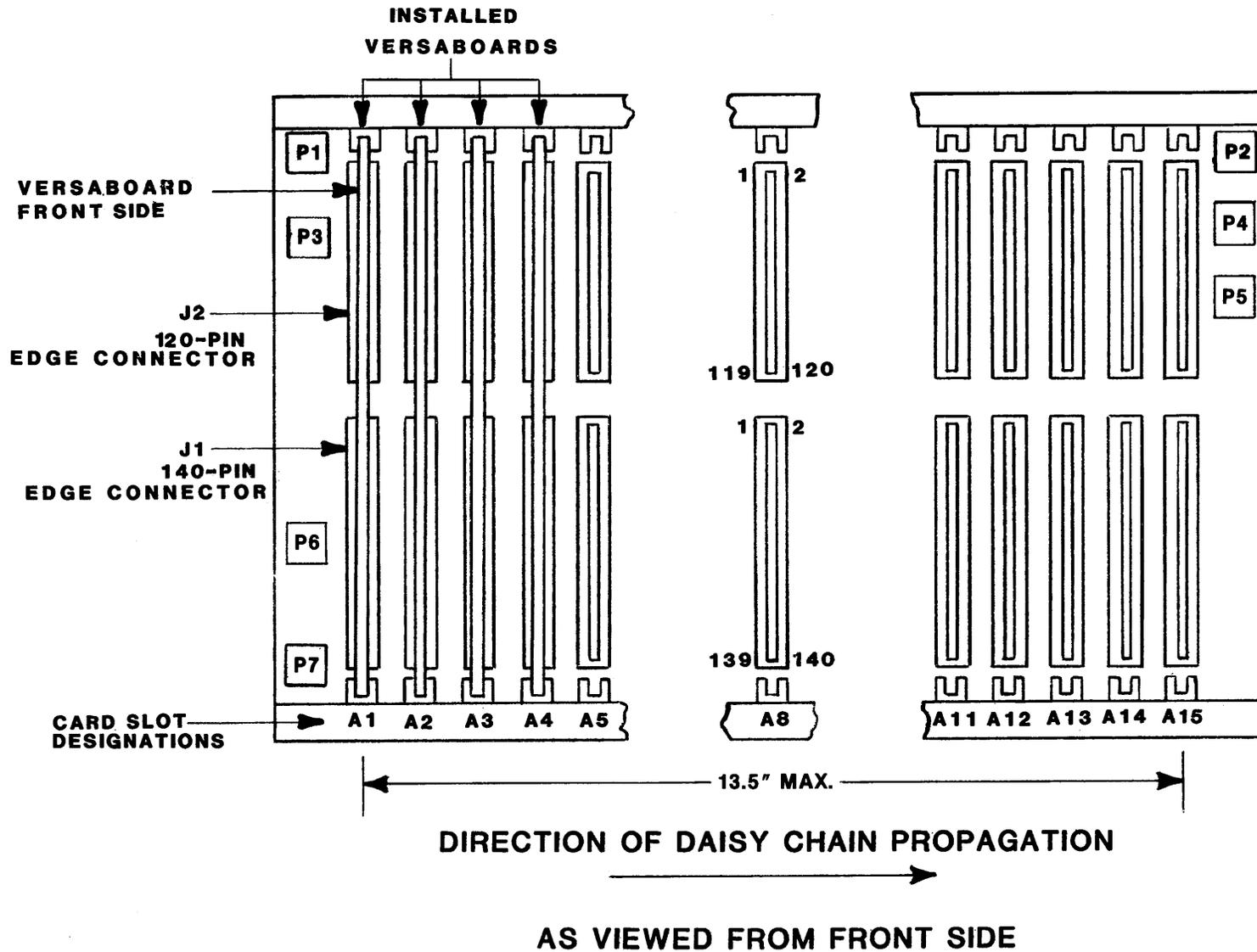
FIGURE 8-3. Backplane Reference Designations and Pin Numbering Standard
