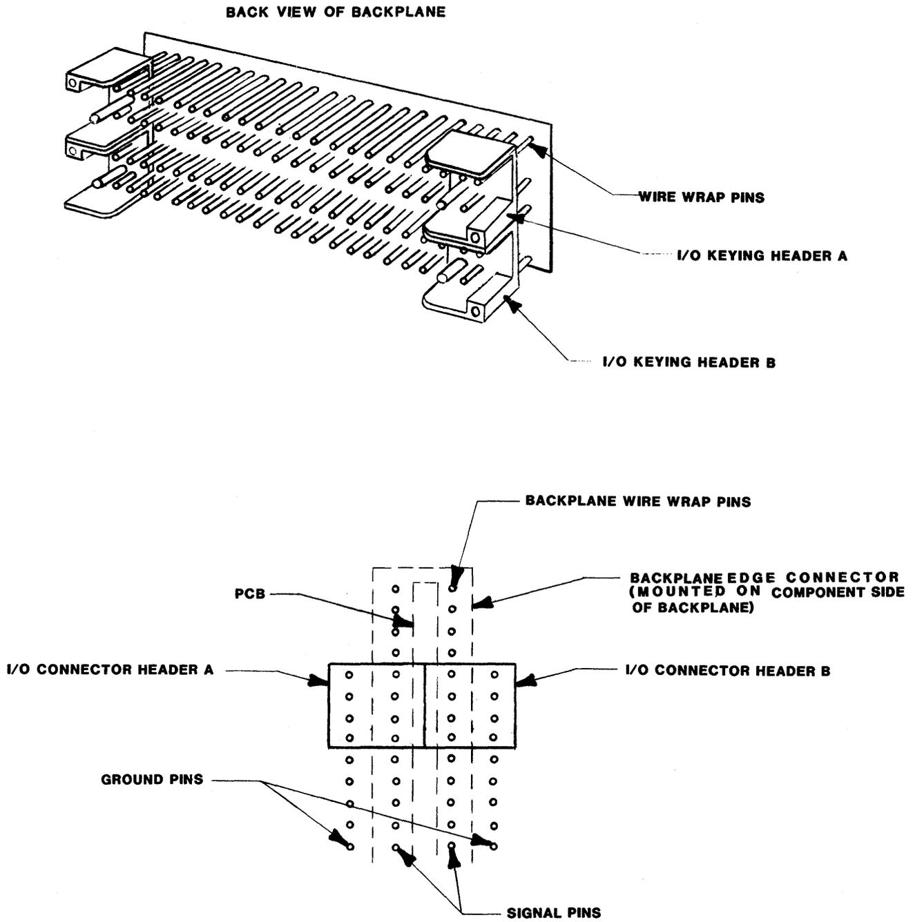
FIGURE 8-9. Dual Cable Method Keying Header Configuration
