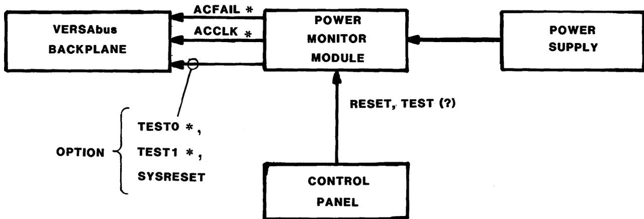
FIGURE 5-5. Block Diagram of POWER MONITOR Module
