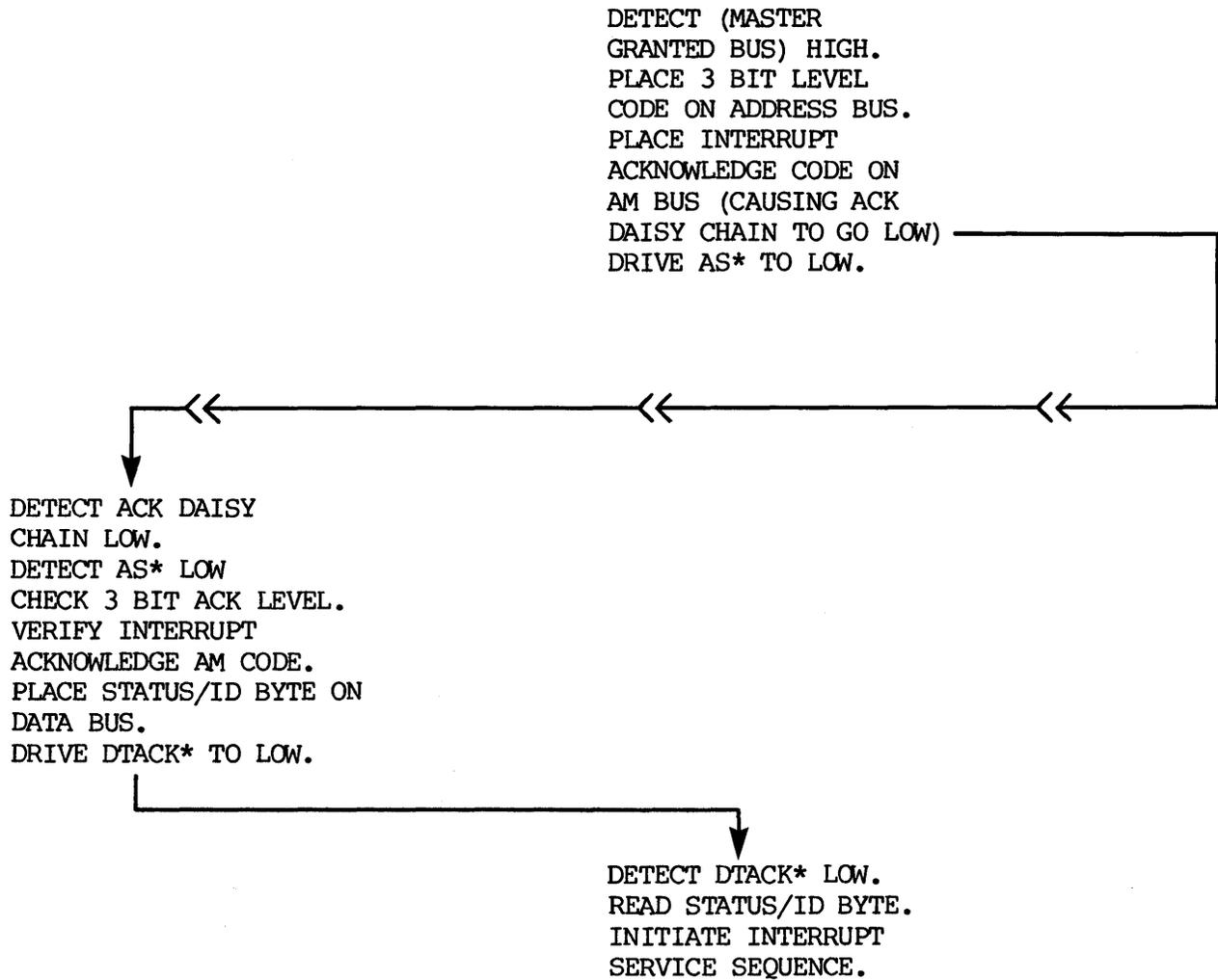
FIGURE 4-10. Typical Single Handler Interrupt System Operation Flow Diagram (Sheet 2 of 2)
