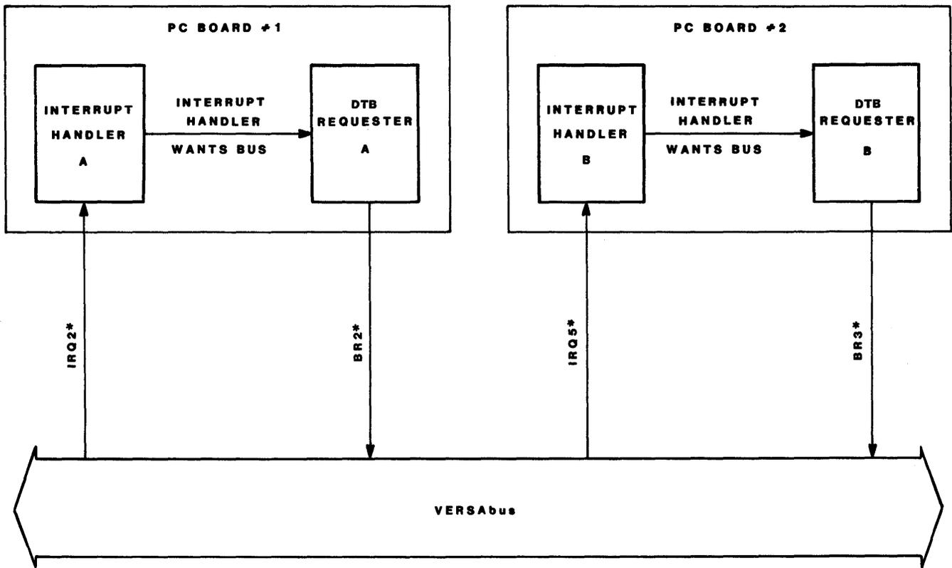
FIGURE 4-8. Two INTERRUPT HANDLERS, Each Monitoring One Interrupt Request Line
