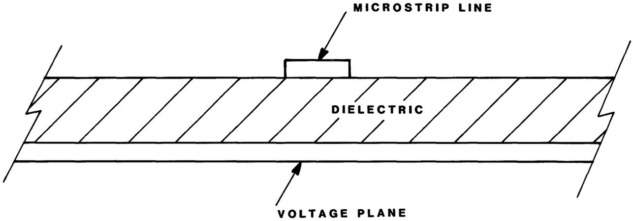
FIGURE 7-3. Backplane Microstrip Signal Line Cross Section
