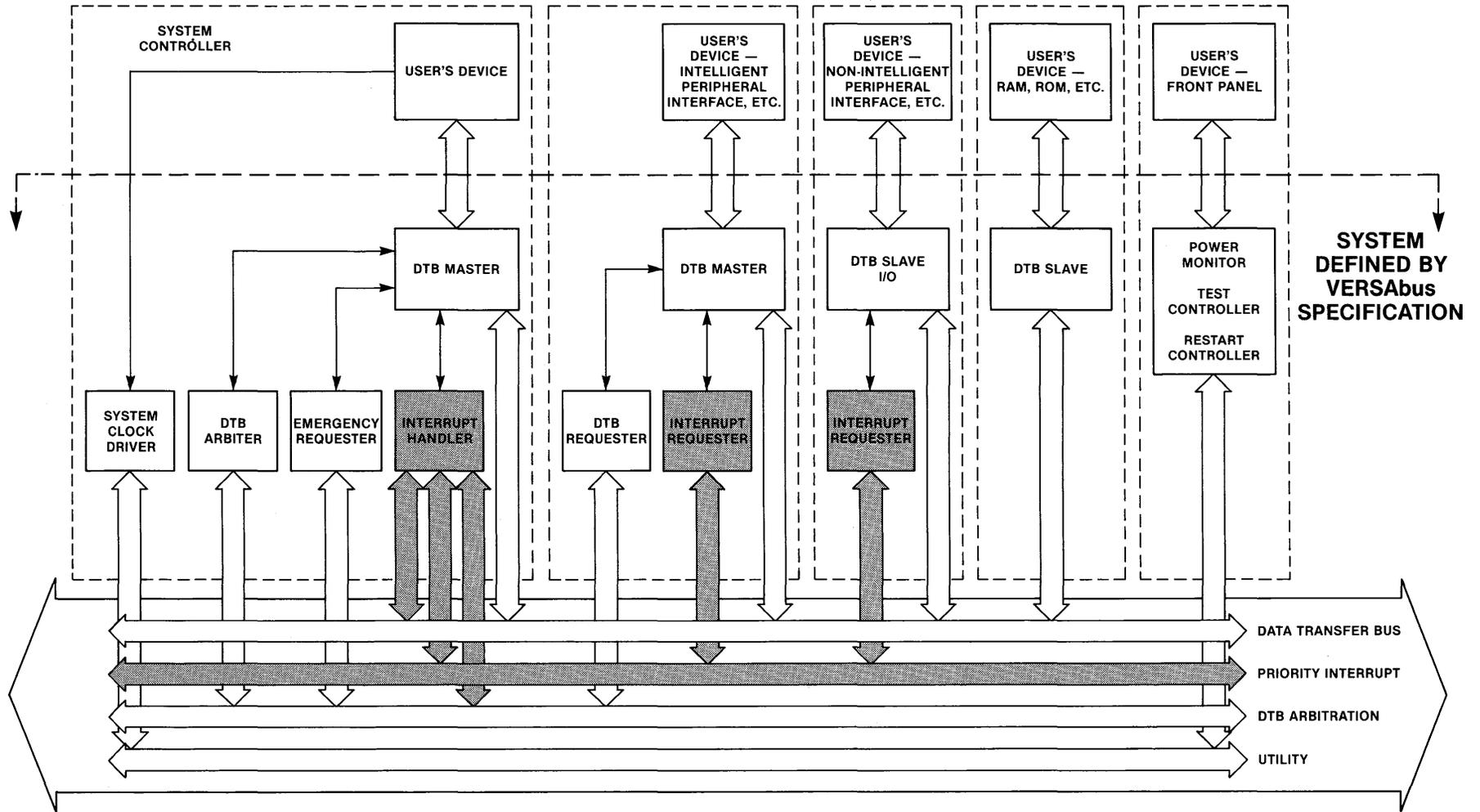
FIGURE 4-3. VERSAbus Priority Interrupt Functional Block Diagram
