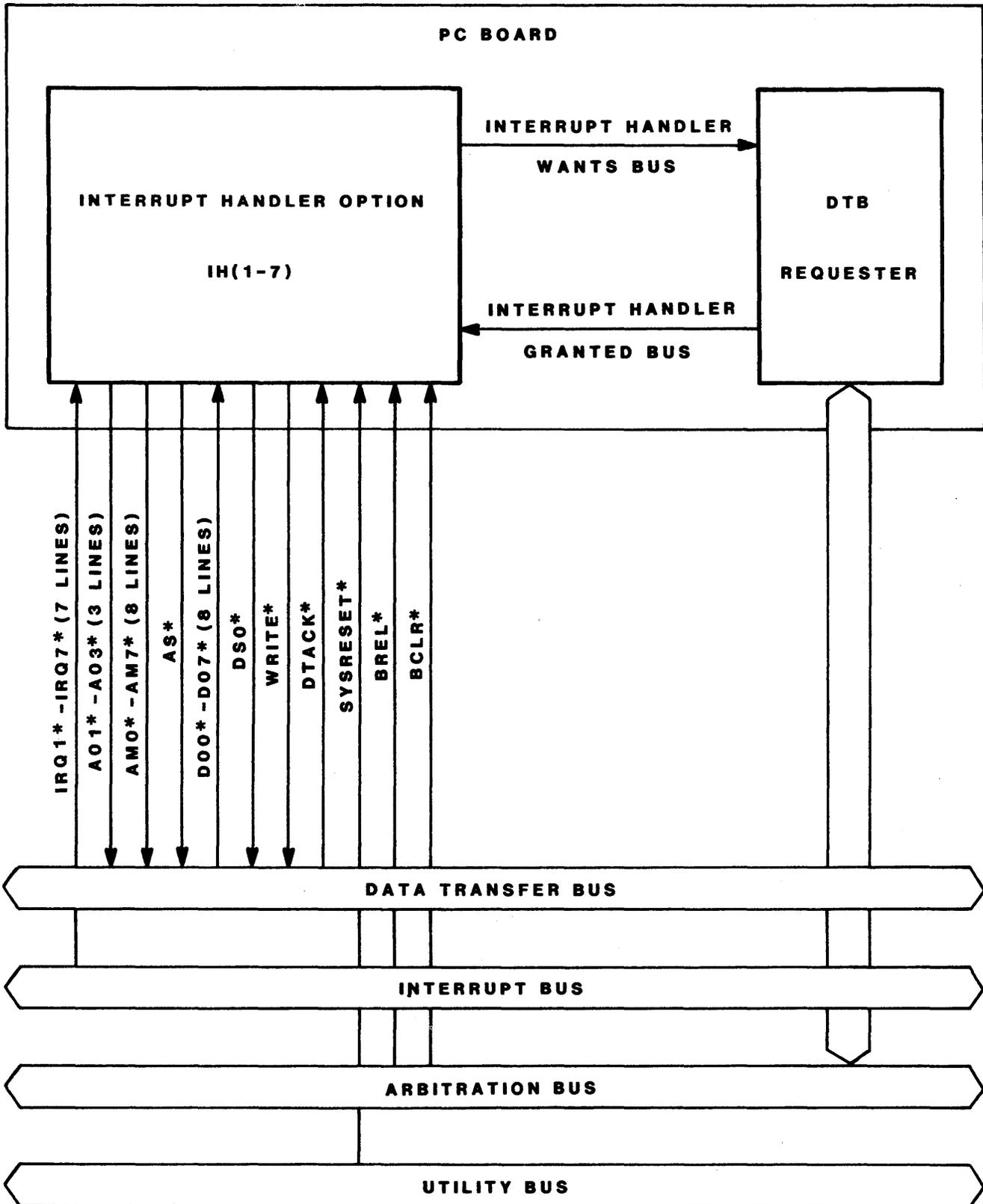
FIGURE 4-4. Signal Lines Used by an IH(1-7) INTERRUPT HANDLER
