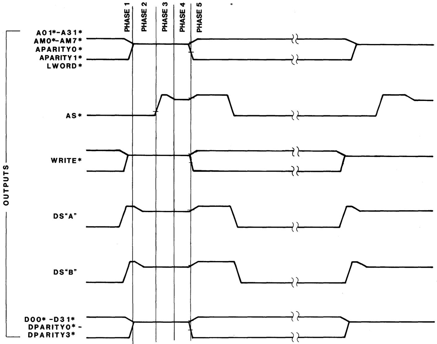
FIGURE 2-15. MASTER Timing: Control Transfers of DTB
