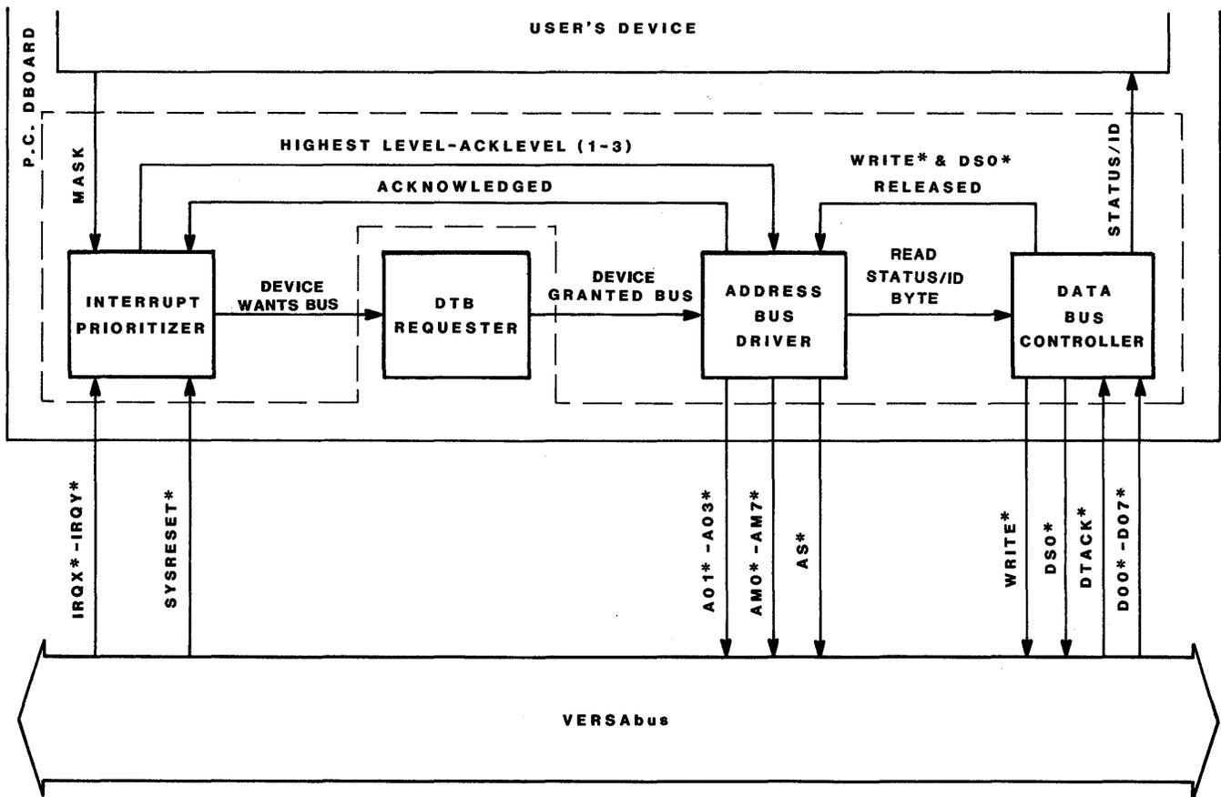
FIGURE 4-14. Block Diagram: INTERRUPT HANDLER
