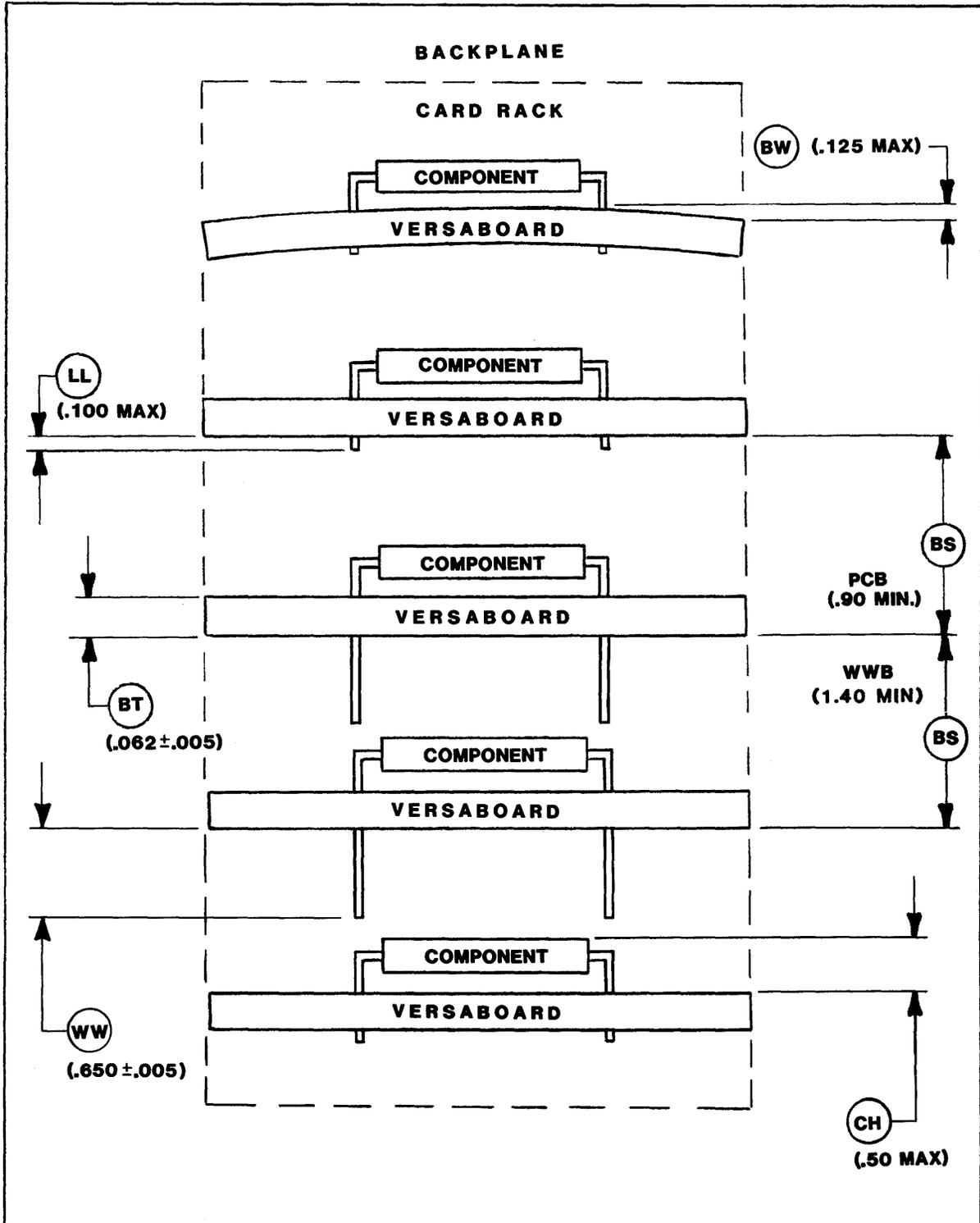
FIGURE 8-4. Backplane/VERSABOARD Dimensional Requirements
