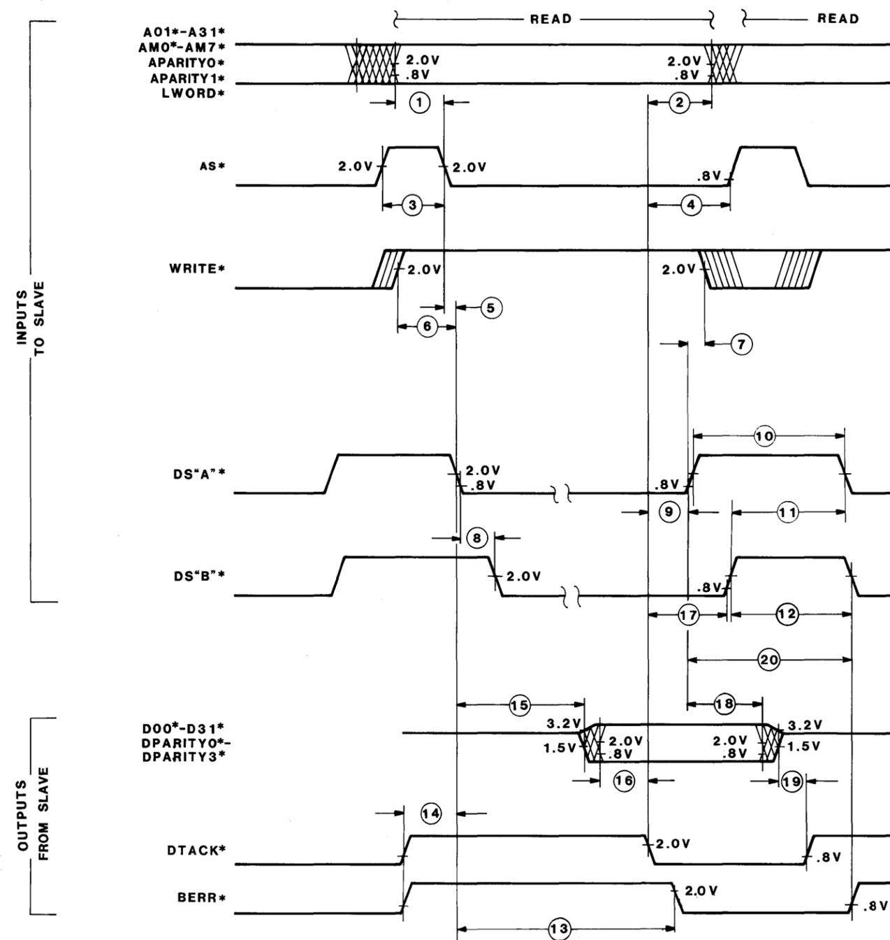
FIGURE 2-16. Data Transfer Bus SLAVE Read Cycle
