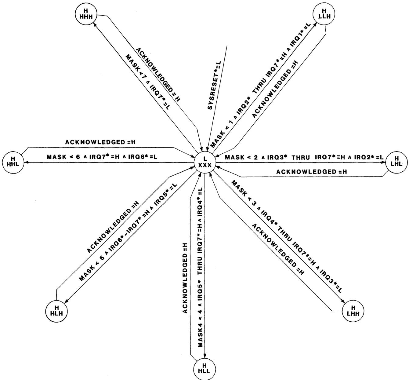
THE STATES ON THIS DIAGRAM ARE LABELLED ACCORDING TO THE LEVELS OF THE INTERRUPT PRIORITIZERS OUTPUT LINES.
