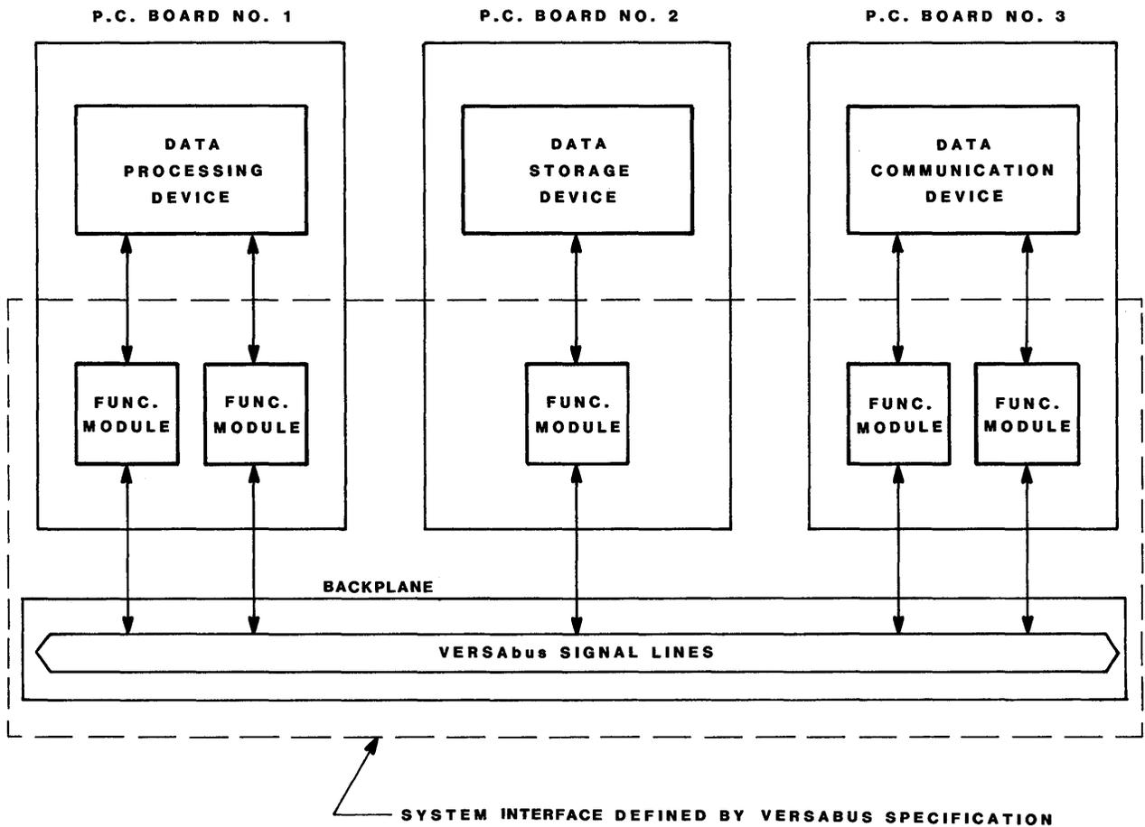
FIGURE 1-2. System Elements Defined by the VERSAbus Specification
