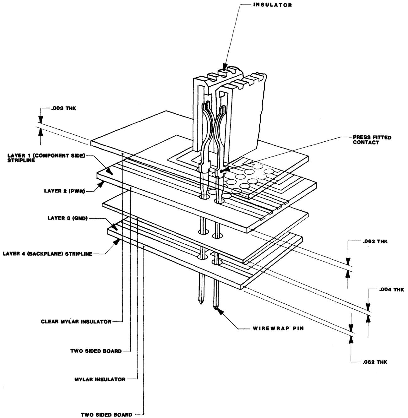
FIGURE 8-1. Typical Multilayer Backplane/PCB Construction Technique
