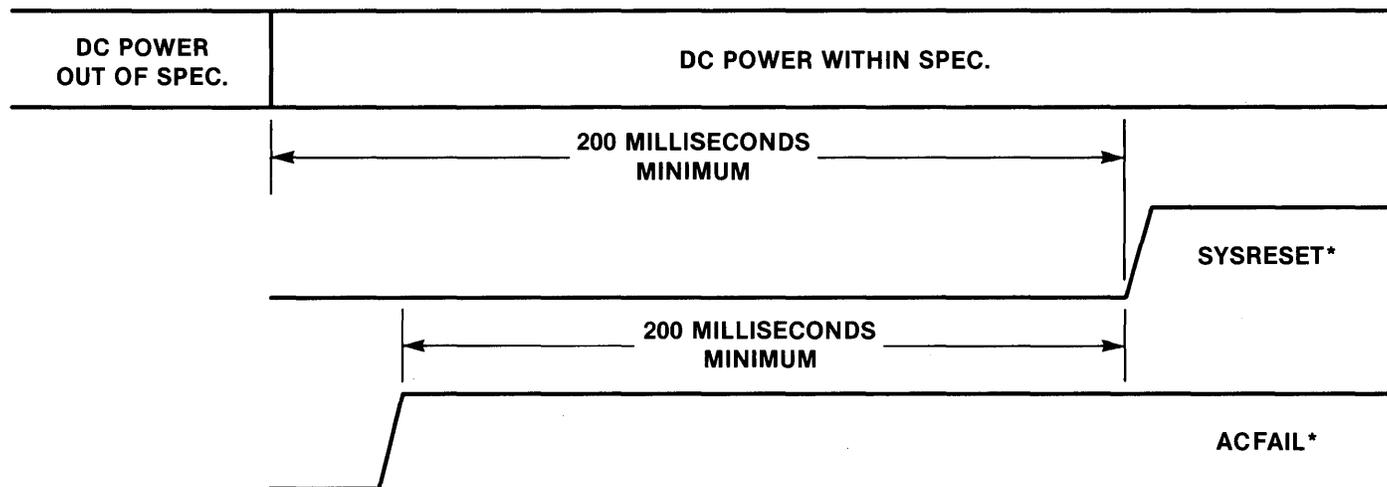
FIGURE 5-7. System Power Restart Timing
