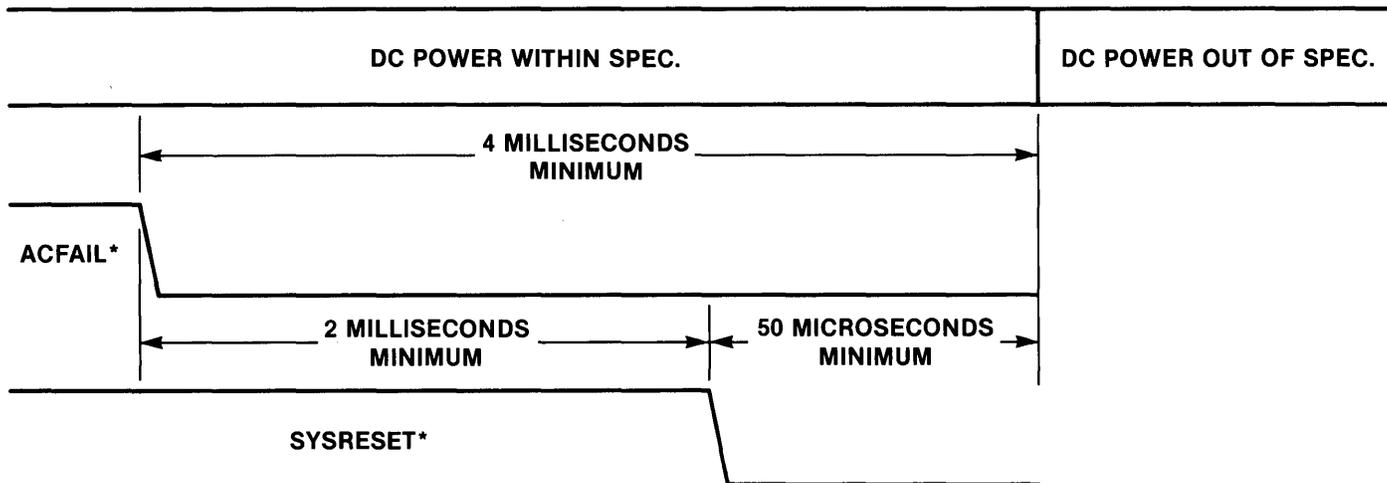
FIGURE 5-6. System Power Fail Timing
