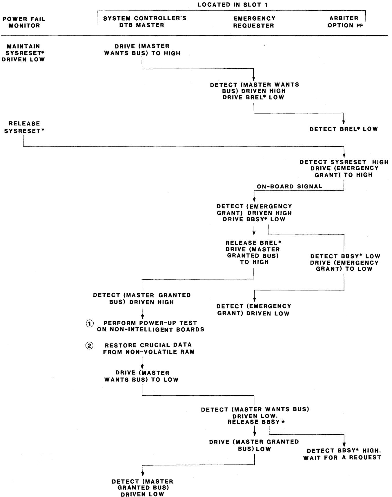
FIGURE 3-13. Power-Up Flow Diagram
