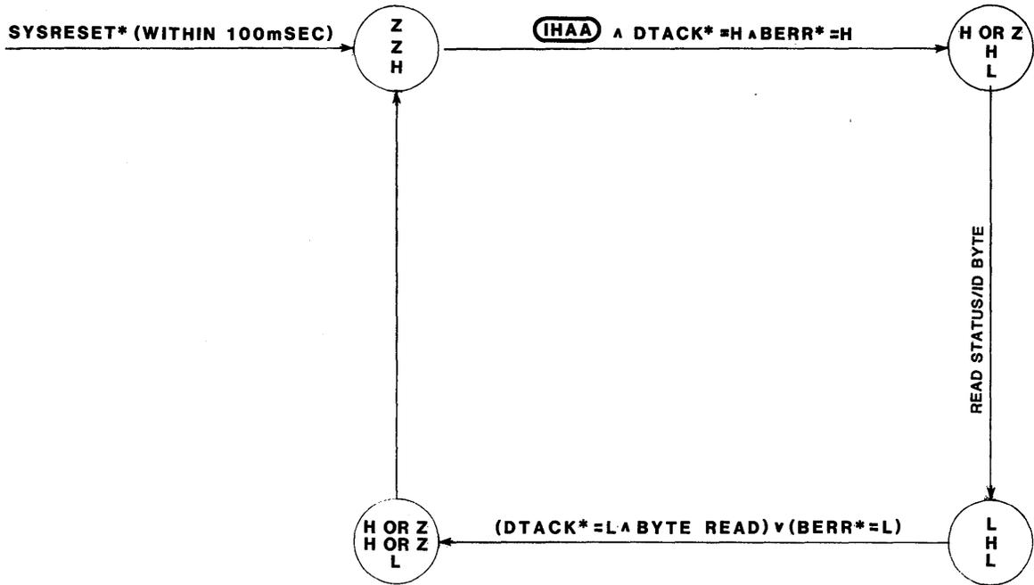
THE STATES IN THIS DIAGRAM ARE LABELLED ACCORDING TO THE LEVELS OF THE INTERRUPT HANDLER'S DATA BUS CONTROLLER OUTPUT LINES.
