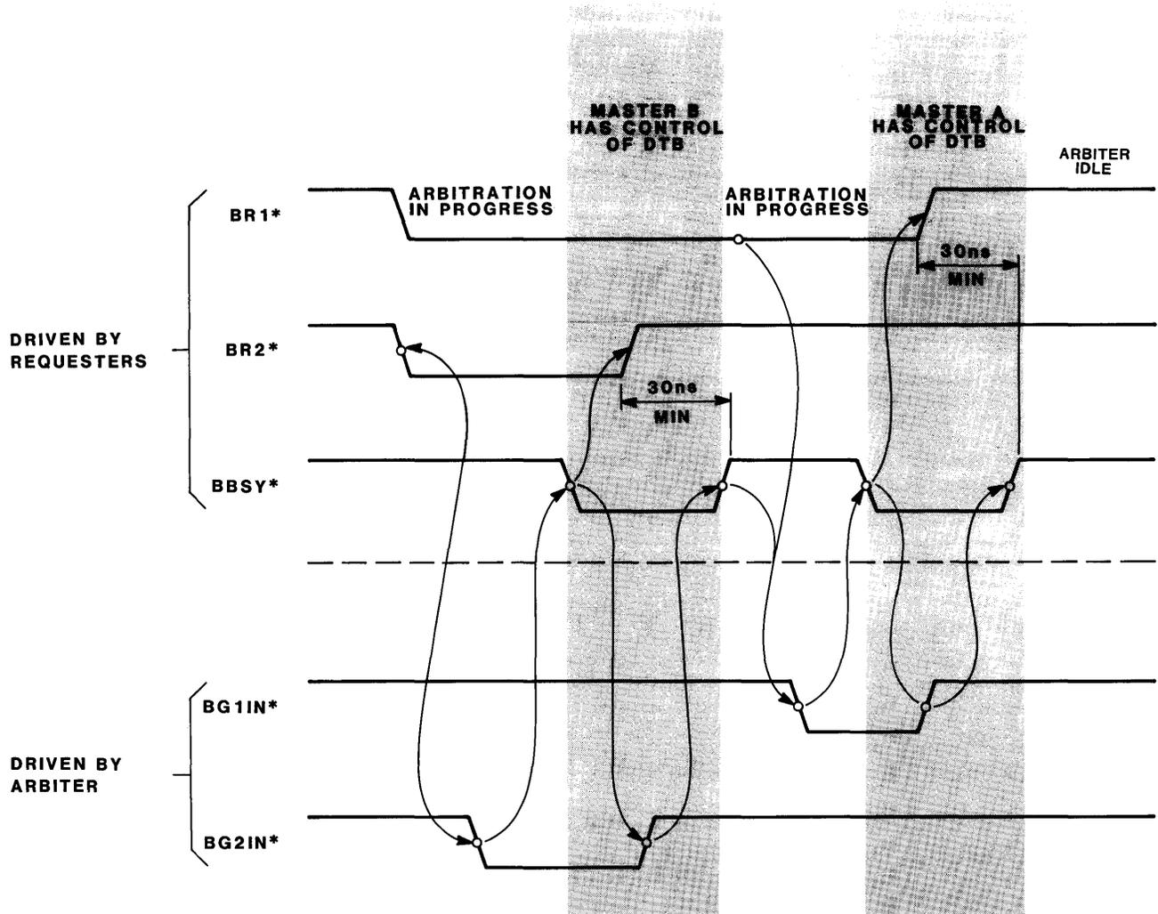
FIGURE 3-8. Arbitration Sequence Diagram: Two REQUESTERS, Two Request Levels
