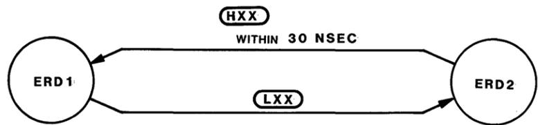
THE STATES SHOWN IN THE DIAGRAM ABOVE DON'T RESULT IN ANY OUTPUT CHANGES. (THEY REPRESENT THE STATE OF AN INTERNAL MONOSTABLE FLIP-FLOP.) THEY ARE LABELLED SIMPLY 'EMERGENCY REQUESTER DELAY STATE 1 AND 2'
