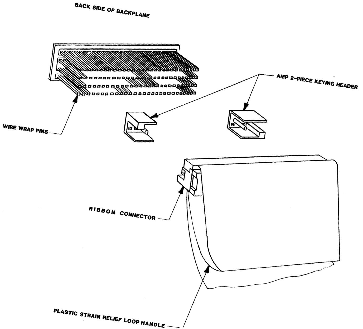
FIGURE 8-6. I/O Cable Connection
