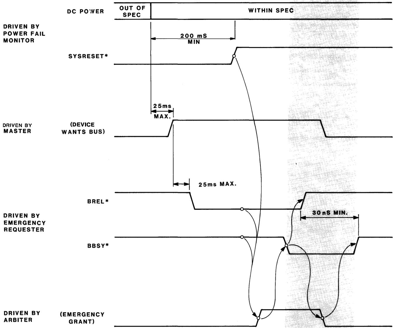
FIGURE 3-14. Power-Up Sequence Diagram
