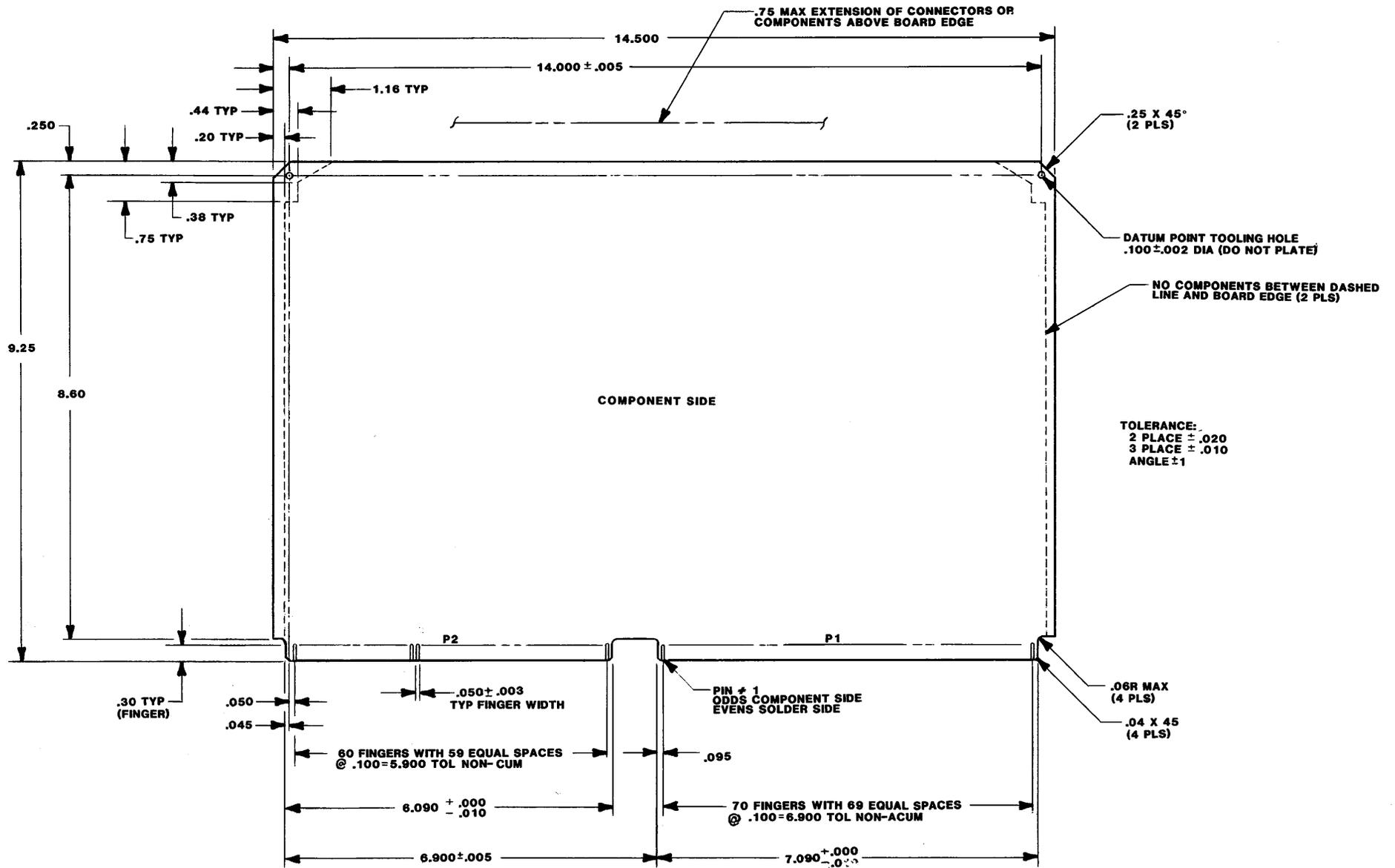
FIGURE 8-11. Standard Size PCB
