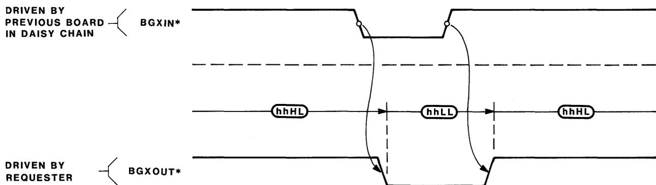
FIGURE 3-17. Sequence Diagram: REQUESTER Drives BGxOUT\*
