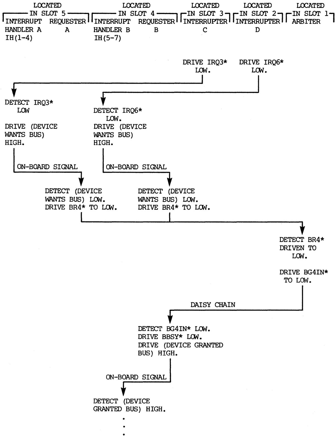
FIGURE 4-11. Distributed Interrupt System with Two INTERRUPT HANDLERS
