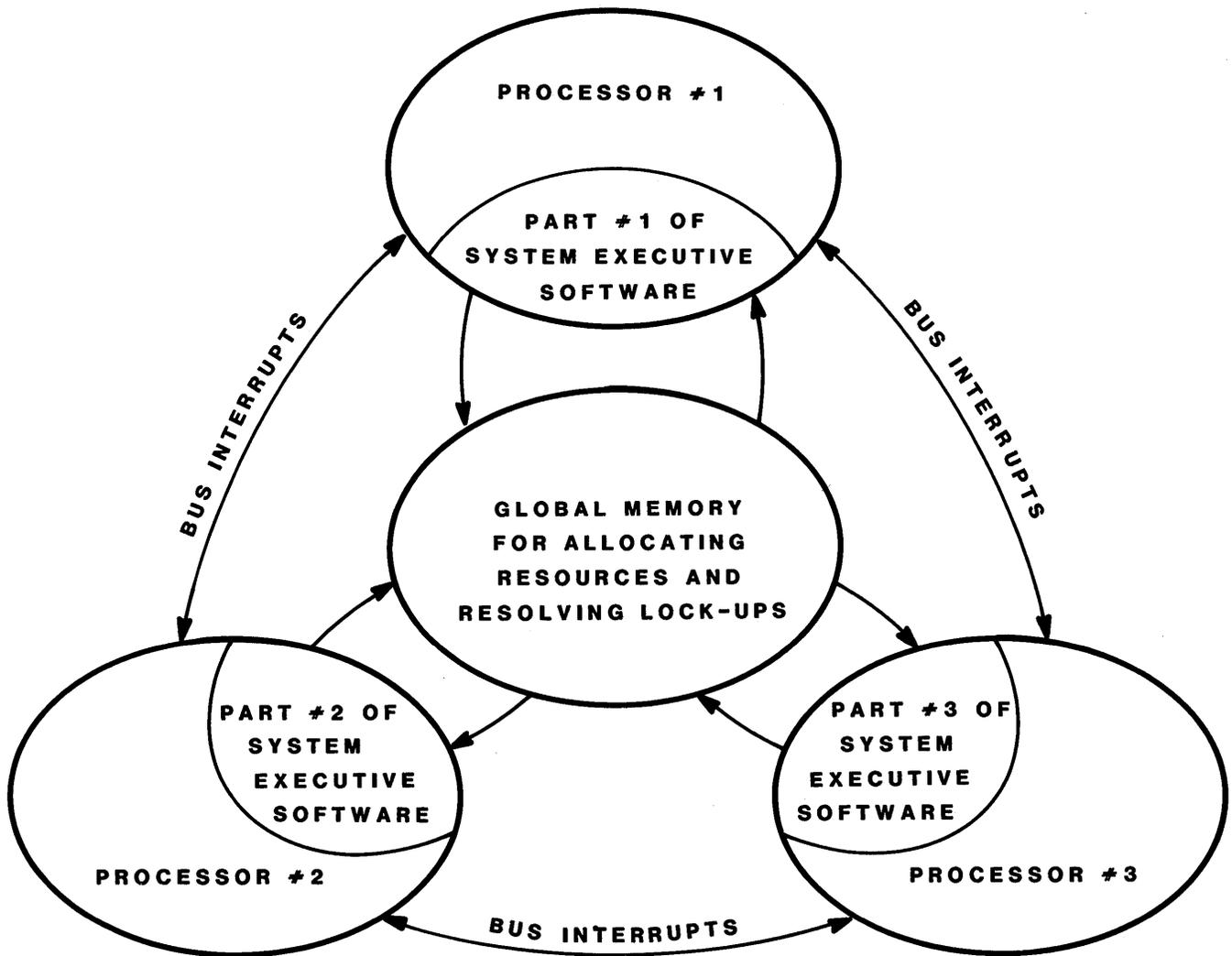
FIGURE 4-2. Interrupt Subsystem Structure: Distributed System
