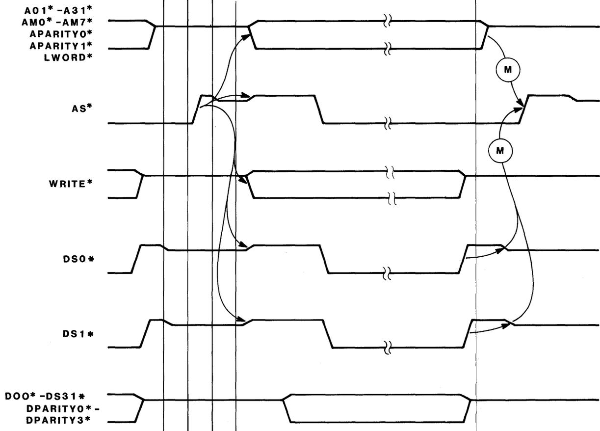
FIGURE 2-10. Data Transfer Bus MASTER Exchange Sequence
