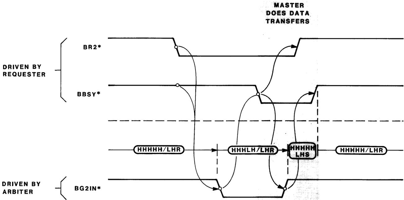
FIGURE 3-20. Sequence Diagram: Arbitration
