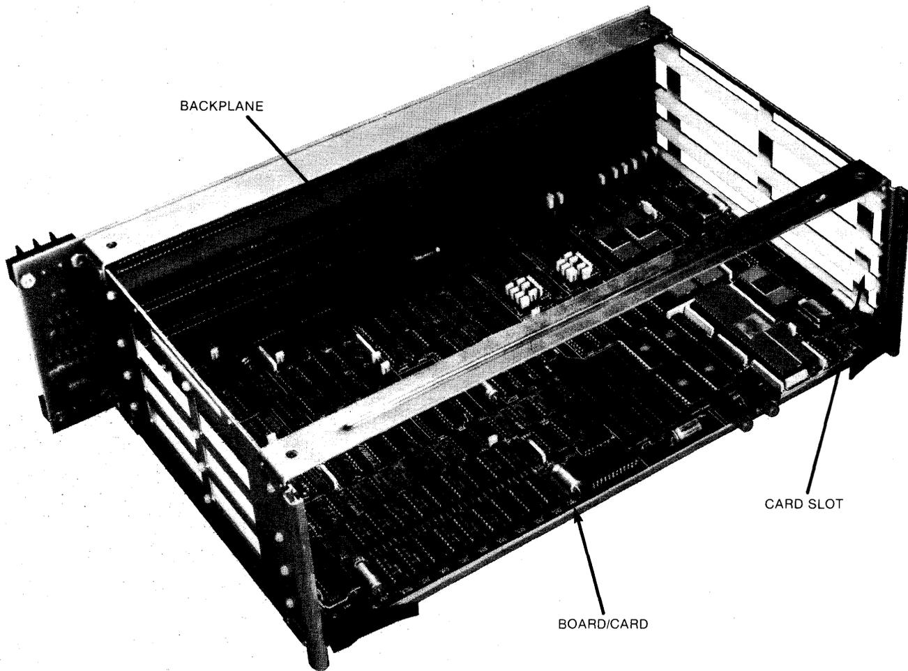
FIGURE 1-1. Typical Multi-Slot System Card Cage with Backplane
