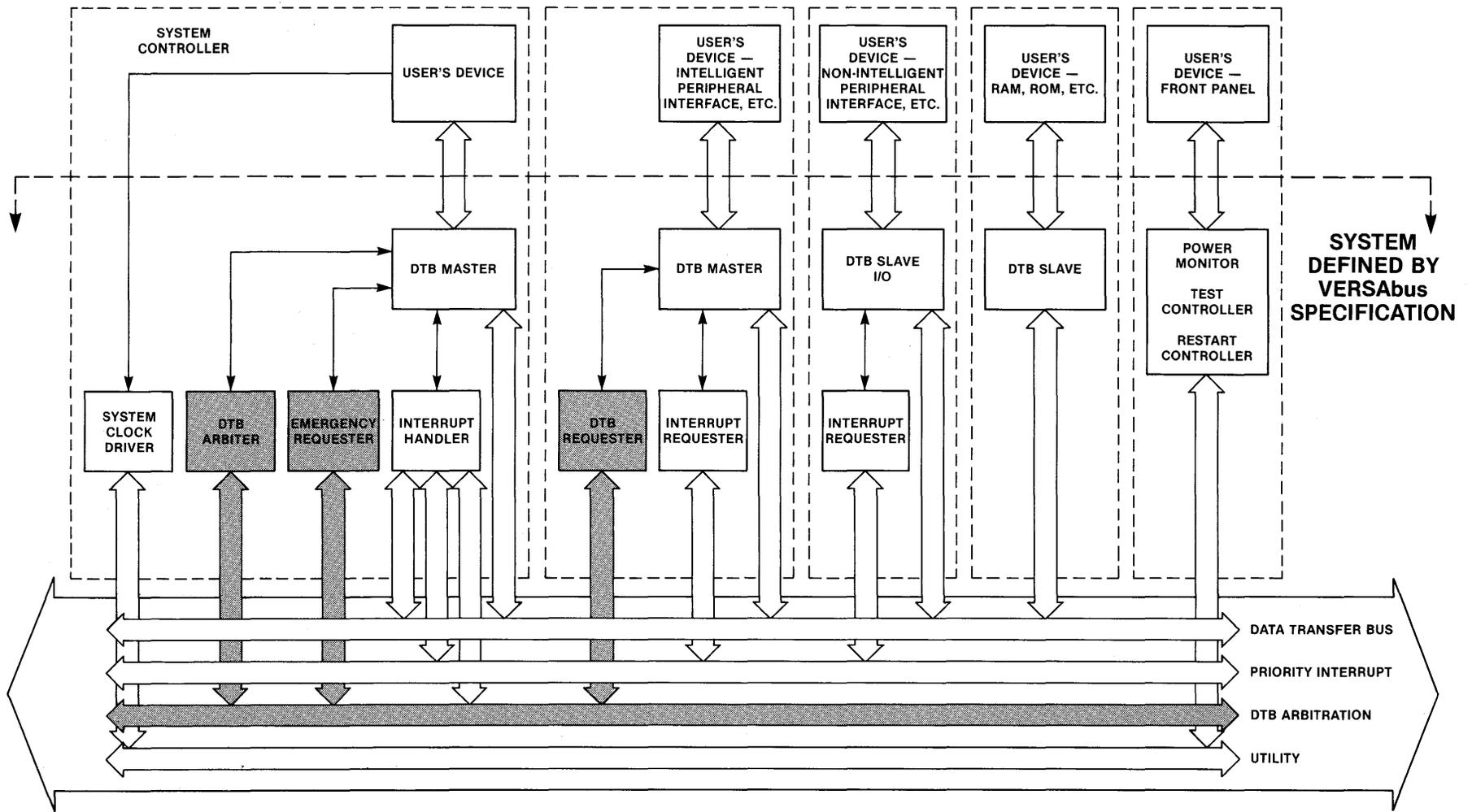
FIGURE 3-1. VERSAbus Arbitration Functional Block Diagram
