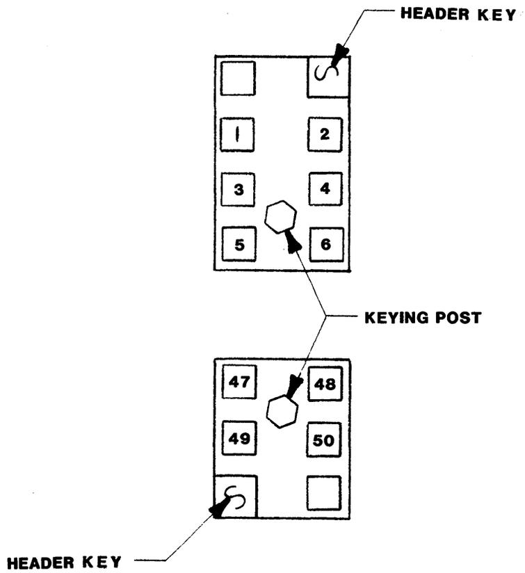
FIGURE 8-7. AMP Two-Piece Keying Header
