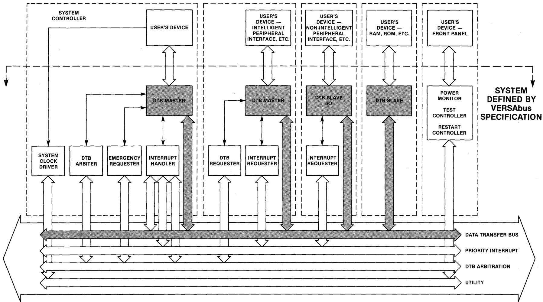
FIGURE 2-1. VERSAbus Data Transfer Functional Block Diagram
