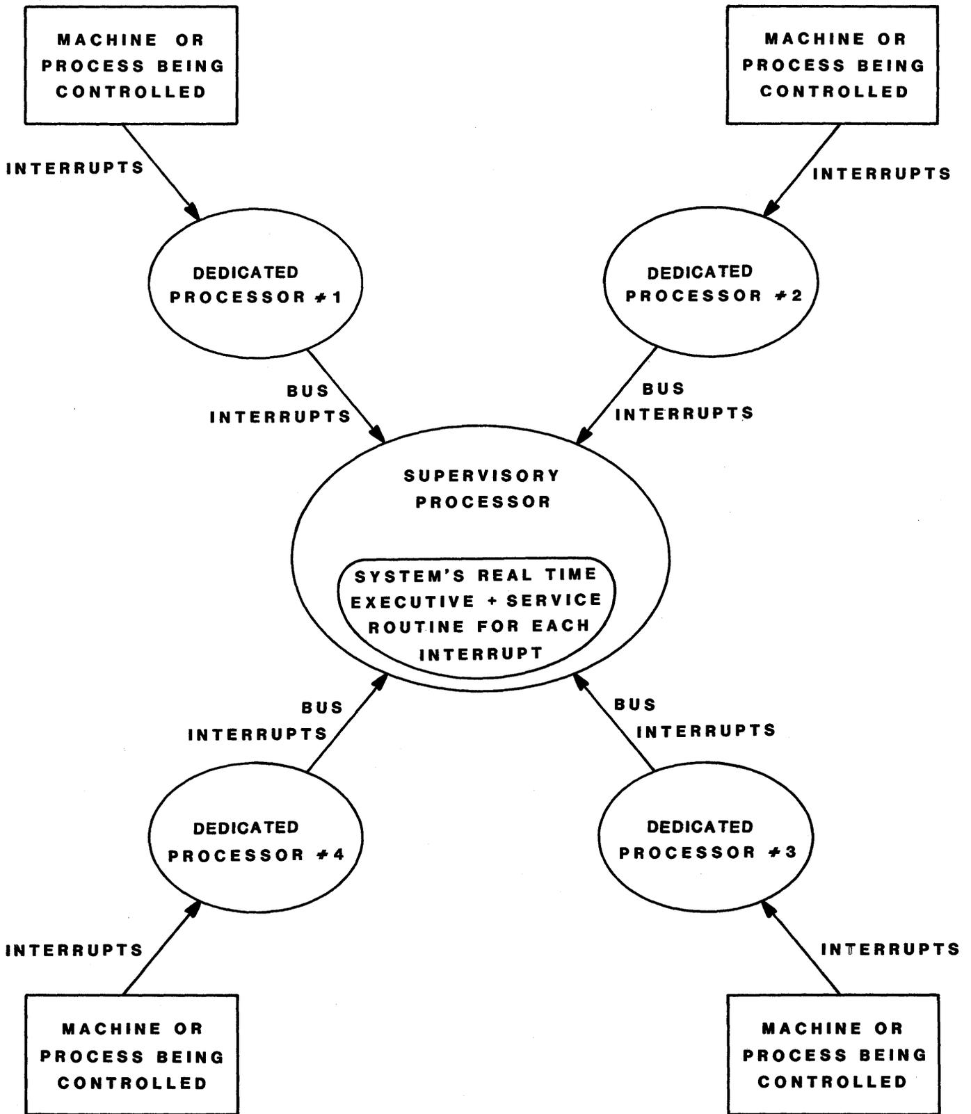
FIGURE 4-1. Interrupt Subsystem Structure: Single Handler System
