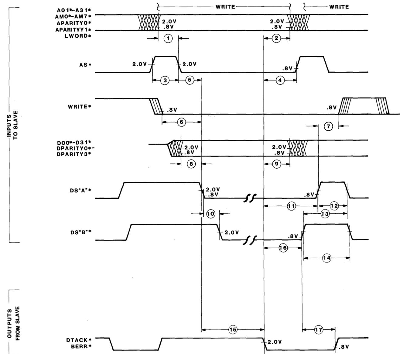
FIGURE 2-17. Data Transfer Bus SLAVE Write Cycle
