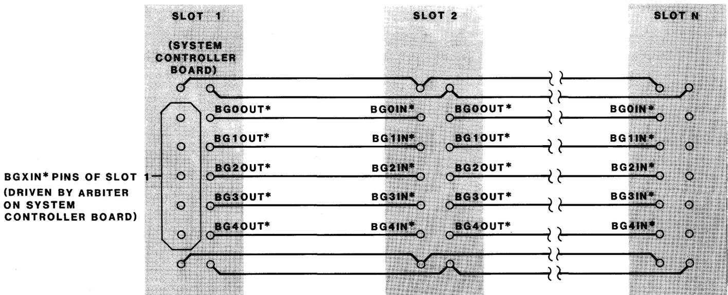
FIGURE 3-2. Illustration of the Daisy Chained Bus Grant Lines
