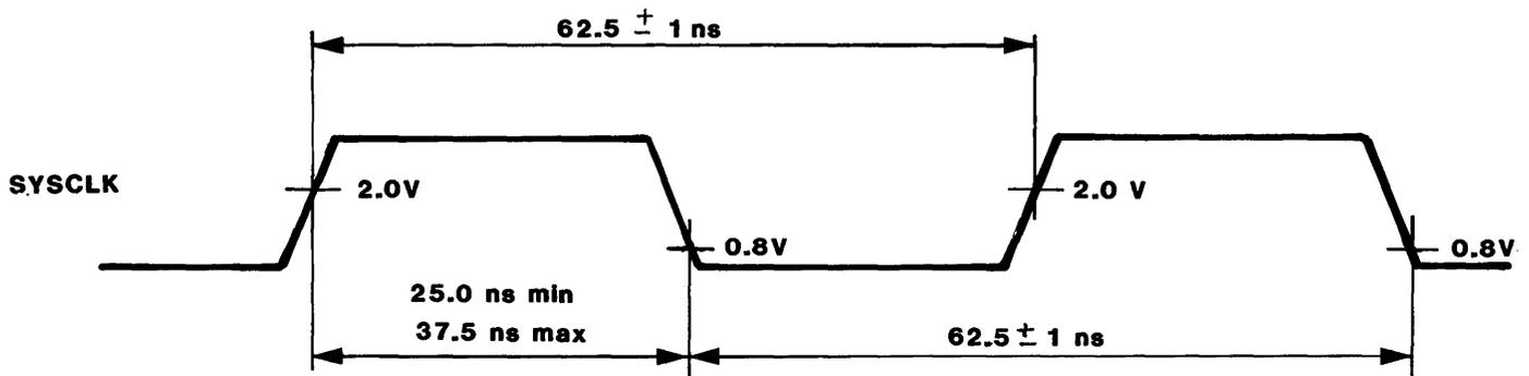
FIGURE 5-2. System Clock Timing Diagram
