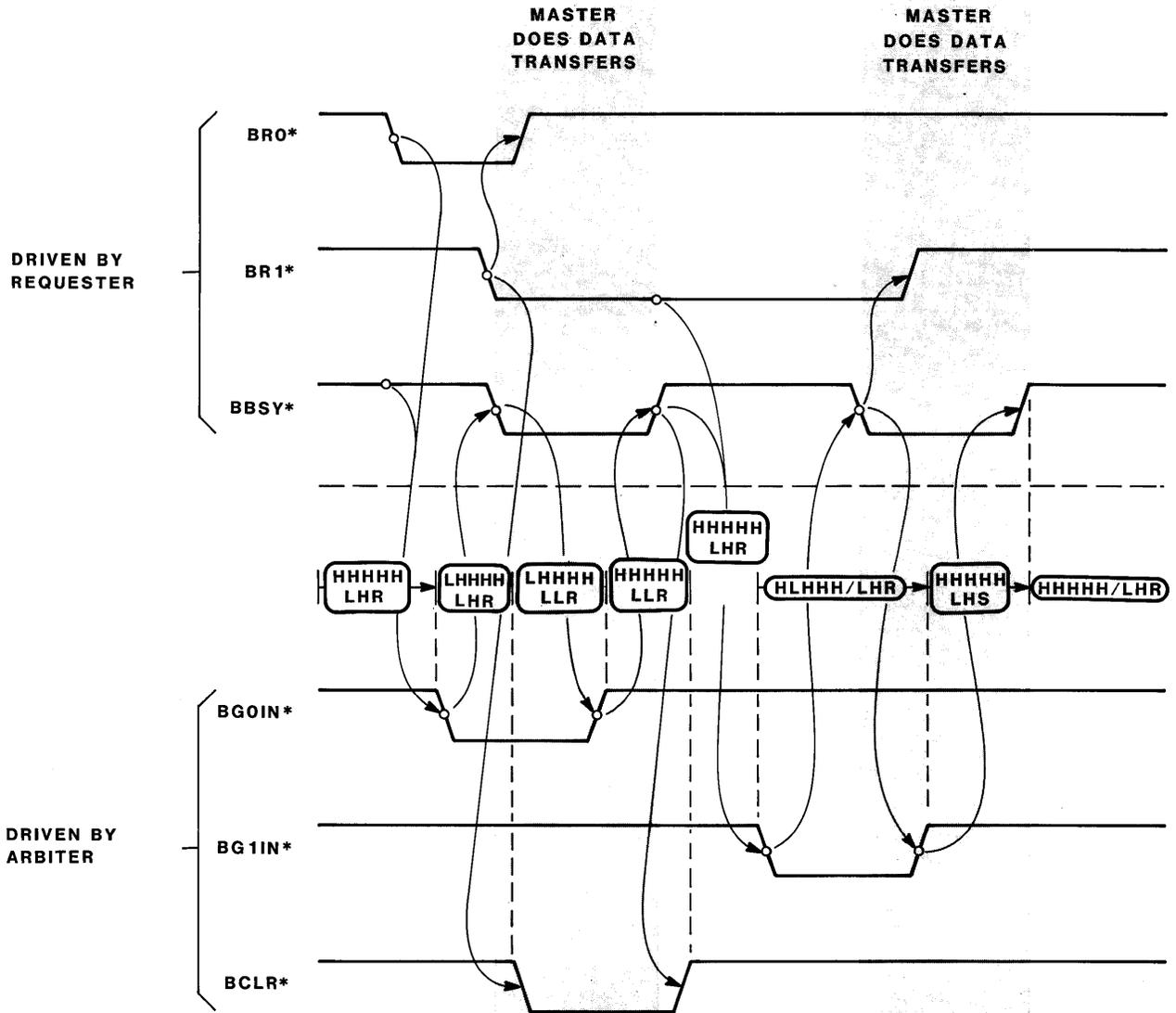
FIGURE 3-21. Sequence Diagram: Clearing the DTB Upon a Higher Priority Request
