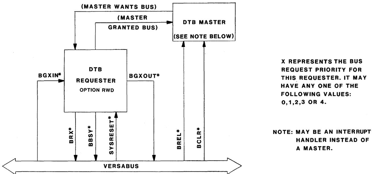
FIGURE 3-5. Block Diagram: Option RWD REQUESTER
