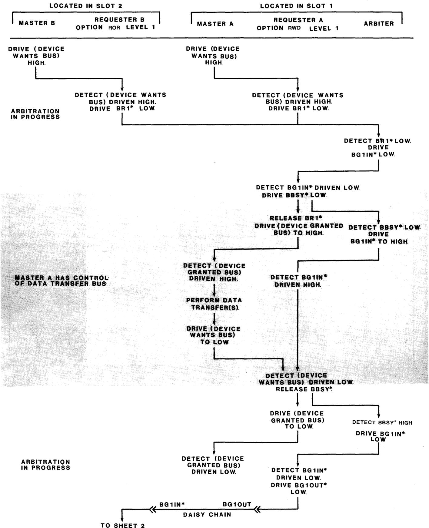
FIGURE 3-9. Arbitration Flow Diagram - Two REQUESTERS/Same Request Level (Sheet 1 of 2)
