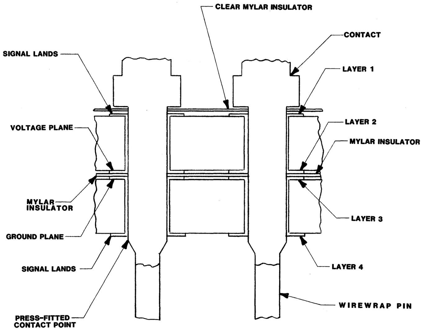
FIGURE 8-2. Typical Multilayer Backplane/PCB Cross-Sectional Area View
