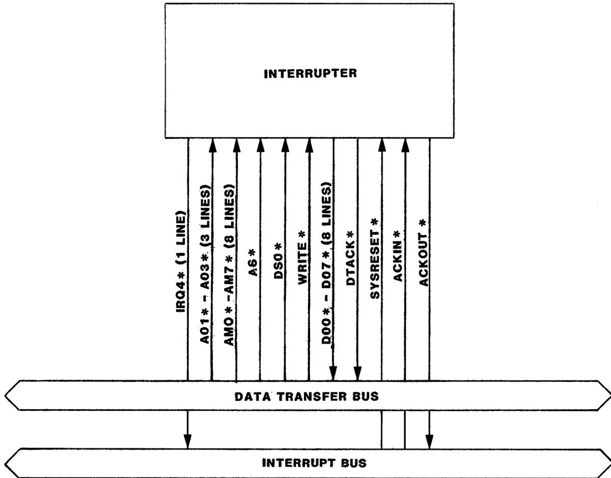
FIGURE 4-5. Signal Lines Used by an I(4) INTERRUPTER
