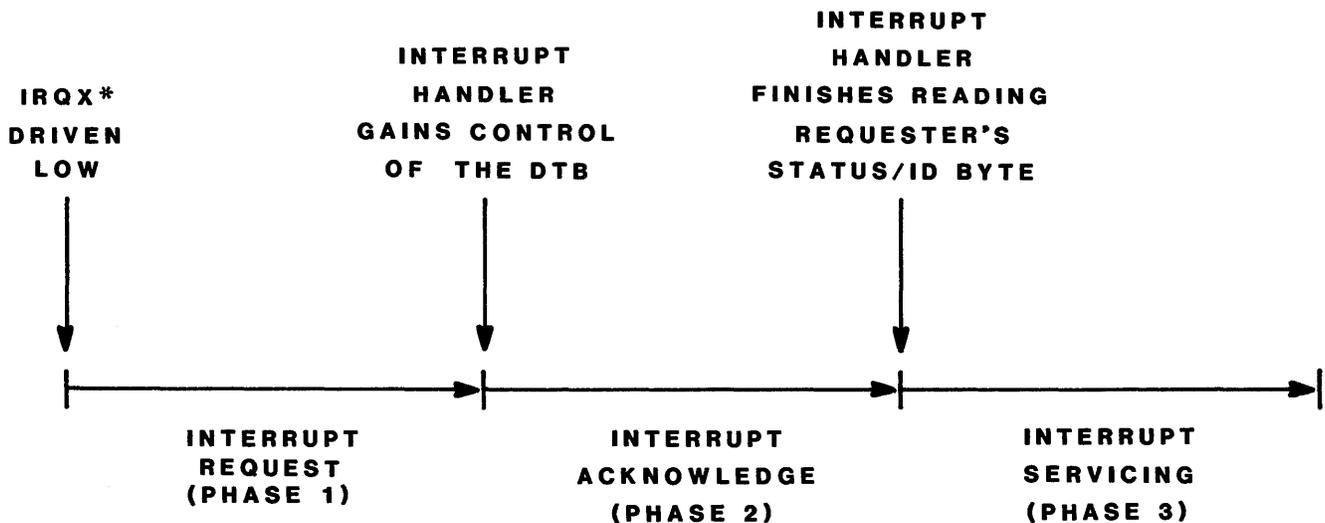
FIGURE 4-6. The Three Phases of an Interrupt Sequence
