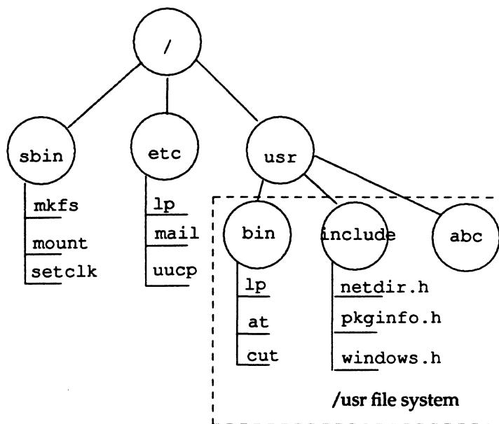
A directory such as `/usr` that is used to form the connection between the root file system and another mountable file system is sometimes called a "leaf" or "mount point." Regardless of the term used, such a directory is the root of the file system that descends from it. The name of that file system is the name of the directory. In our example the name of the file system is `/usr`.
