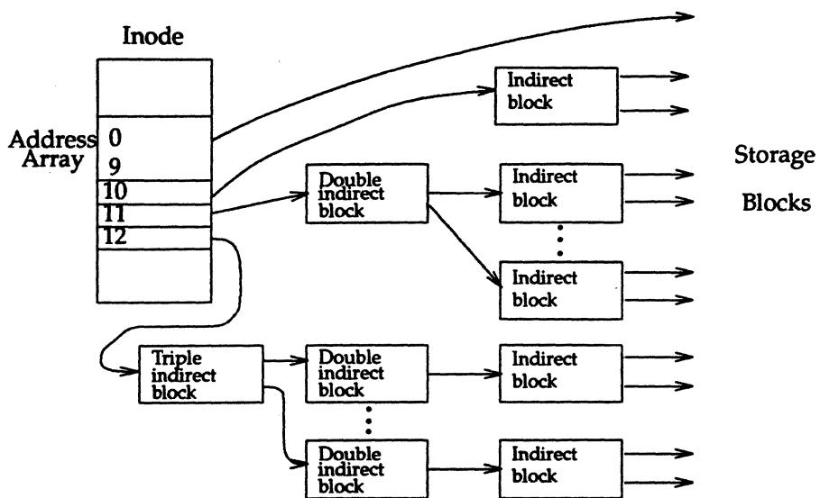
The following table shows the number of bytes addressable by the different levels of indirection in the inode address array for s5 file systems. These numbers are calculated using the logical block size of the file system and the number of bytes (four) used to hold an address.
