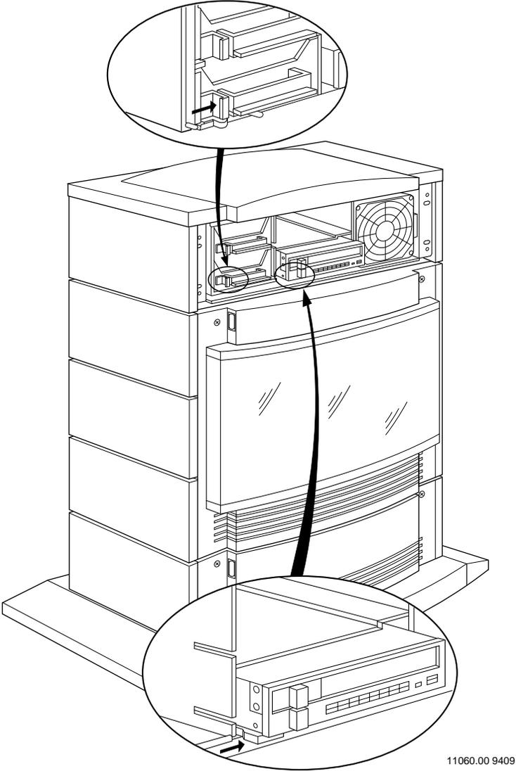
**Figure 4-4. Drive Module Release Latches**
