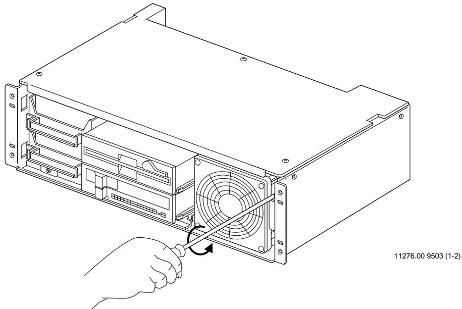
**Figure 4-3. Power Supply Removal**
