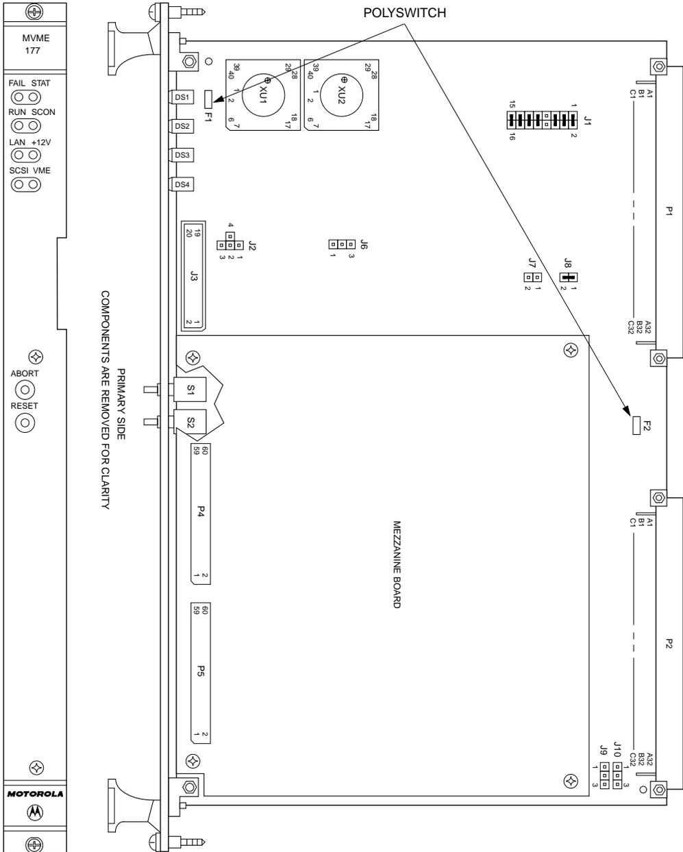
Figure 2-1. MVME177 Switches, Headers, Connectors, Polyswitches, and LEDs
