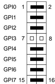
The MVME177 may be configured with these readable jumpers. These jumpers can be read as a register (at \$FFF40088) in the VMEchip2 LCSR. The bit values are read as a one when the jumper is off, and as a zero when the jumper is on. This jumper block (header J1) contains eight bits. Refer to the *Single Board Computers Programmer's Reference Guide*.
