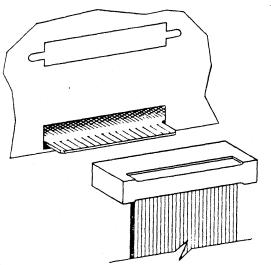
Figure D-2. Connecting the 34-pin plug
