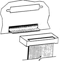
Figure 1-3: Connecting the 34-pin Plug
