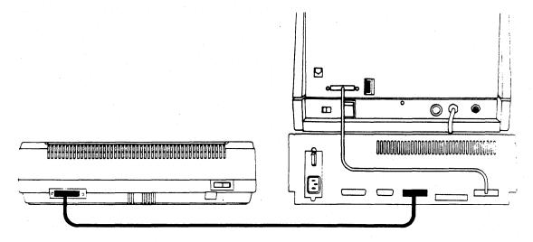
Figure 1-5: Serial Printer Connection (Mythical printer shown)
