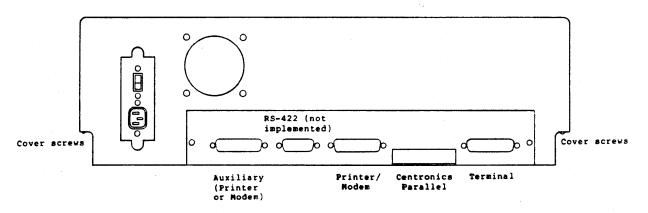
Figure D-1. MD-11 peripheral connectors
