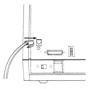
Figure 1-2: Connecting the MDT-60 Keyboard
