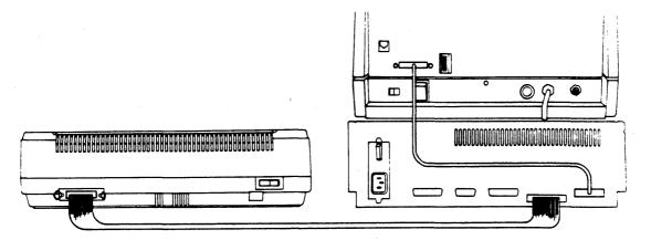
Figure 1-4: Connecting a Parallel Printer (MP-100 shown)
