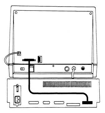
Figure 1-1: Terminal Cable Connection (MDT-60 Terminal shown)
