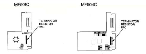
Fig. 1 Terminator and Jumper Plug Locations
