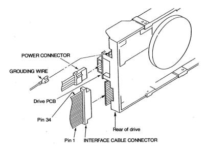
Fig. 2 Flexible Disk Drive Connector Locations
