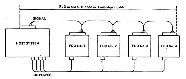
Figure 3-2 Cable connection (Schematic diagram)
