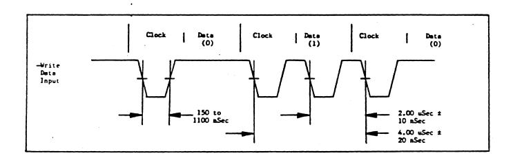
Figure 8-1 FM Write Timing
