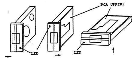
(Door open to left) (Door open to right) (Door open to upward)
