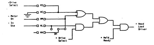
(Pull-up Resistors Amitted For Clarity)
