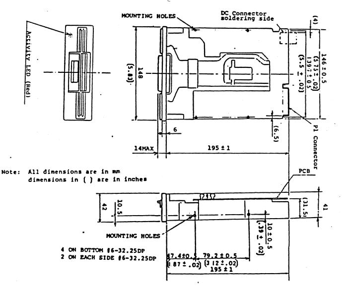
Figure 6-2 Dimensions of M4854-1S 6-2
