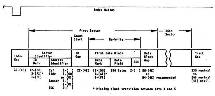
Figure 8-8 ISO-7487/2 Style, All Other Tracks (MFM) 250 or 300 Kbit/second Transfer Rate 8-6
