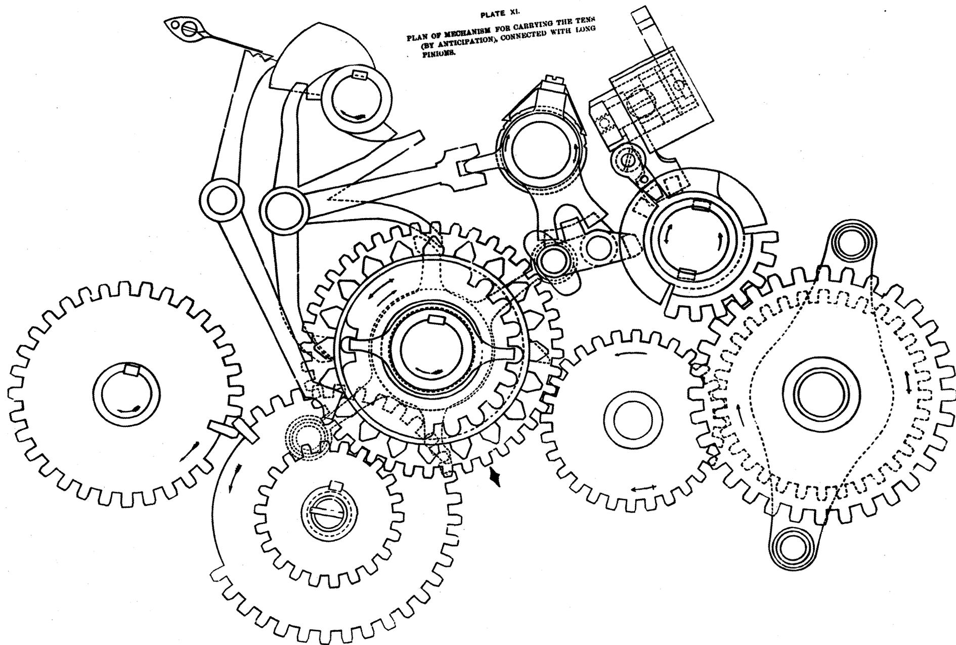
have been placed, the engine is special for that particular formula. The numerical value of its constants must then be put on the columns of wheels below them, and on setting the Engine in motion it will calculate and print the numerical results of that formula.
