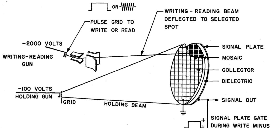
Fig. 6. Storage tube schematic
