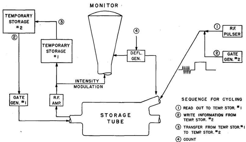
Fig. 13. Block diagram of dynamic tester
