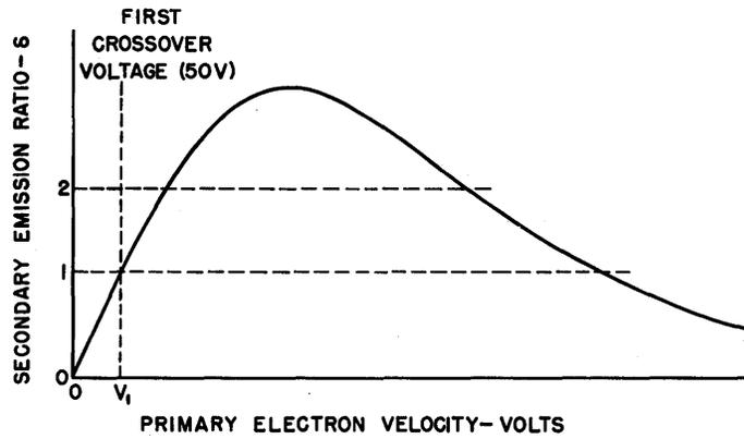
Fig. 9. Typical secondary emission curve
