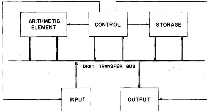
Fig. 6. Digital computer - simplified block diagram
