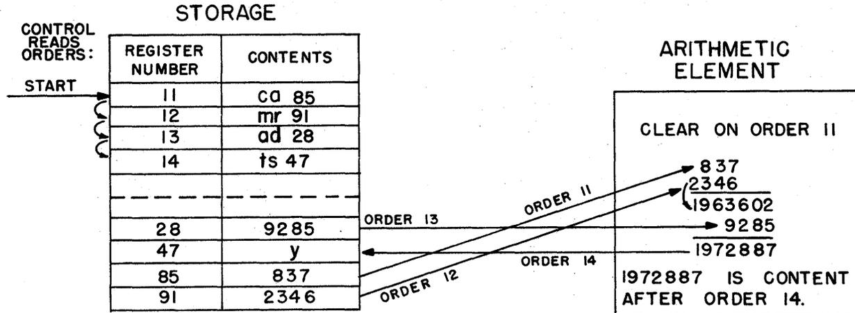
Fig. 13. Computer operations - specific example
