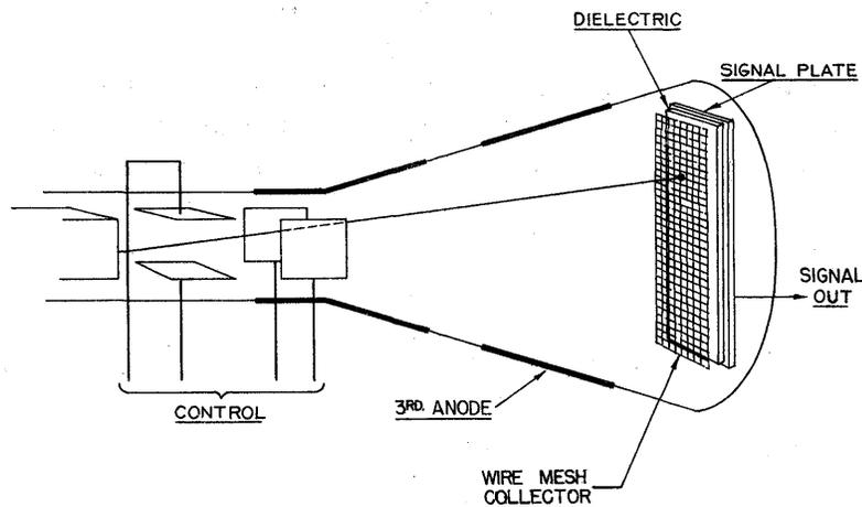
Fig. 11. Electrostatic storage tube
