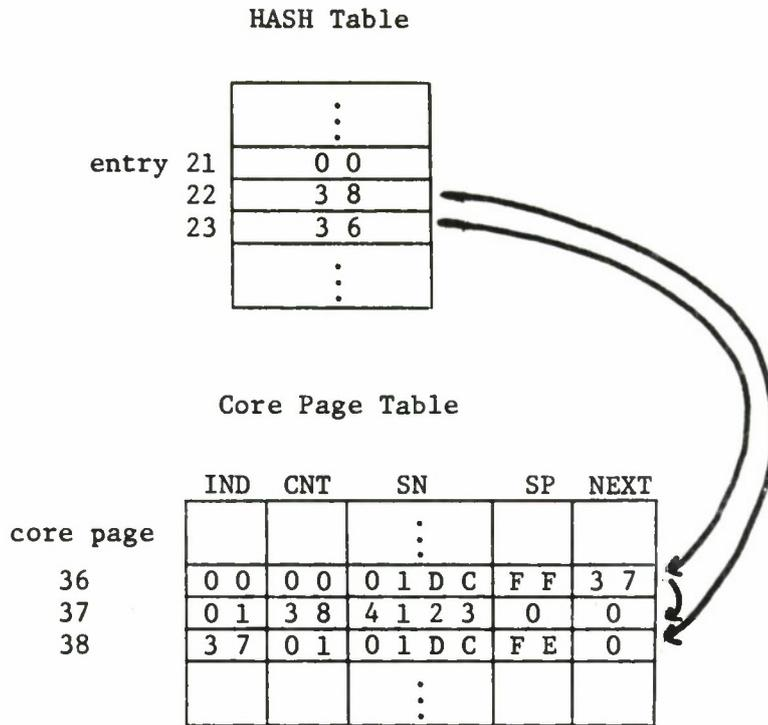
1. Three entries in HASH are shown.  $\text{HASH}_{21} = 0$ , which means no stream page located in core at the moment hashes into 21.  $\text{HASH}_{22}$  and  $\text{HASH}_{23}$  both contain the starts of hash chains. The chain coming from  $\text{HASH}_{22}$  is only one link long ( $\text{HASH}_{22} = 38$  and  $\text{NEXT}_{38} = 0$ ). The chain coming from  $\text{HASH}_{23}$  is two links long ( $\text{HASH}_{23} = 36$ ,  $\text{NEXT}_{36} = 37$ , and  $\text{NEXT}_{37} = 0$ ).
