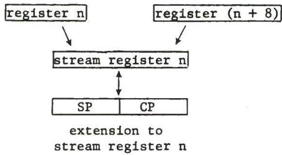
Figure 1. The Relationship between Registers, Stream Registers and Extensions
