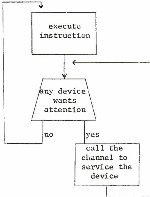
Figure 3. How the Channel Fits into the Microprogram
