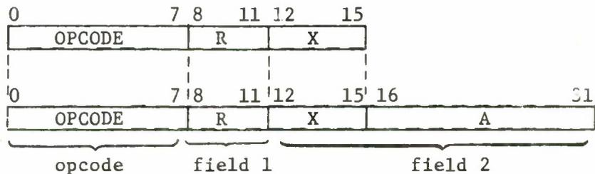
The opcode is 8 bits long. The first field, R, is 4 bits long and usually contains the number of a general register. The second field is either 4 bits long or 20 bits long. If it is 4 bits long, it contains the number, X, of a general register and the instruction is called a short instruction. A short instruction is written:
