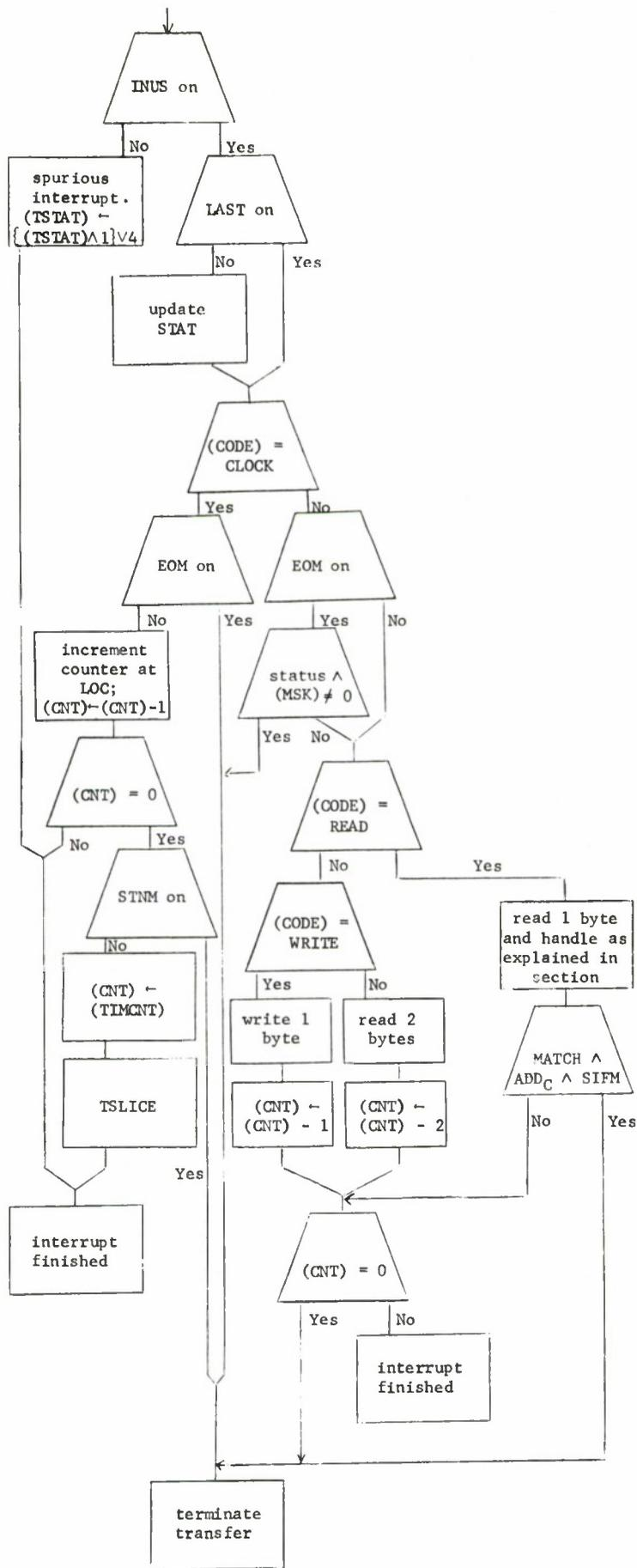
Figure 6. Channel Interrupt-Handling for a Device
