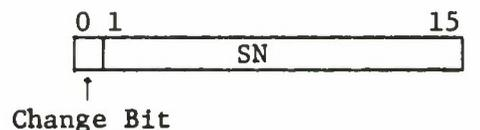
Bit 0 of this halfword is set by the microprogram whenever data is stored in the core page. SN is the name of the stream whose page occupies this core page.
