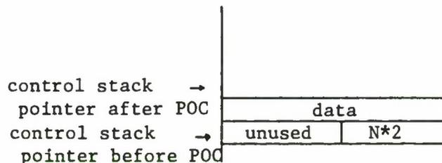
This data is fetched (from the next word in the control stack) and stored in the correct place. Recall that N is the address of a general register, stream register or (part of a) condition instruction. If N is the address of a stream register, then the effect of the POC instruction on N is precisely the same as if a "load stream name" instruction were being used to set the stream register at N. This means, if
