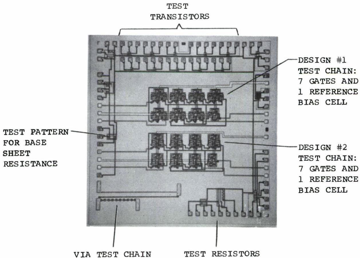
Figure 2. Photomicrograph of SMX14 Microcircuit Test Chip.
