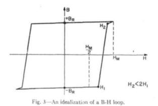
From the idealized hysteresis loop of Fig. 3, some necessary conditions for coincident-current operation
