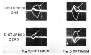
Fig. 6-Coincident-current test results, best ferritic core.
