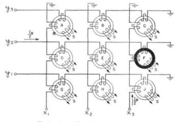
Fig. 2-A two-dimensional array of cores.
