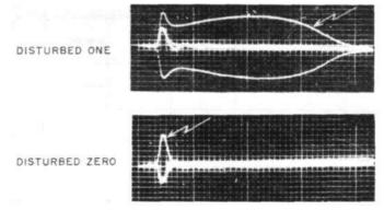
Fig. 5-Coincident-current test results, best metallic core.
