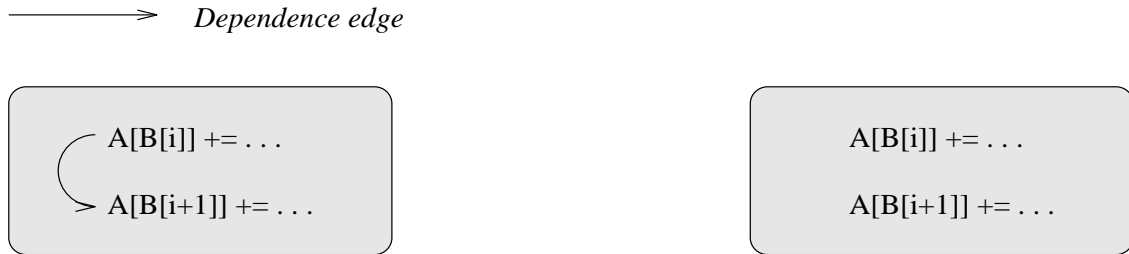
Figure 5.5: Example code benefiting from updates. (a) Initial code. Read/modify/write operations are performed on the two A[\dots] locations. The two stores to A[\dots] are potentially dependent and must be serialized. (b) Code after the update optimization. The two read/modify/write operations are moved into atomic message handlers for dynamic messages. Consequently, the two effectively have no dependence, since addition is associative and commutative. Hence the two read/modify/writes can be run as an independent epoch, as in described earlier in this section.
