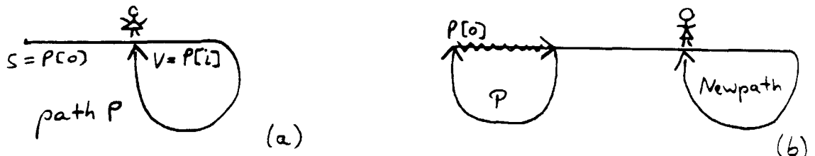
Figure 5-24: Partial Graph after the sink is found: (a) P is not a loop and SINK-CASE is called in line 9 of DEFICIENCY-ONE, (b) path P is a loop and work on P ends in sink v on path Newpath
